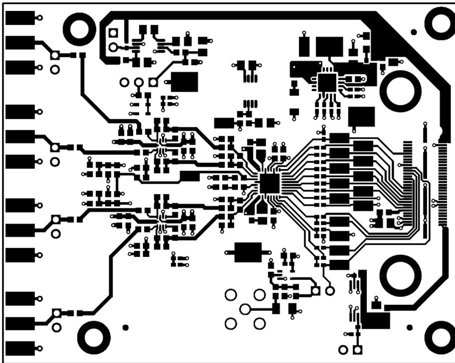
Figure 7-2. ADS9224REVM PCB Layer 1: Top Layer
