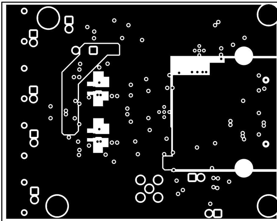
Figure 7-4. ADS9224REVM PCB Layer 3: Power Planes
