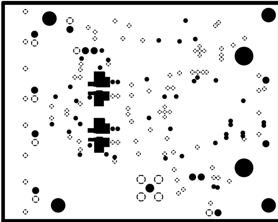
Figure 7-3. ADS9224REVM PCB Layer 2: GND Plane
