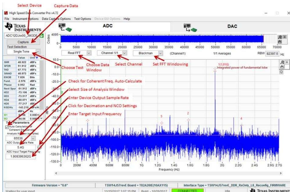
Figure 6. High Speed Data Converter Pro (HSDC) GUI
