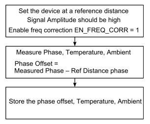
Figure 5. Phase Offset Calibration Procedure
