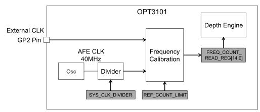
Figure 3. Frequency Calibration Block Diagram
