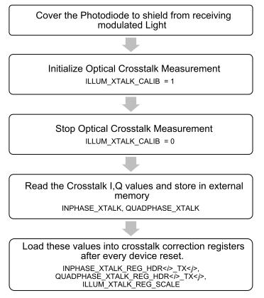
Figure 4. Illumination Crosstalk Calibration Procedure
