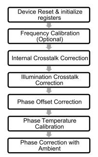
Figure 2. OPT3101 System Calibration Steps
