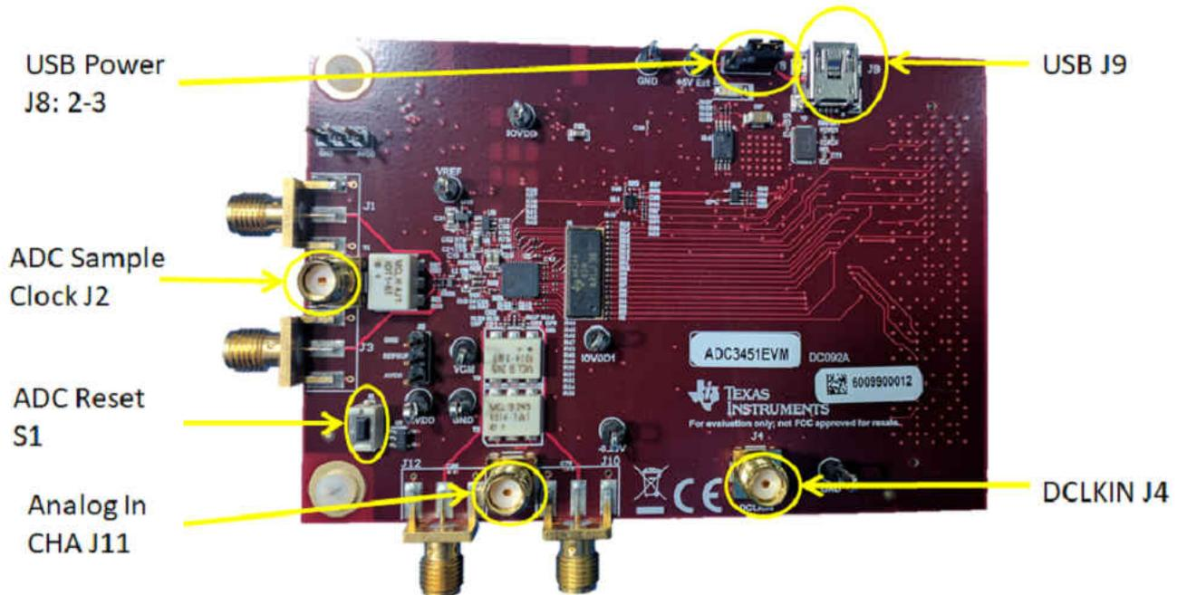
**Figure 2-1. ADC354xEVM Feature Identification**
