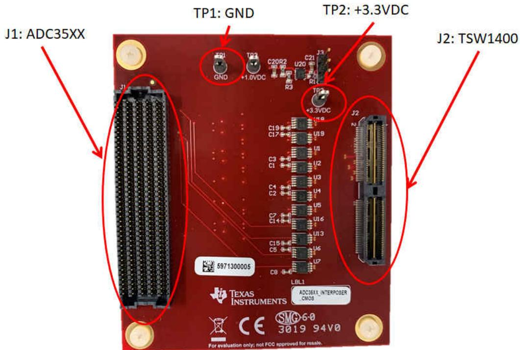
Figure 2-2. CMOS FPGA Interposer
