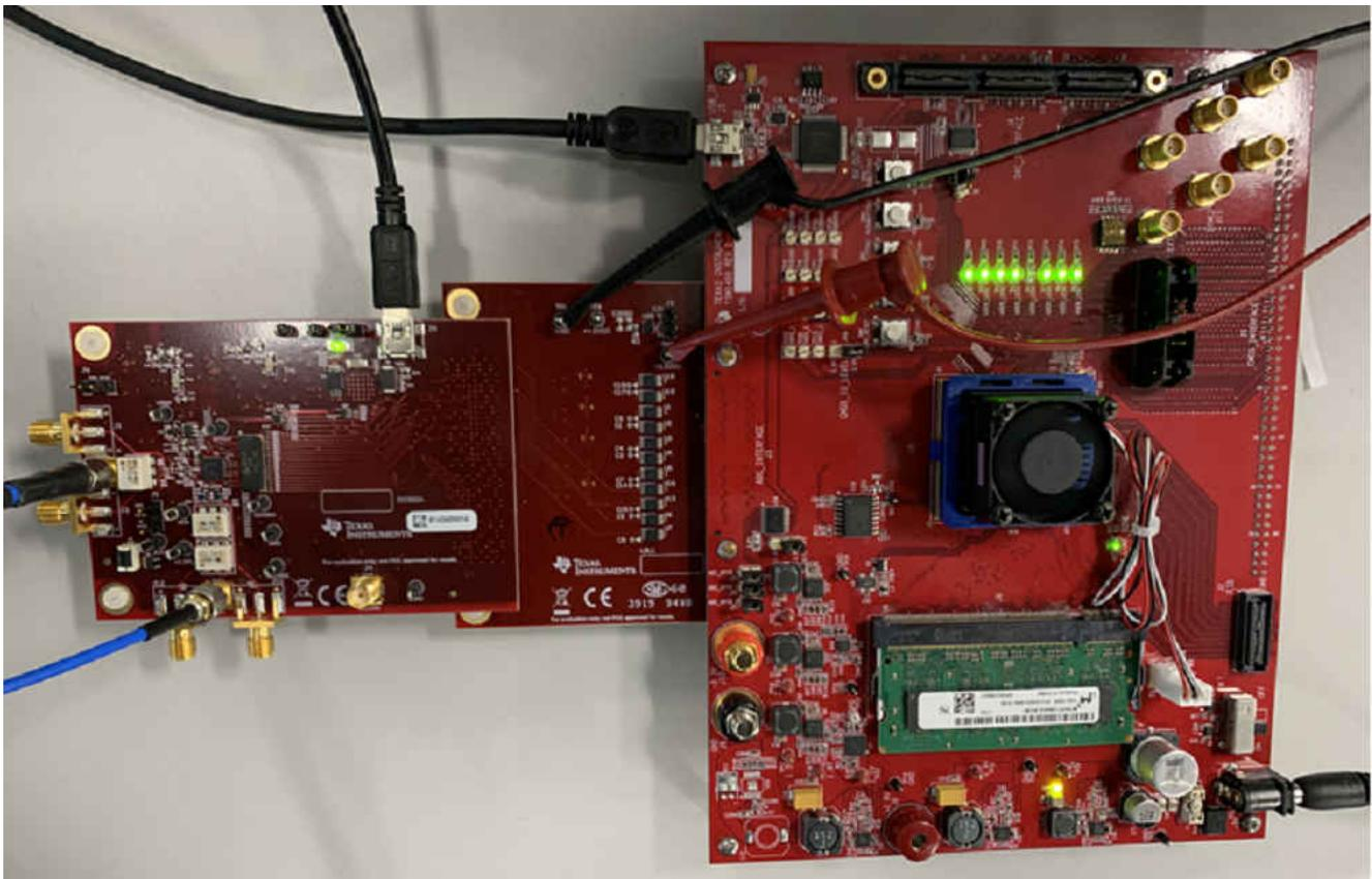
**Figure 3-1. ADC354xEVM Full Setup**
