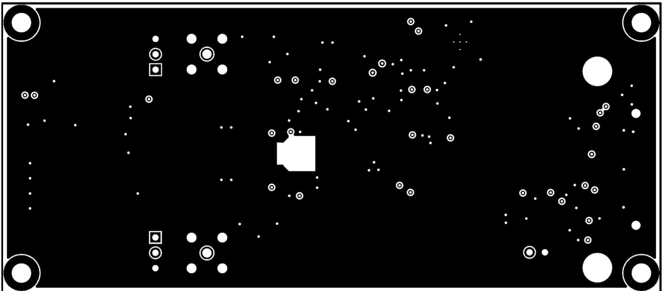
Figure 16. ADS8881EVMV2 PCB Layer 2: GND Plane
