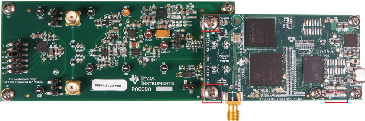
**Figure 7. EVM Hardware Setup and LED Indicators**
