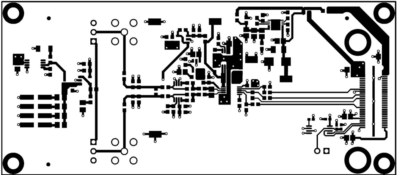
Figure 15. ADS8881EVMV2 PCB Layer 1: Top Layer
