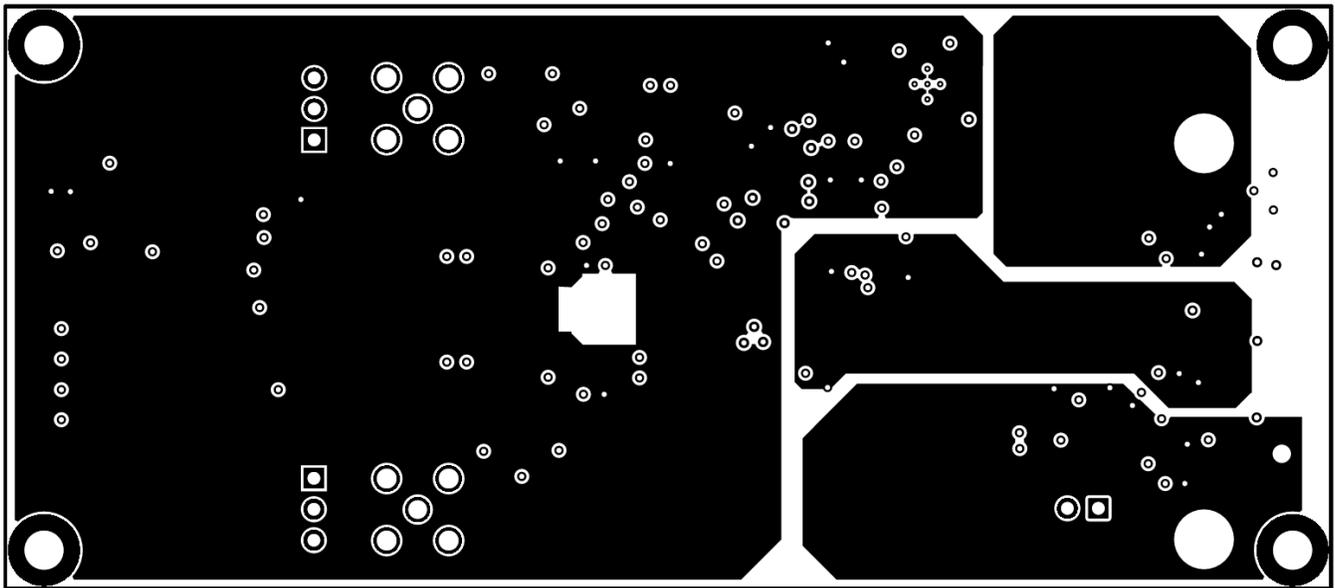
Figure 17. ADS8881EVMV2 PCB Layer 3: Power Planes
