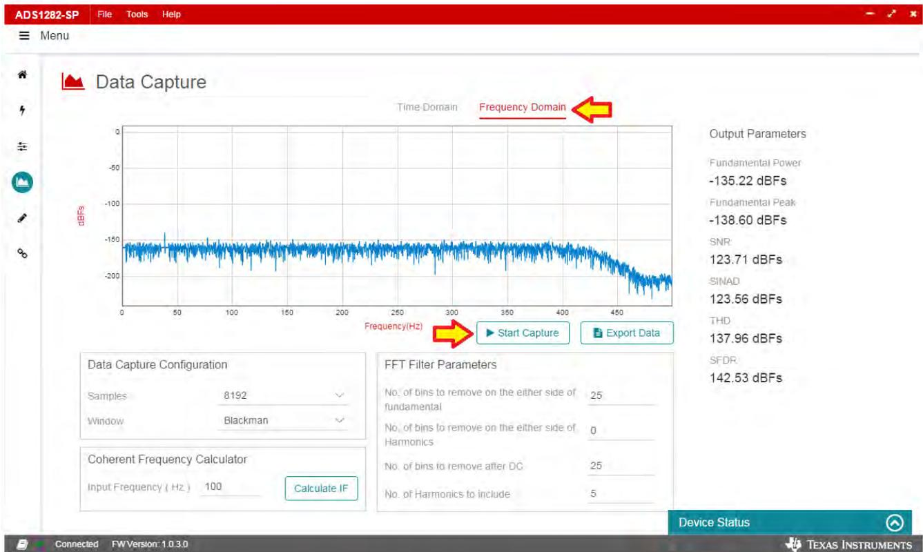
Figure 10. ADS1282-SP EVM GUI Data Capture Frequency Domain
