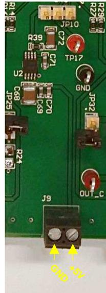
**Figure 5. Onboard Reference Supply Connections**
