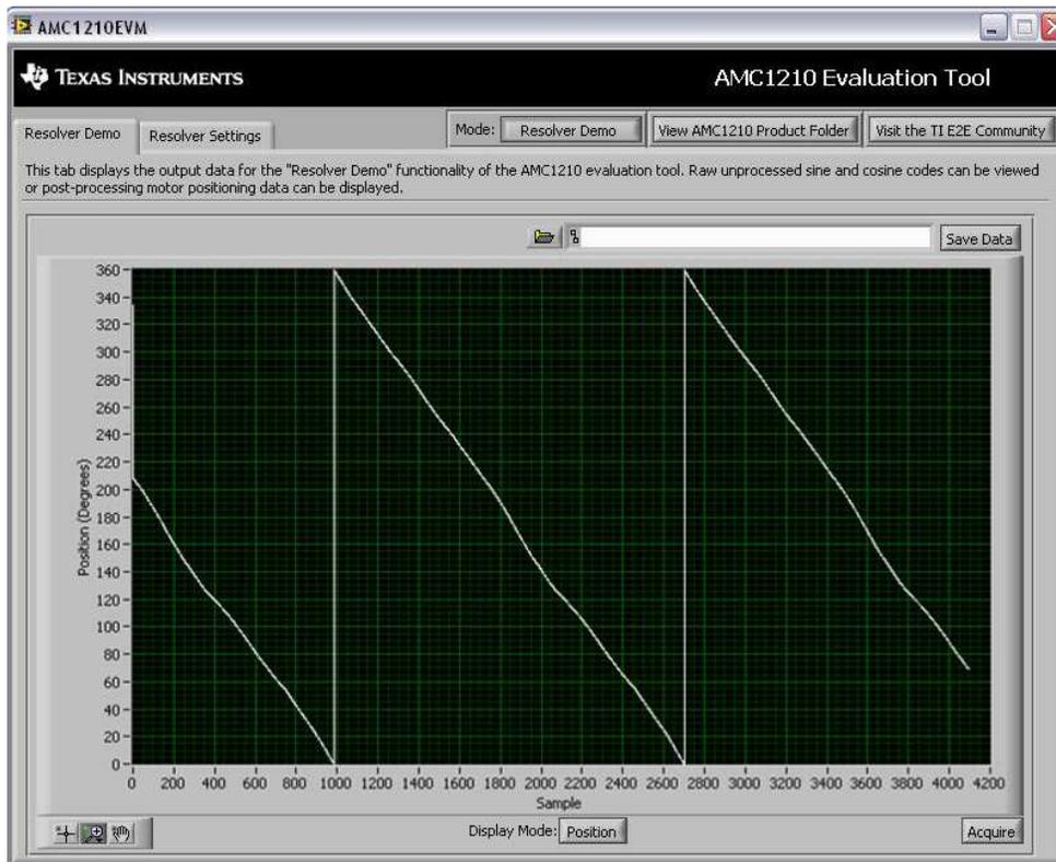
Figure 12. AMC1210MB-EVM Software Resolver Demo GUI: Position Data
