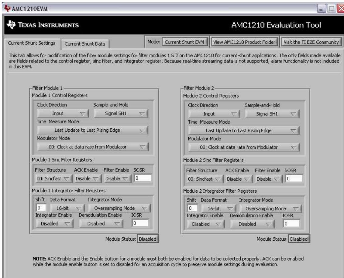
Figure 7. AMC1210MB-EVM Software Current Shunt Mode GUI
