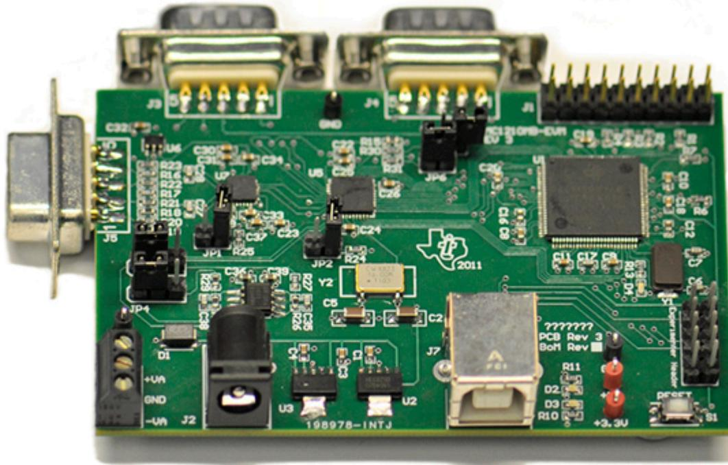
This user's guide describes the characteristics, operation, and use of the [AMC1210MB-EVM](#) as part of an evaluation system when used with Texas Instruments delta-sigma ( $\Delta\Sigma$ ) modulator evaluation modules (EVMs) in resolver or current-shunt applications. A schematic diagram and bill of materials are included in this document.
