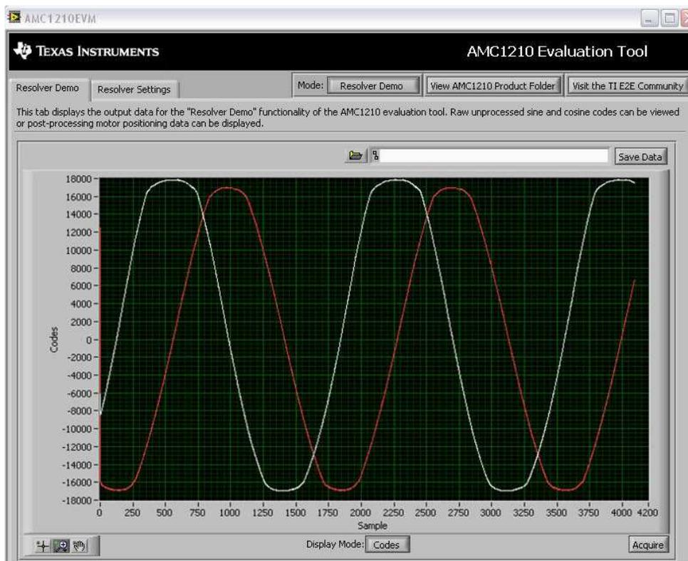
Figure 13. AMC1210MB-EVM Software Resolver Demo GUI: Raw Data
