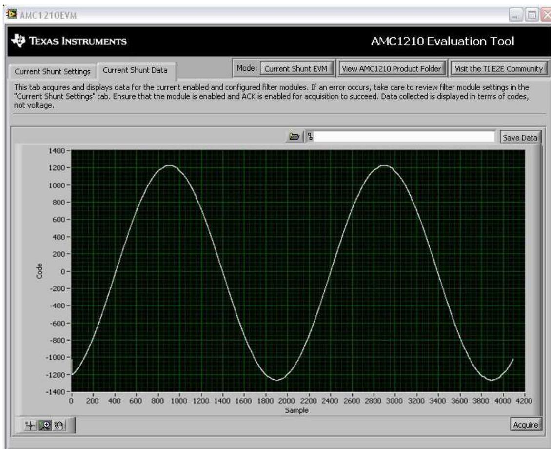
**Figure 10. AMC1210MB-EVM Software Current Shunt Data GUI**
