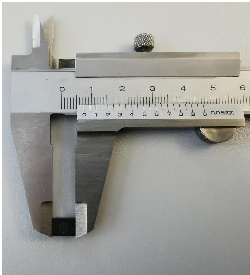
*Figure 2 Measuring of Clearance and Creepage*
