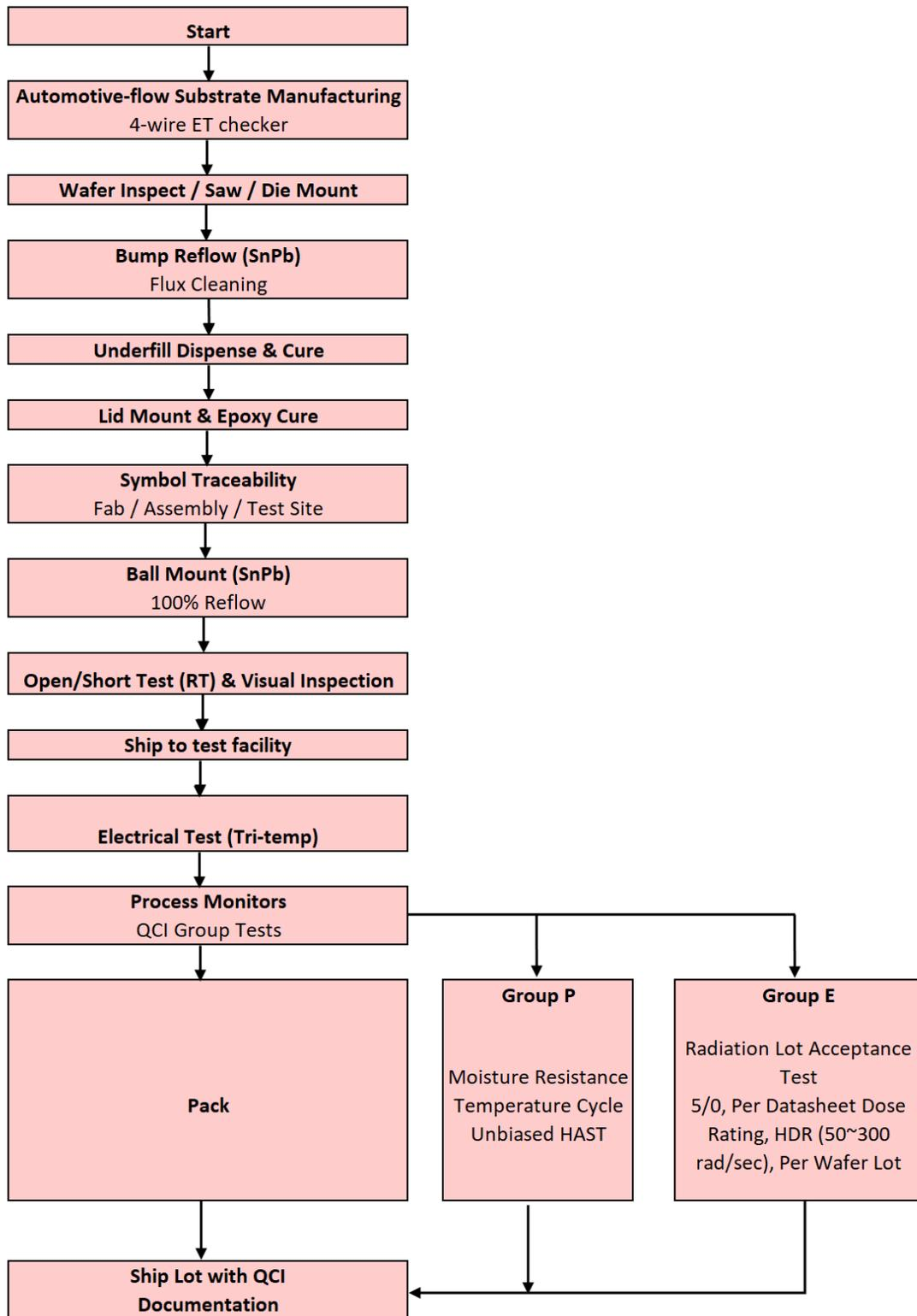
Figure 2-1. ADC12DJ5200-SEP Space-Enhanced Product Production Flow Chart
