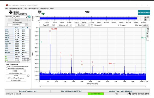
Figure 7-3. FFT Capture of Nominal Operating Conditions
