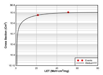
Figure 8-2. Cross Section for Short Events
