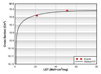
Figure 8-3. Cross Section for Long Events
