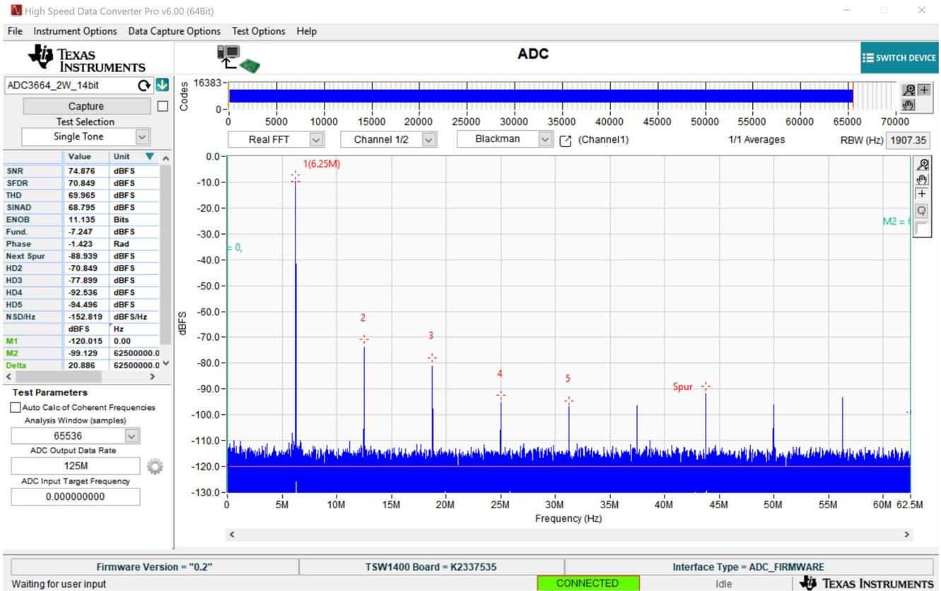
Figure 8-3. FFT Capture of Nominal Operating Conditions
