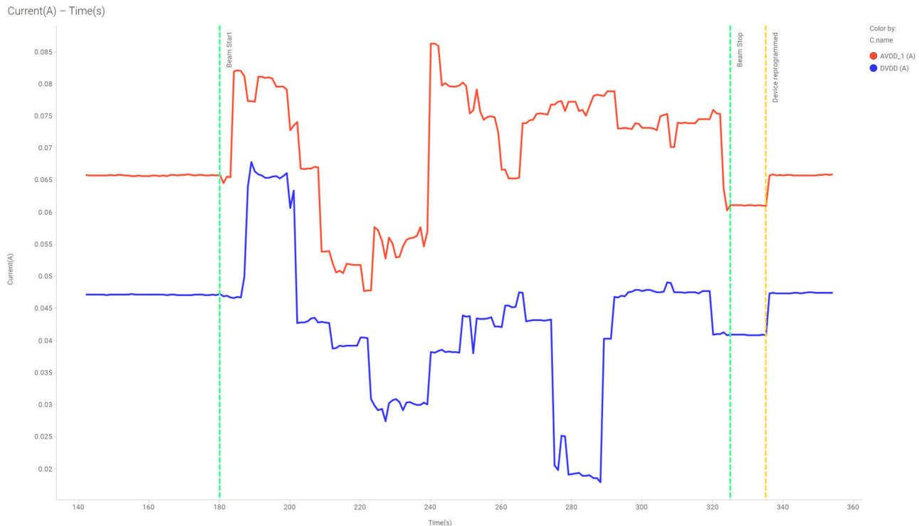
**Figure 7-1. Current Versus Time for ADC3683-SP at T = 125°C**
