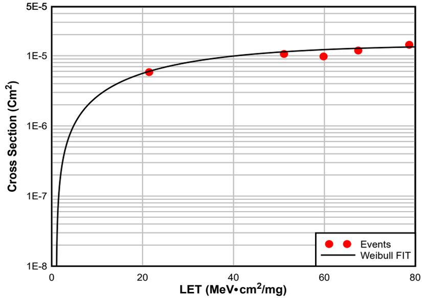
Figure 9-2. Cross Section for Short Events
