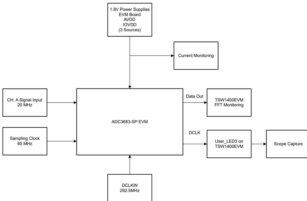
**Figure 6-1. Block Diagram of SEE Test Setup With the ADC3683-SP**
