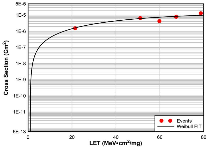
Figure 9-3. Cross Section for Long Events
