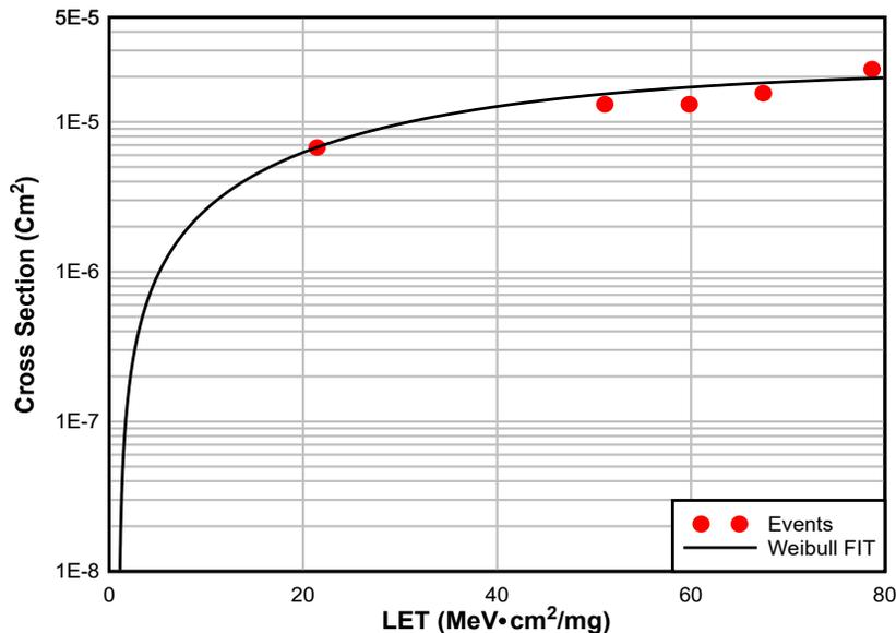
**Figure 9-1. Cross Section Plot for All Events**
