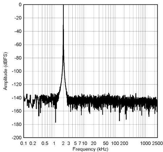
**Figure 2. FFT for  $f_{in} = 2\text{kHz}$**
