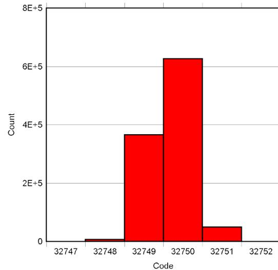
**Figure 3. Shorted-Input DC Offset Histogram**
