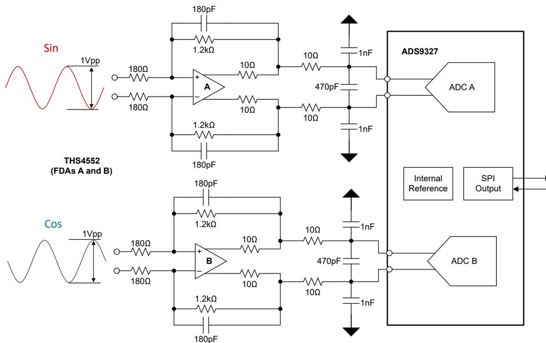
Figure 1. Circuit for Measuring  $1V_{PP}$  Sine and Cosine Signals
