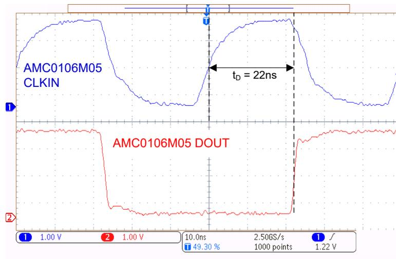
Figure 4-2. Digital Interface Timing
