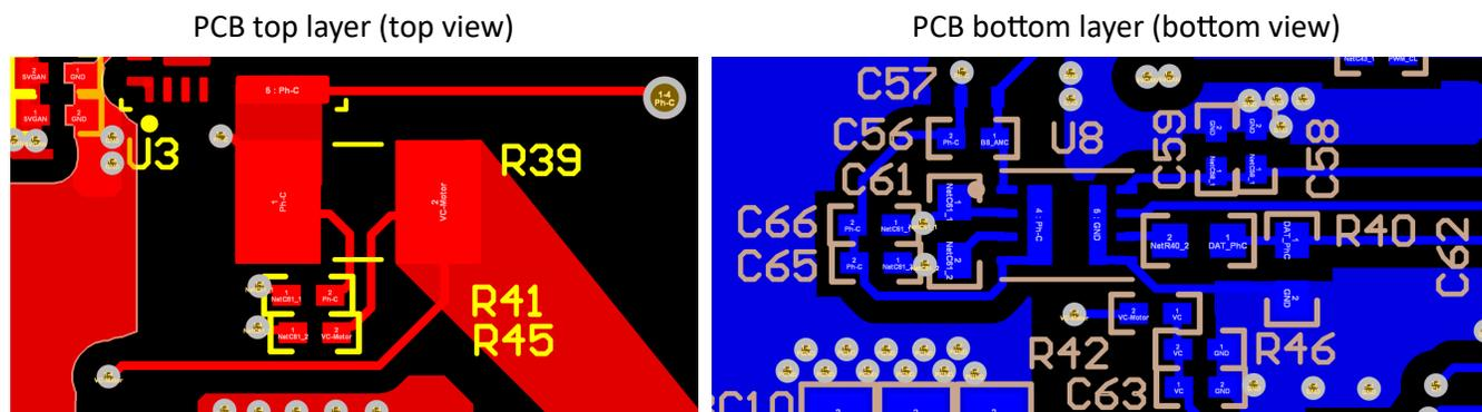
Figure 3-5. AMC0106M05 Top and Bottom Layer PCB Layout
