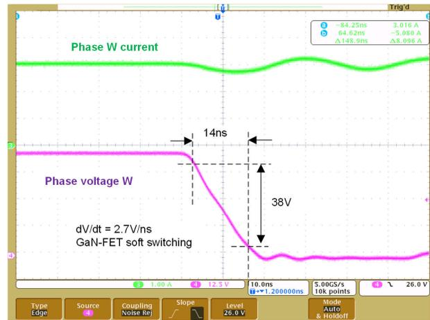
Figure 4-6. Phase W Voltage Falling Edge at 3A Current
