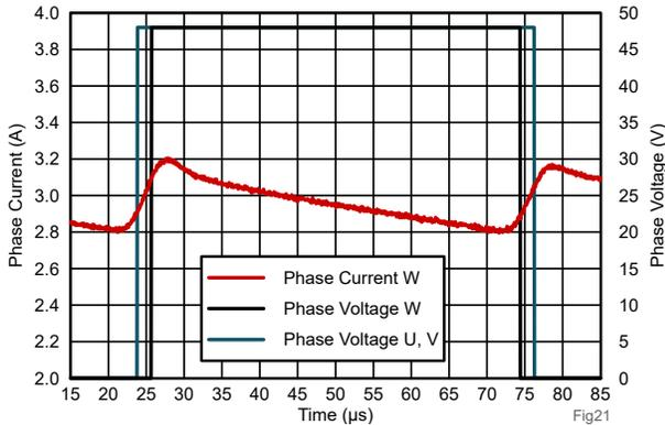
Figure 4-11. AMC0106M05 Phase Current  $I_W$  With OSR 64 at 3A Over one PWM Cycle
