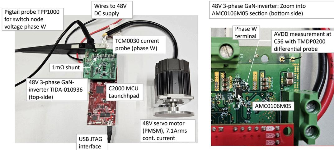
Figure 4-1. Picture of the Test Setup
