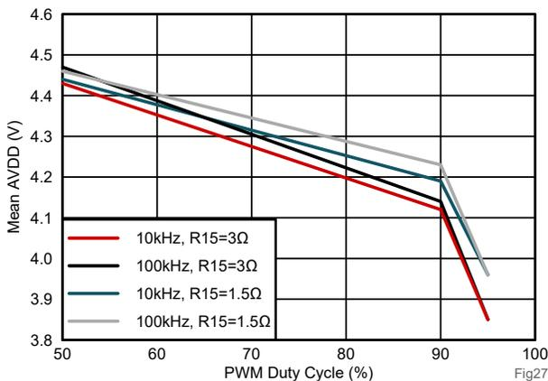
**Figure 4-17. Mean AVDD Bootstrap Voltage**
