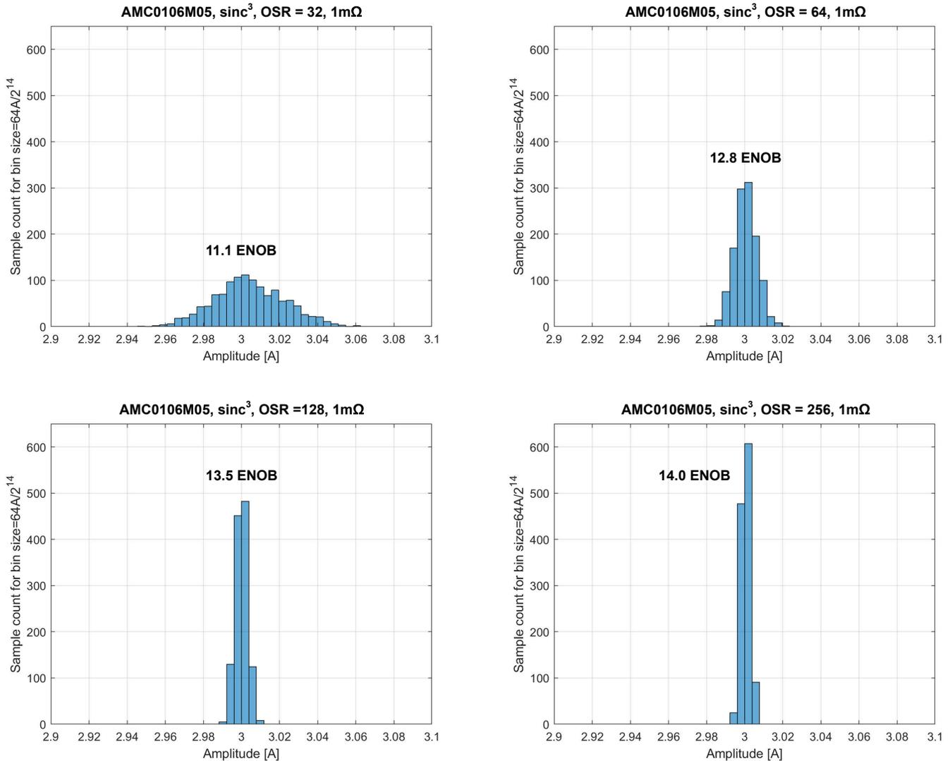
Figure 4-3. Phase Current Histograms for Different OSRs at 3A Phase Current
