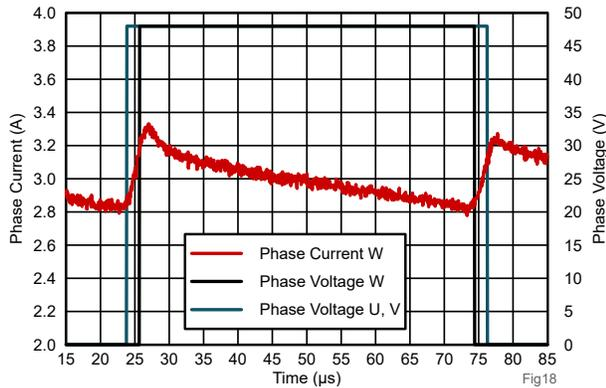
**Figure 4-8. AMC0106M05 Phase Current  $I_W$  with OSR=32 at 3A Over one PWM Cycle**
