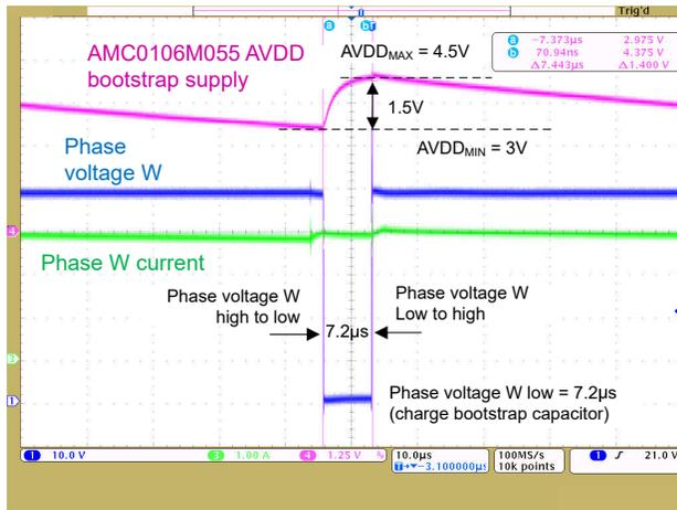
**Figure 4-20. Phase W Voltage at 10kHz PWM with 92.8% Duty Cycle, Phase Current W and AMC0106M05 AVDD**
