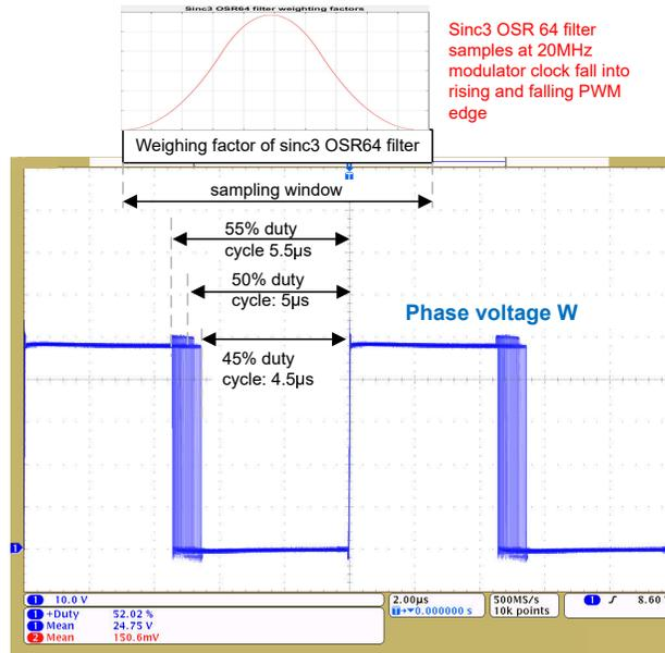
Figure 4-13. Scope Plot of Infinite Persistence Measurement of the Phase W Voltage
