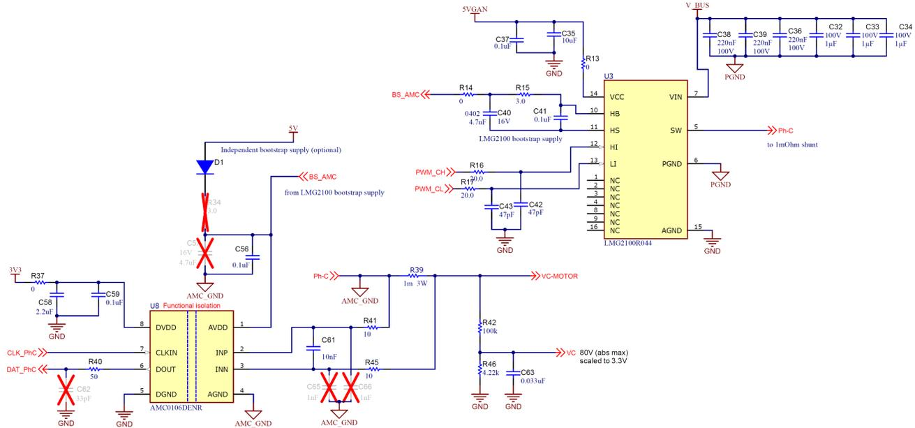
Figure 3-4. AMC0106M05 Schematic Using the LMG2100R44 Bootstrap Supply
