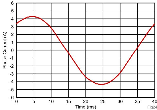
Figure 4-14. AMC0106M05 Phase Current  $I_w$  with OSR 64 at 100kHz PWM
