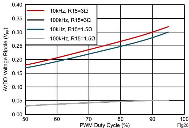
**Figure 4-18. AVDD Bootstrap Voltage Ripple**
