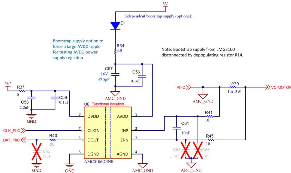
**Figure 4-19. AMC0106M06 AVDD Bootstrap Configuration for This Test**
