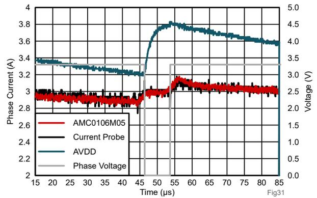
**Figure 4-21. AMC0106M05 Measurement with OSR 32 at 3A vs Current Probe During Large AVDD Ripple**
