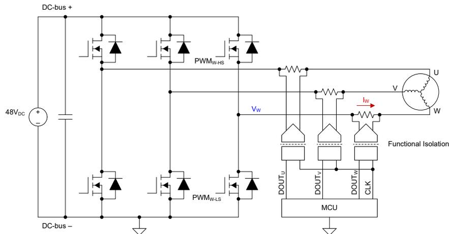
**Figure 1-1. 48V, 3-Phase Inverter With Shunt-Based, In-Phase Current Sensing**
