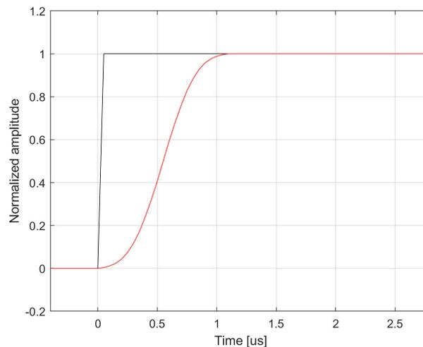
**Figure 3-8. Step Response of a Sinc<sup>3</sup> OSR 8 Filter**
