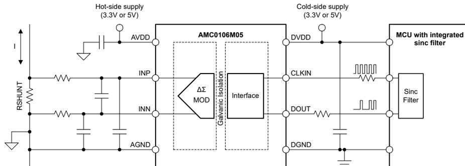
**Figure 3-1. Isolated Phase Current Sense Subsystem with MCU Integrated Sync Filter**
