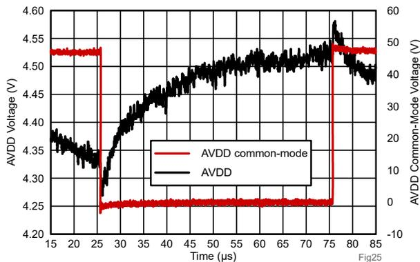
Figure 4-15. Bootstrap Voltage at 10kHz PWM, 50% Duty Cycle
