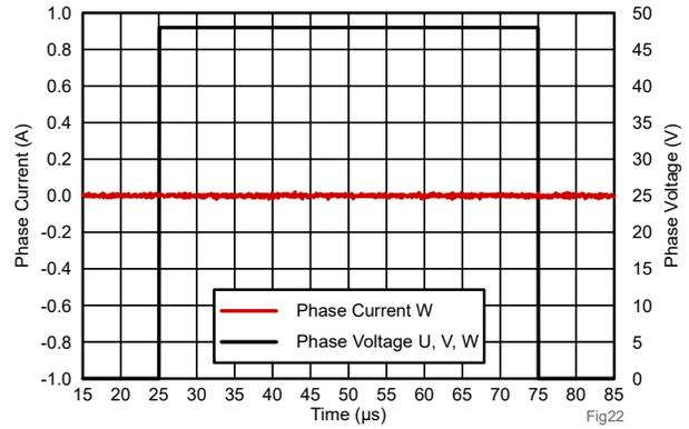
Figure 4-12. AMC0106M05 Phase Current  $I_W$  with OSR 64 at 0A Over one PWM Cycle
