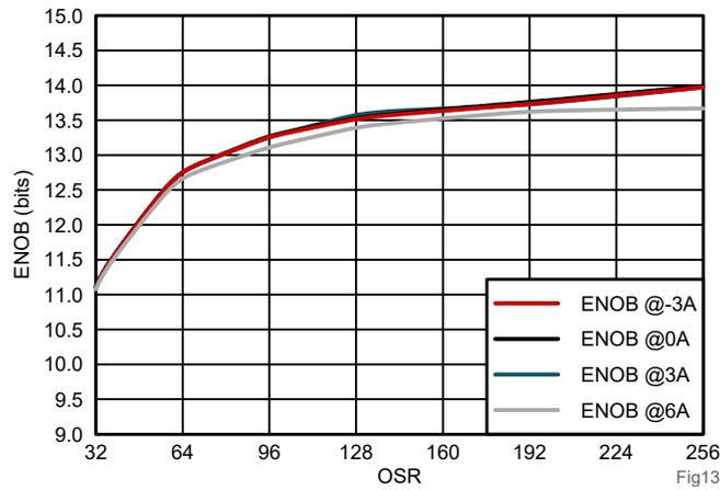
**Figure 4-4. Phase Current ENOB vs. OSR**
