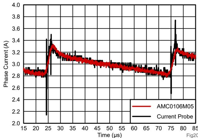
**Figure 4-10. AMC0106M05 Phase Current  $I_W$  with OSR=32 at 3A versus Current Probe Measurement Over one PWM Cycle**
