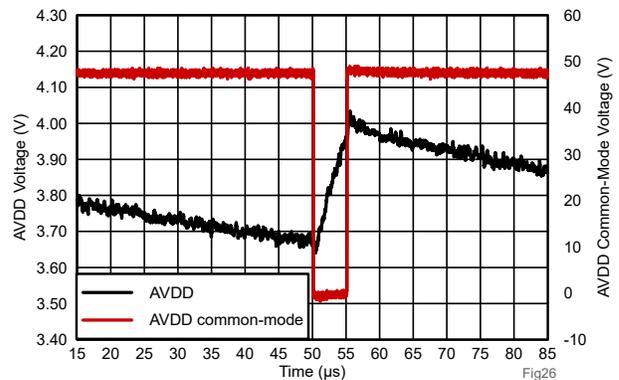
Figure 4-16. Bootstrap Voltage at 10kHz PWM, 95% Duty Cycle
