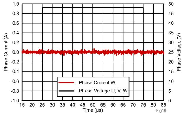
**Figure 4-9. AMC0106M05 Phase Current  $I_W$  with OSR=32 at 0A Over one PWM cycle**
