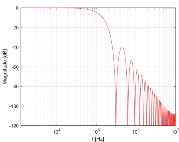
**Figure 3-6. Magnitude Response,  $f_{mod} = 20\text{MHz}$ , sinc<sup>3</sup>, OSR=64**
