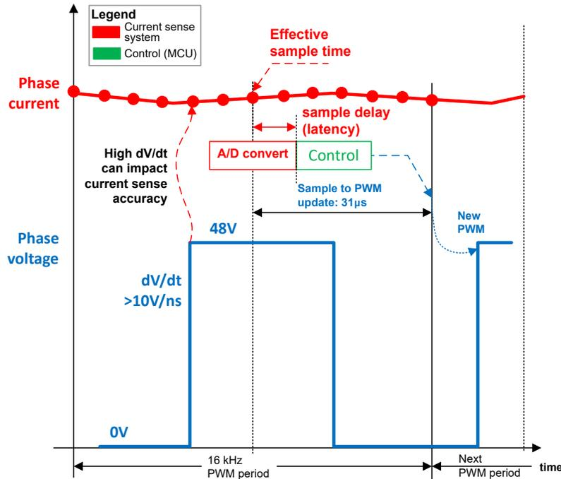
**Figure 2-1. Current Sampling for Closed-Loop Phase Current Control and Short-Circuit Detection**
