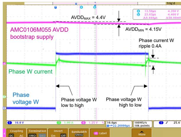
Figure 4-7. Phase W Voltage and Current Over One PWM Cycle
