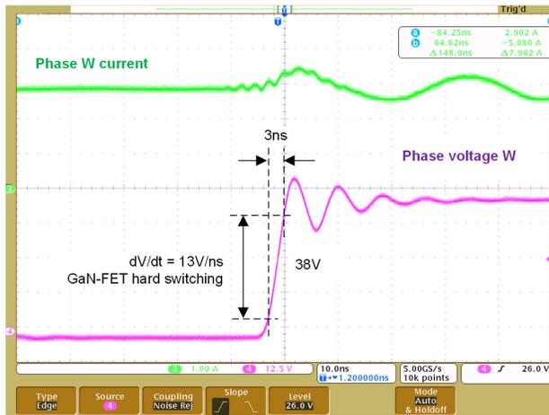
Figure 4-5. Phase W Voltage Rising Edge at 3A Current
