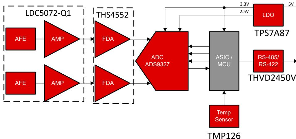
**Figure 2. Inductive Encoder Signal Chain**
