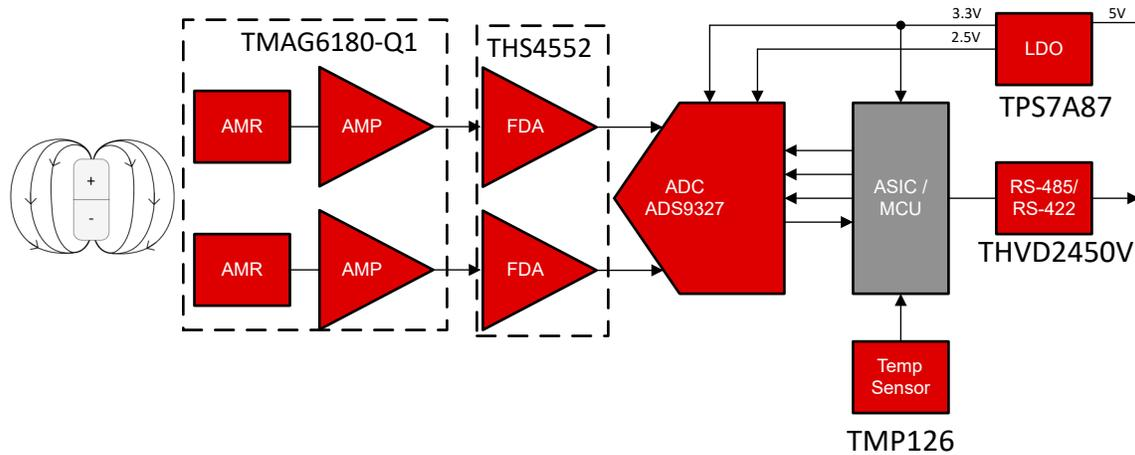
Figure 3. Magnetic Encoder Signal Chain
