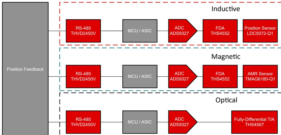
Figure 1. Encoder Signal Chain
