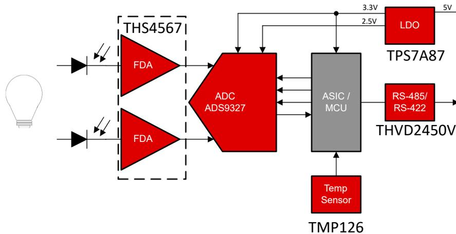
Figure 4. Optical Encoder Signal Chain
