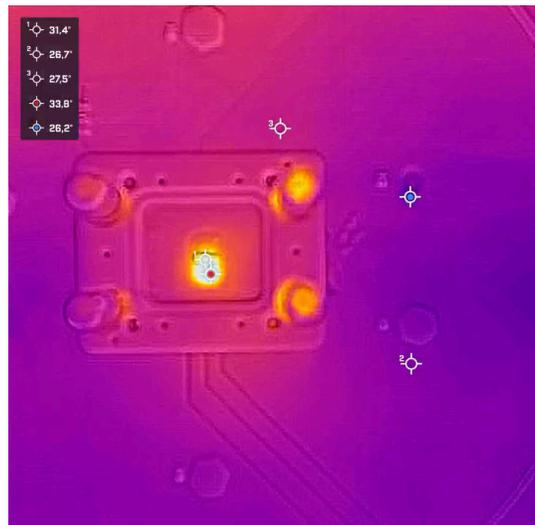
**Figure 2-6. AMC038x Thermal Results: 12.5MΩ**
