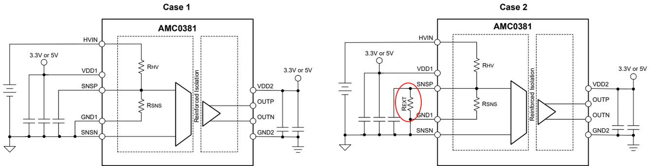
**Figure 2-7. Gain Error Resistor Divider Variation Schematics**
