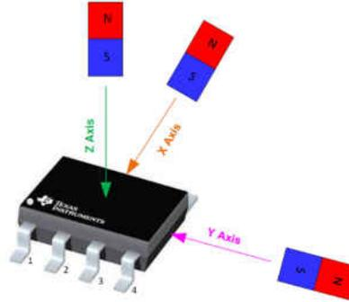
**Figure 3-1. 3D Hall Sensor Axis**
