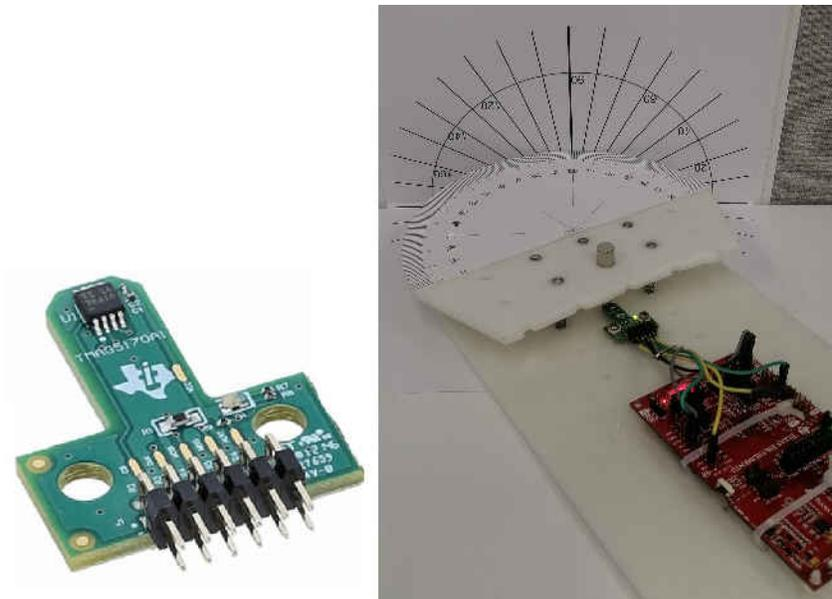
**Figure 6-1. TMAG5170EVM Board and Robot Collision Angle Detecting Demo**
