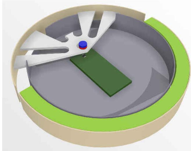
**Figure 4-1. Structure of Mounted Hall Sensor and Magnet**
