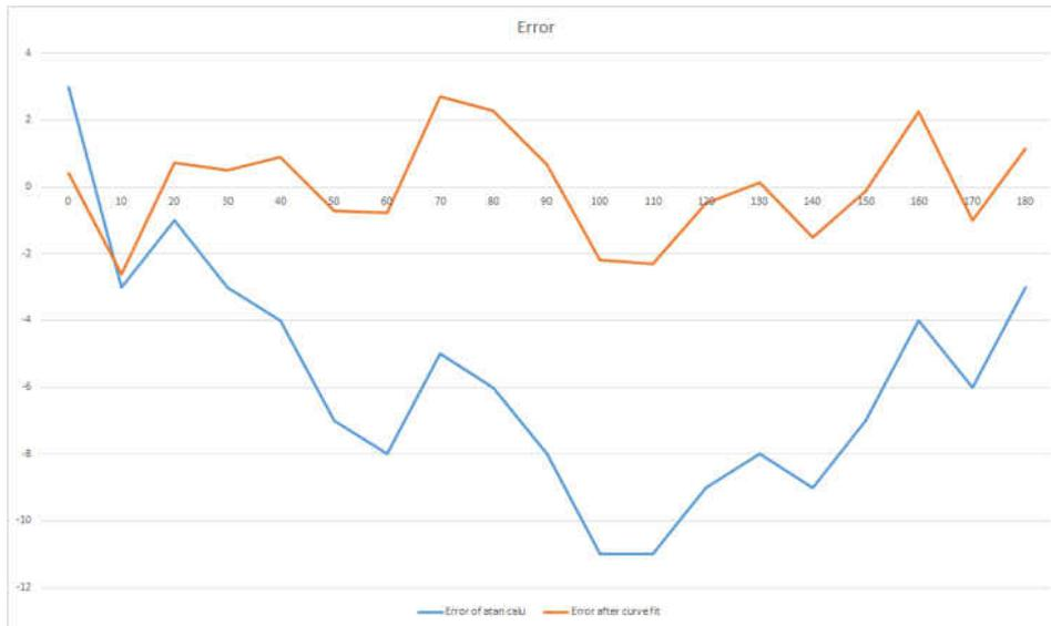
**Figure 6-4. Error of Hall Sensor Output in Demo**
