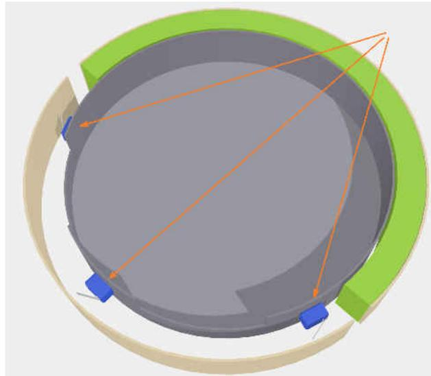
**Figure 2-1. Switch on Vacuum Robot**
