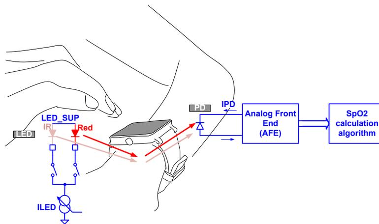
Figure 1.  $SpO_2$  Measurement on a Wearable Device
