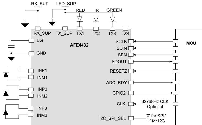
**Figure 2. Reference Schematic for an SPO<sub>2</sub> System Using AFE4432**
