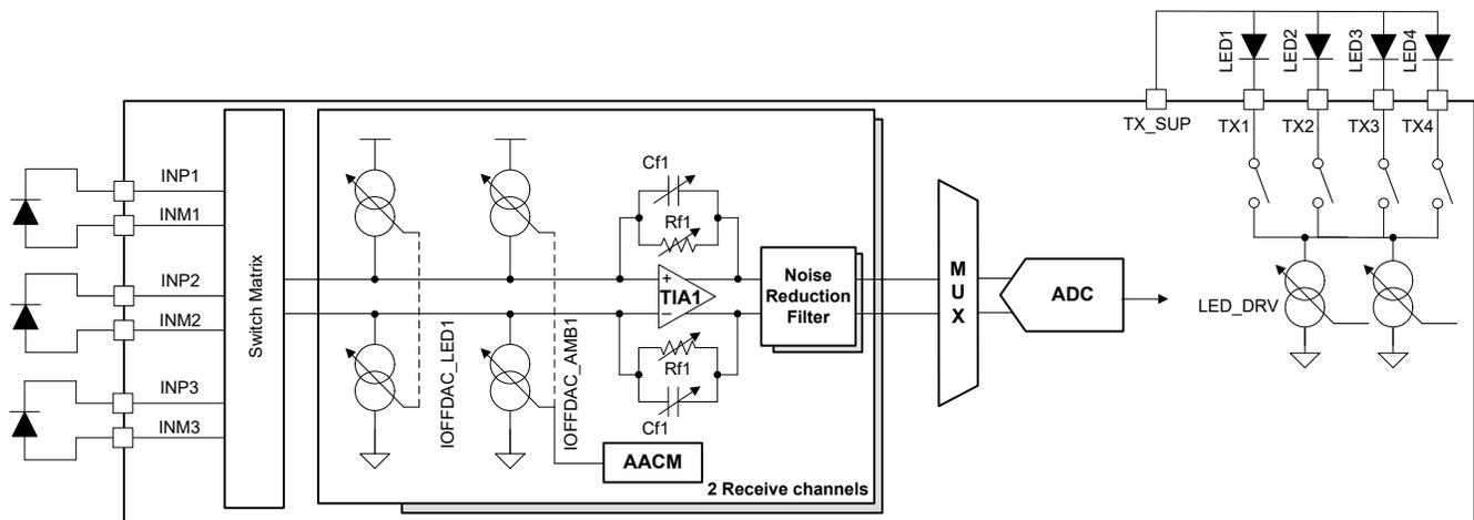
**Figure 3. PPG Signal Chain in AFE4432**
