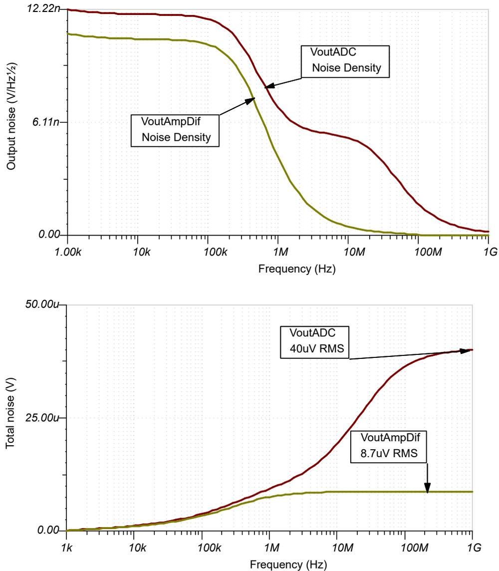
Figure 1-6. RMS Noise at Amplifier Output and ADC Output
