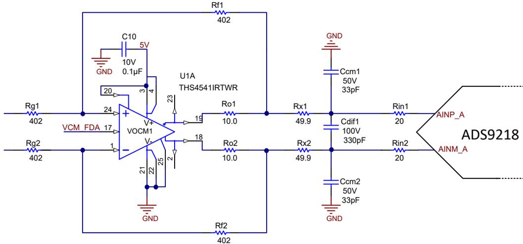
**Figure 1-2. Signal Chain Optimized for 1 MHz With THS4551**
