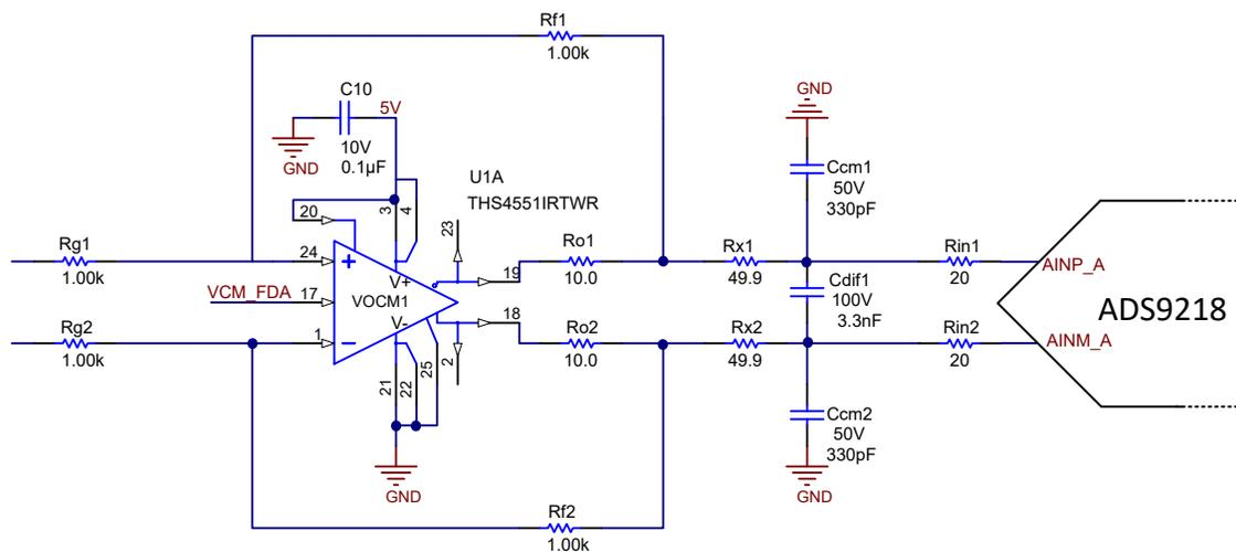
Figure 1-1. Differential Front End for ADS9218
