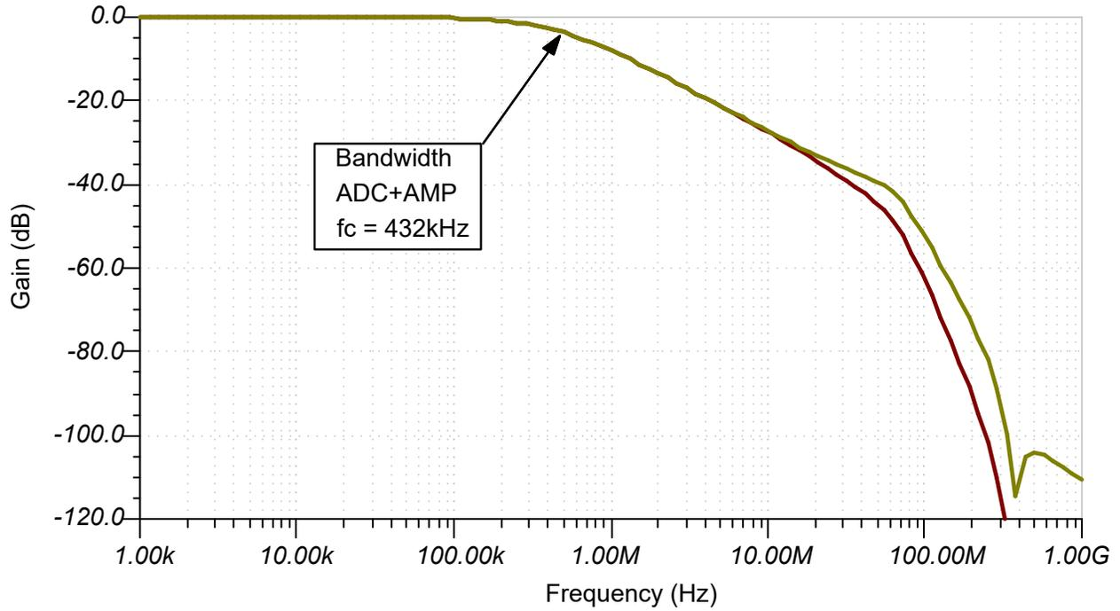
Figure 1-4. AC Transfer Characteristics ( $f_c = 432$  kHz)
