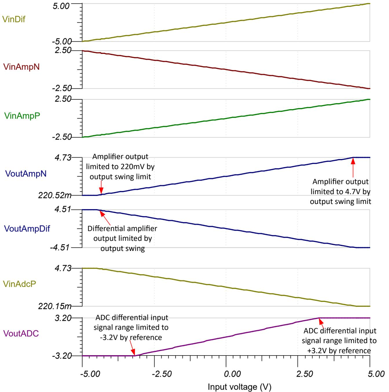
**Figure 1-5. DC Transfer Characteristics ( $V_{cmi} = 0.0$  V,  $V_{cmo} = 2.048$  V,  $V+ = 5$  V)**
