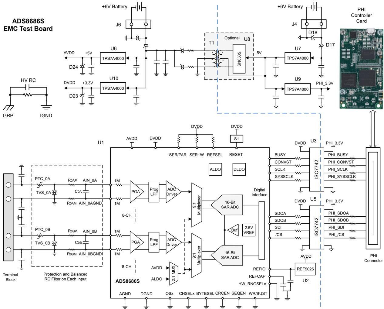
Figure 2-1. ADS8686S EMC Test Board Circuit
