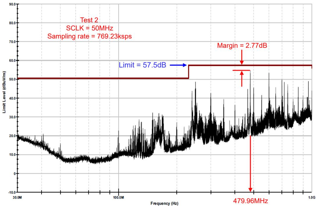
Figure 3-16. Test 2 - Measured Radiated Emission, Horizontal Antenna Polarization
