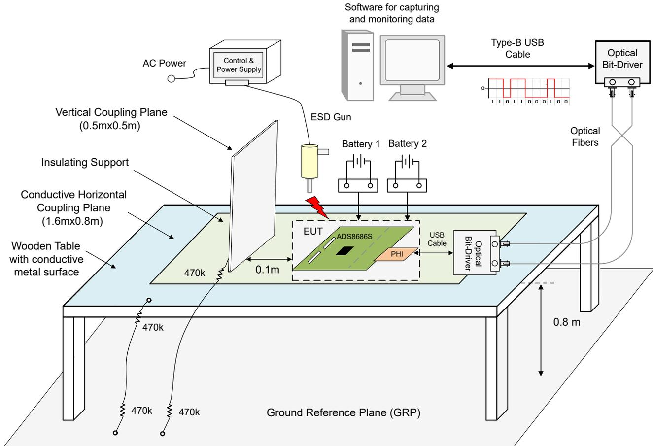
Figure 3-3. Diagram of Laboratory Setup for ESD Test
