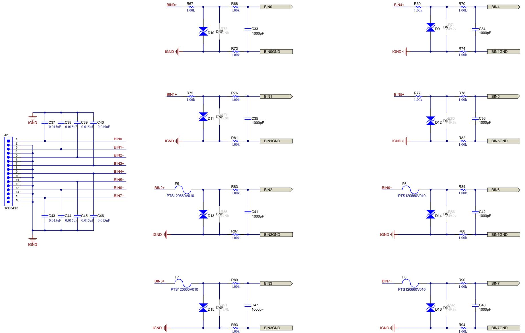
Figure 4-3. Schematic – Input of ADC - B
