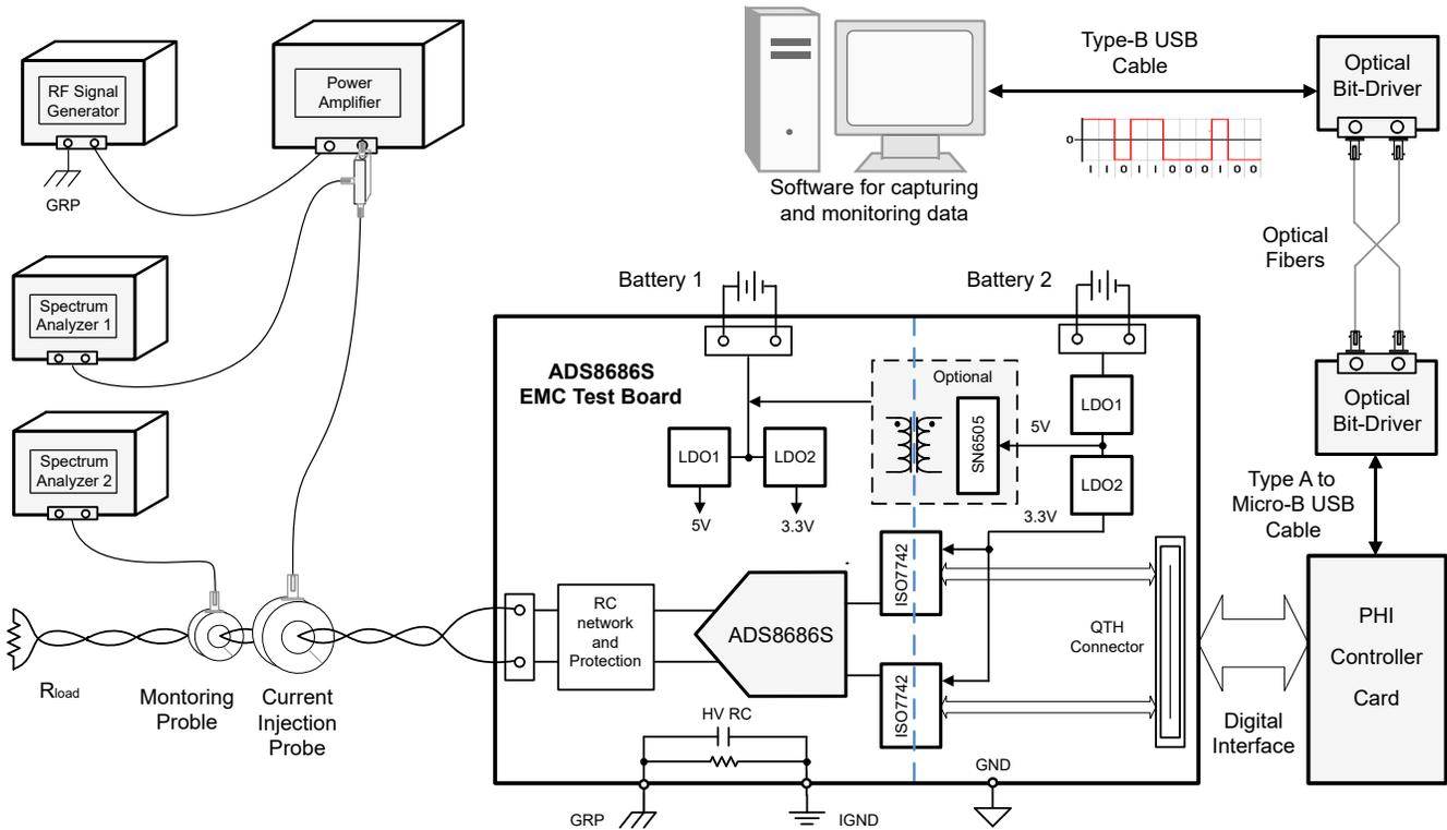
Figure 3-8. Diagram of Laboratory Setup for Conducted Immunity Test
