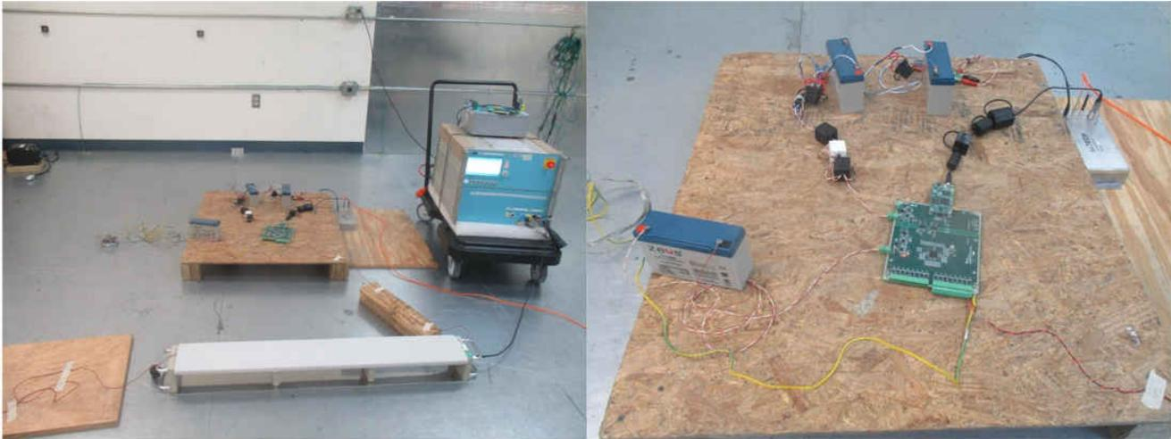
**Figure 3-2. Photograph of Laboratory Setup for EFT Test**
