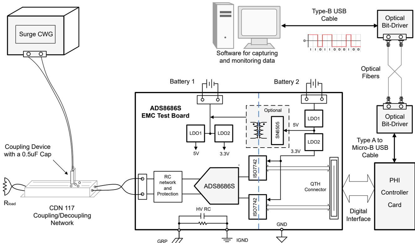
Figure 3-6. Diagram of Laboratory Setup for Surge Test
