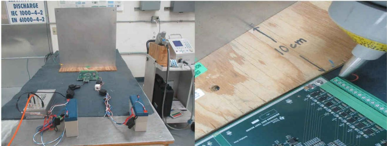
**Figure 3-5. Photograph of Laboratory Setup for ESD Test**
