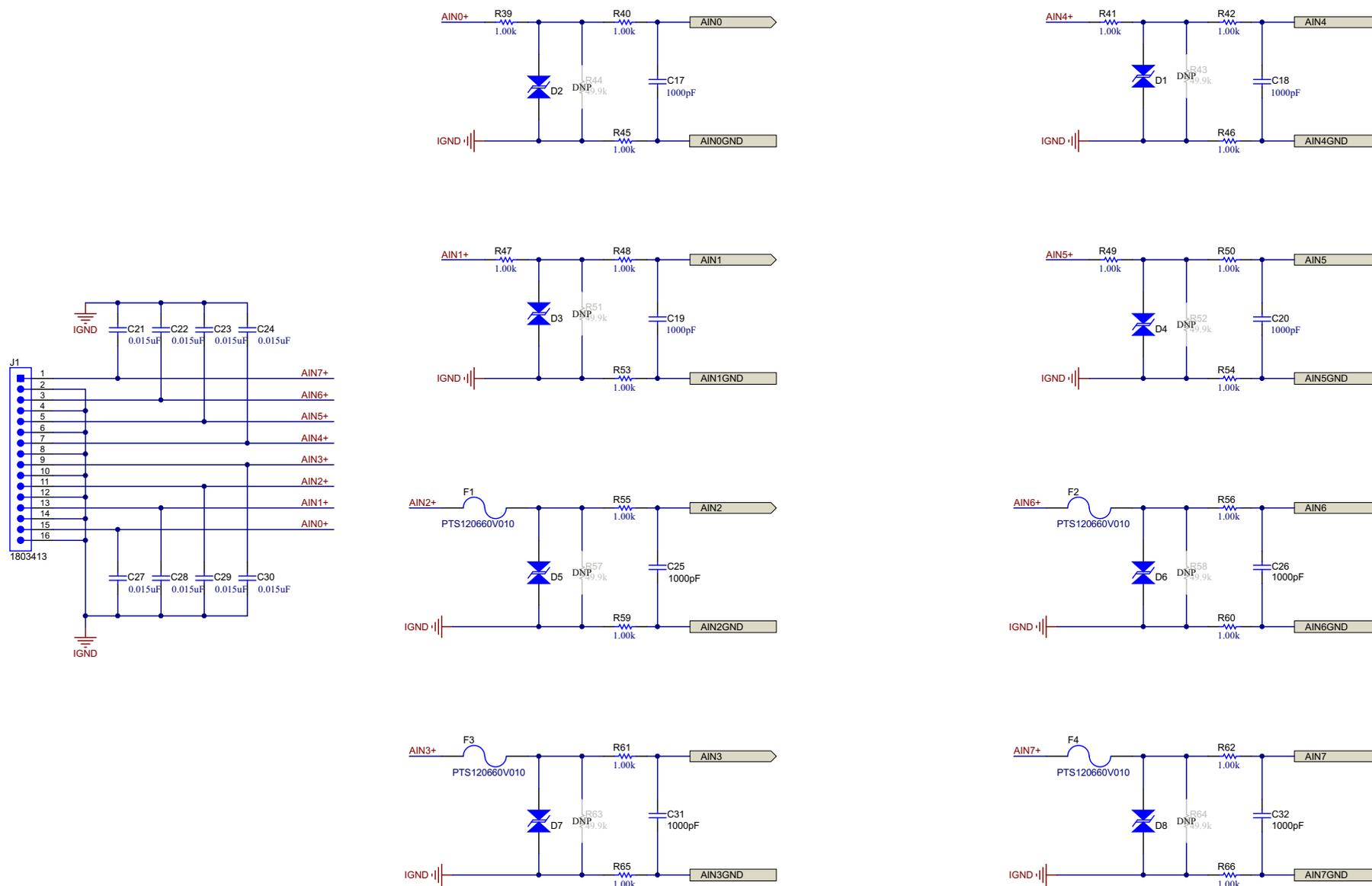
Figure 4-2. Schematic – Input of ADC - A
