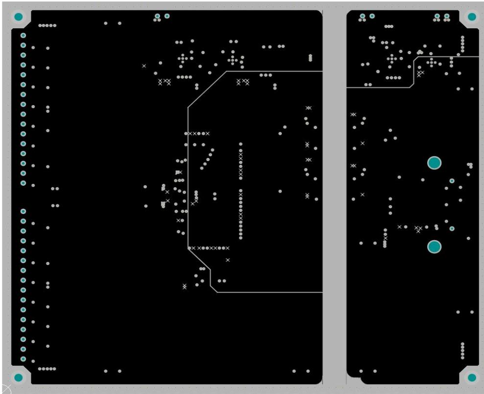
**Figure 5-3. Layout – Inner Power Layer**
