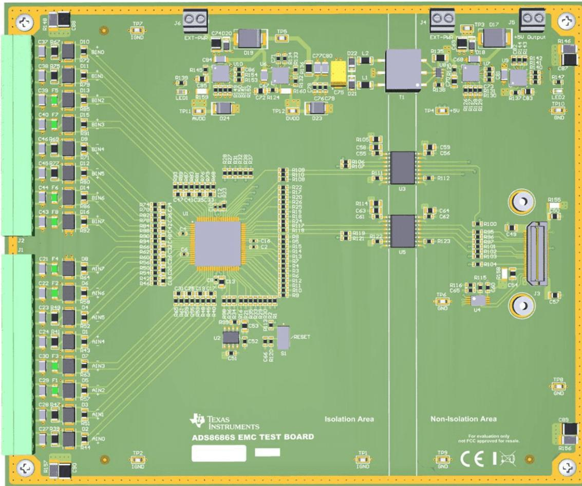
Figure 1-1. ADS8686S EMC Test Board
