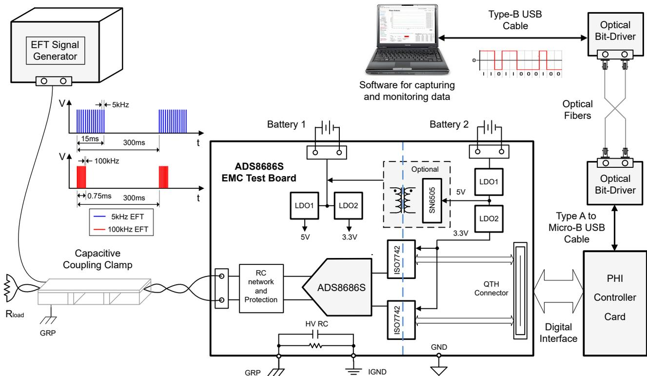
Figure 3-1. Diagram of Laboratory Setup for EFT Test
