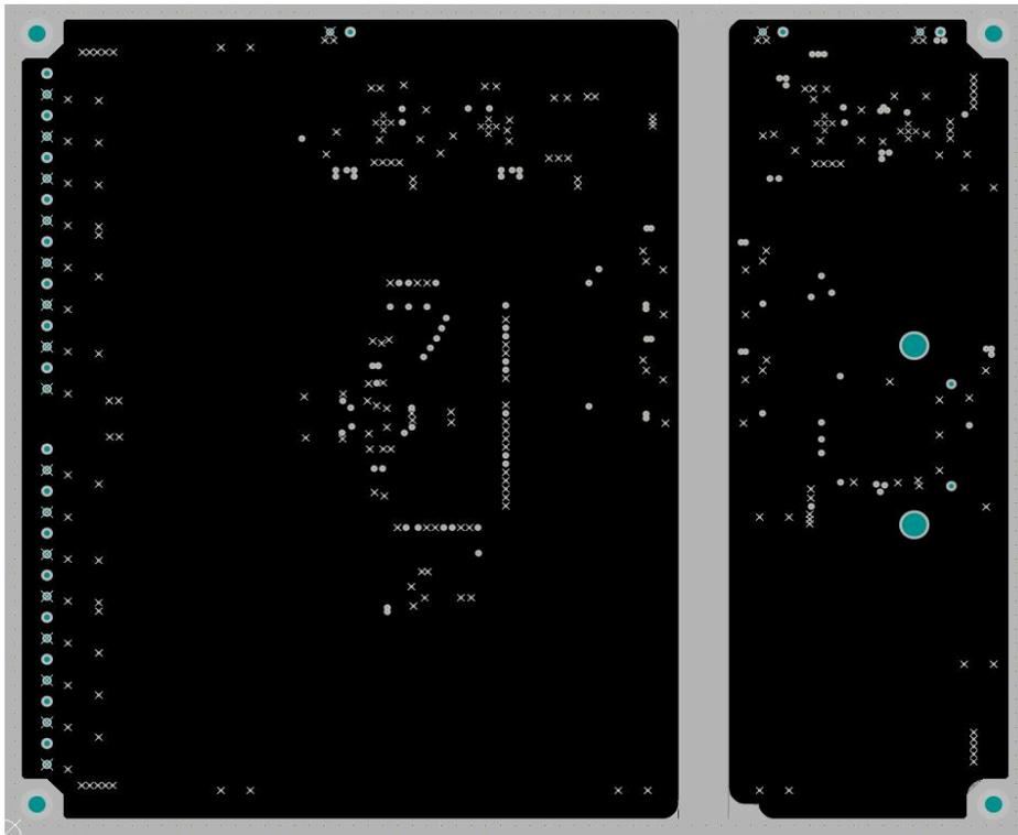
Figure 5-2. Layout – Inner Ground Layer
