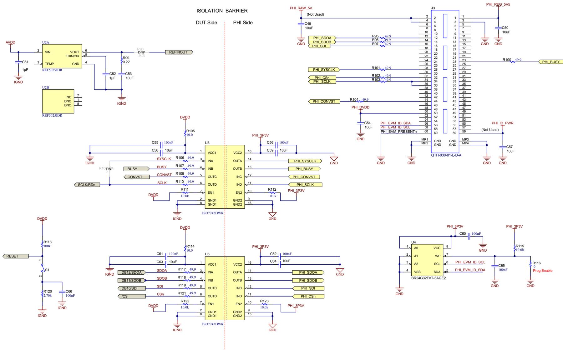
Figure 4-4. Schematic – Digital Isolation
