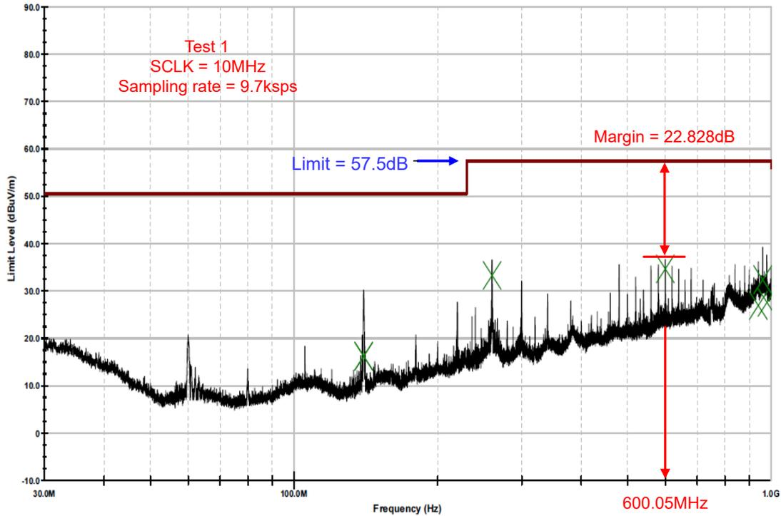
Figure 3-15. Test 1 - Measured Radiated Emission, Horizontal Antenna Polarization
