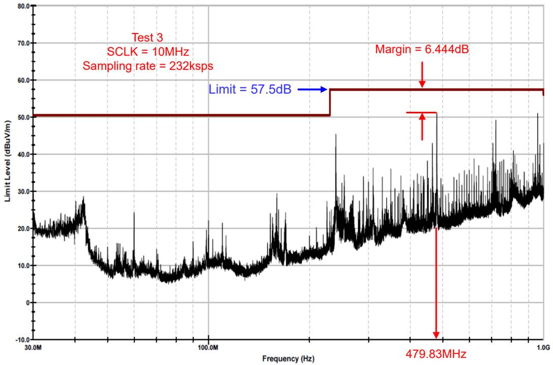
Figure 3-17. Test 3 - Measured Radiated Emission, Vertical Antenna Polarization
