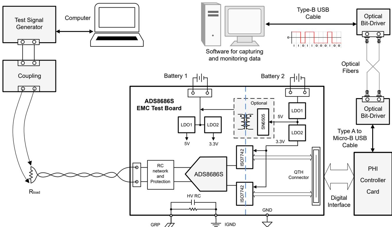
Figure 2-3. General EMC Test Setup
