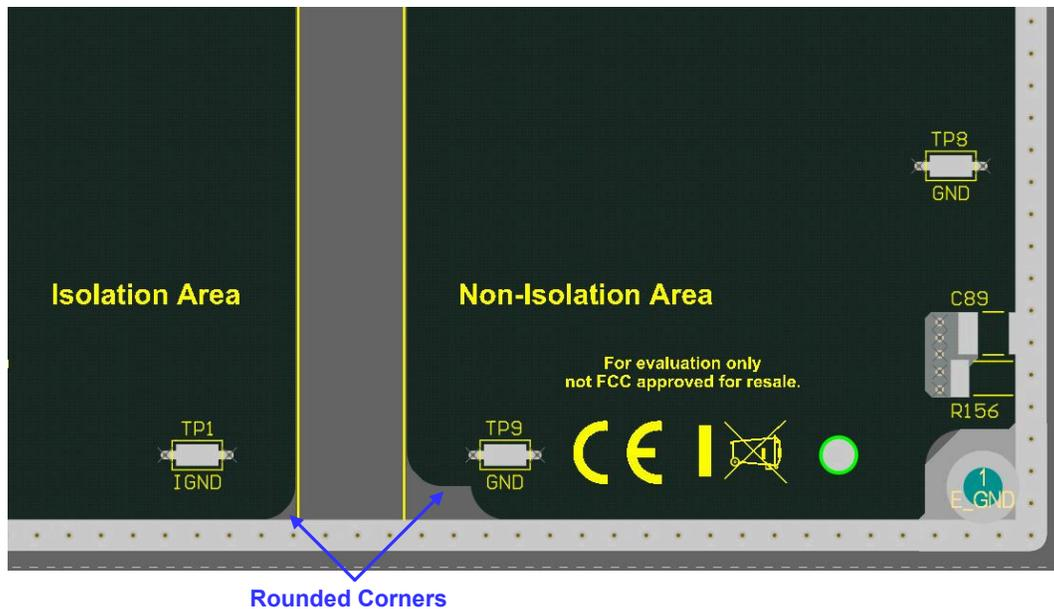
Figure 2-2. PCB Layout Design – Plane Edge on Inner Negative Layer
