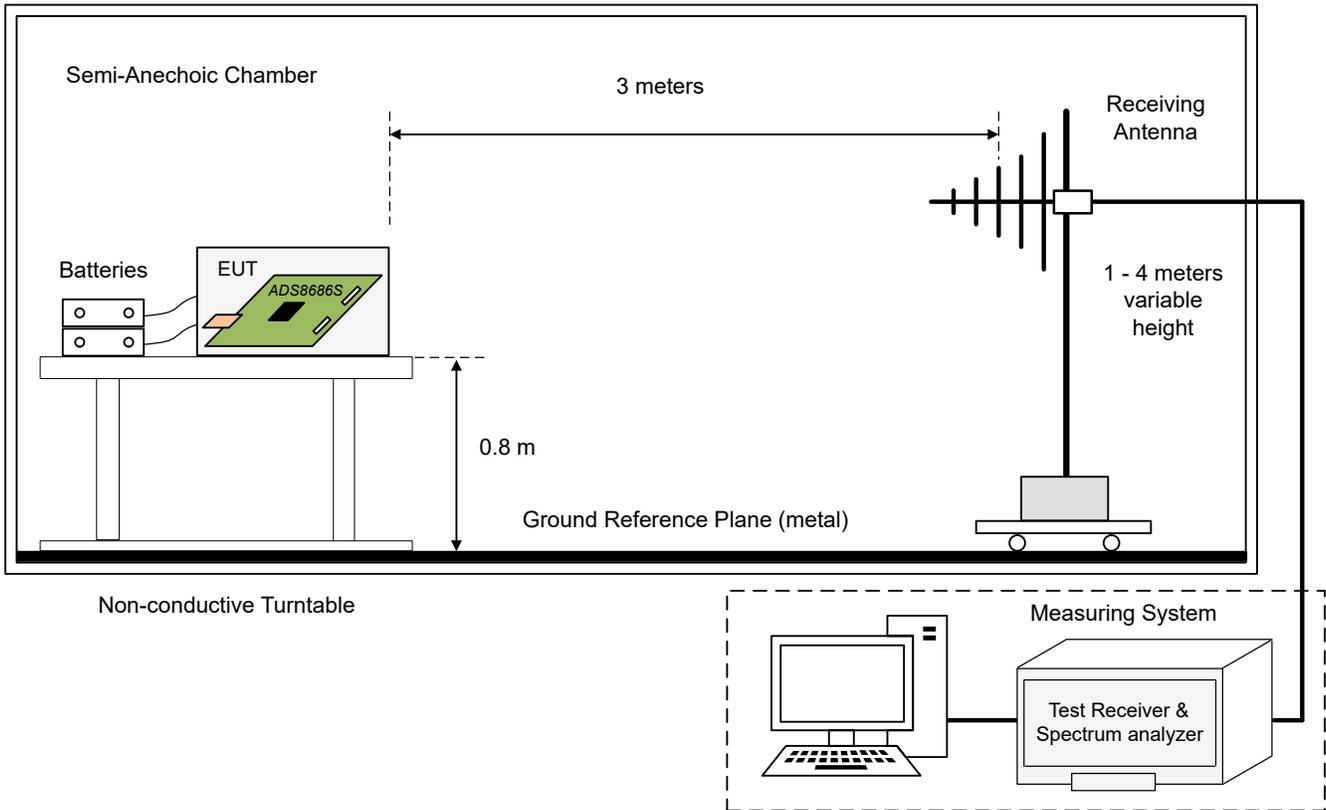
Figure 3-13. Diagram of Laboratory Setup for Radiated Emission Test
