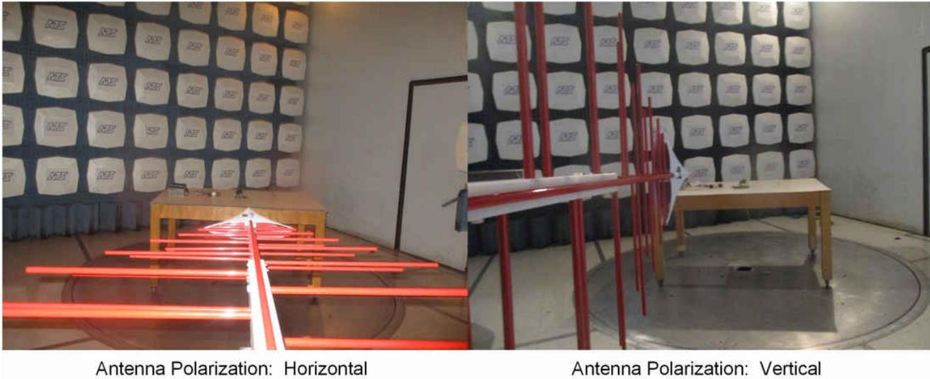
Figure 3-14. Photograph of Laboratory Setup for Radiated Emission Test
