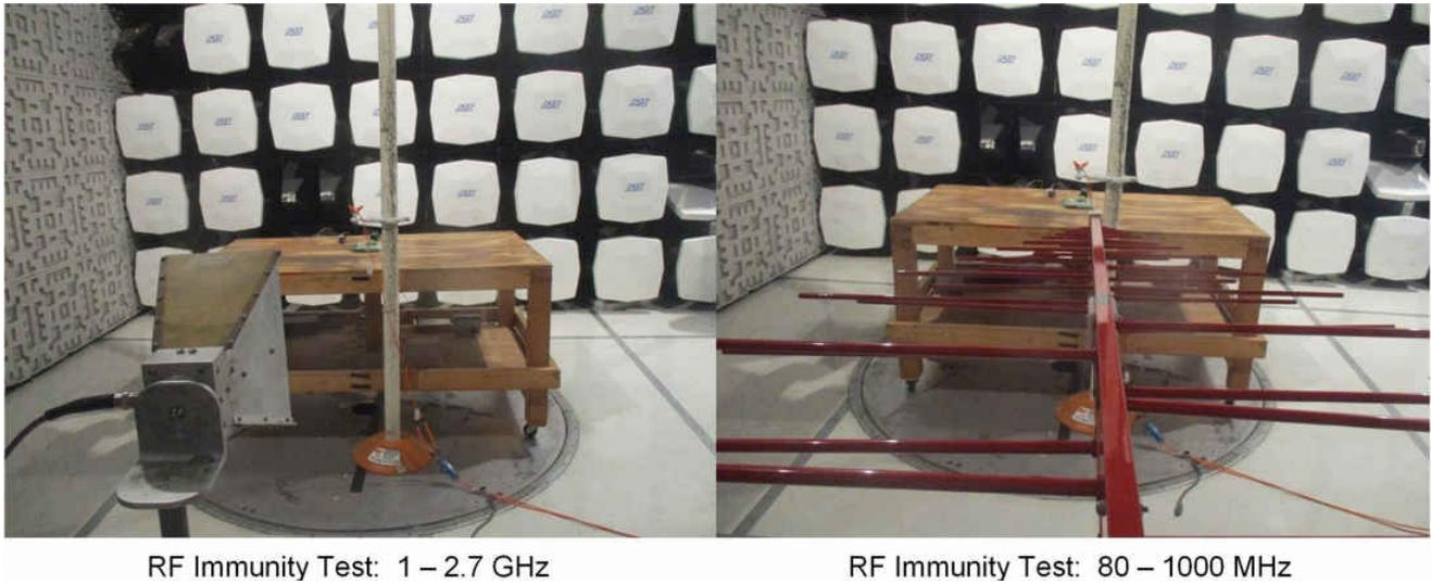
**Figure 3-11. Photograph of Laboratory Setup for Radiated Immunity Test**
