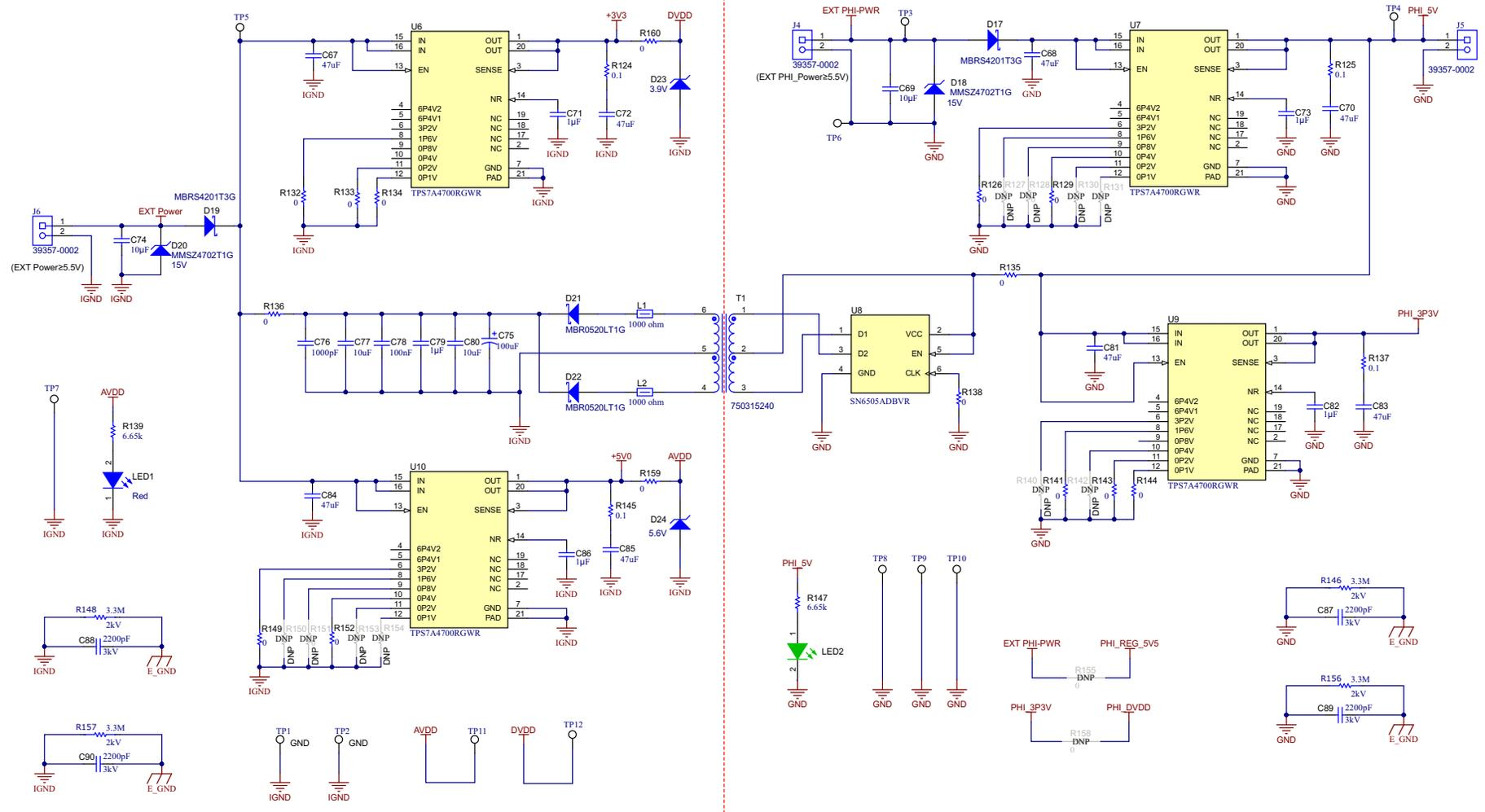
Figure 4-5. Schematic – Power Supply
