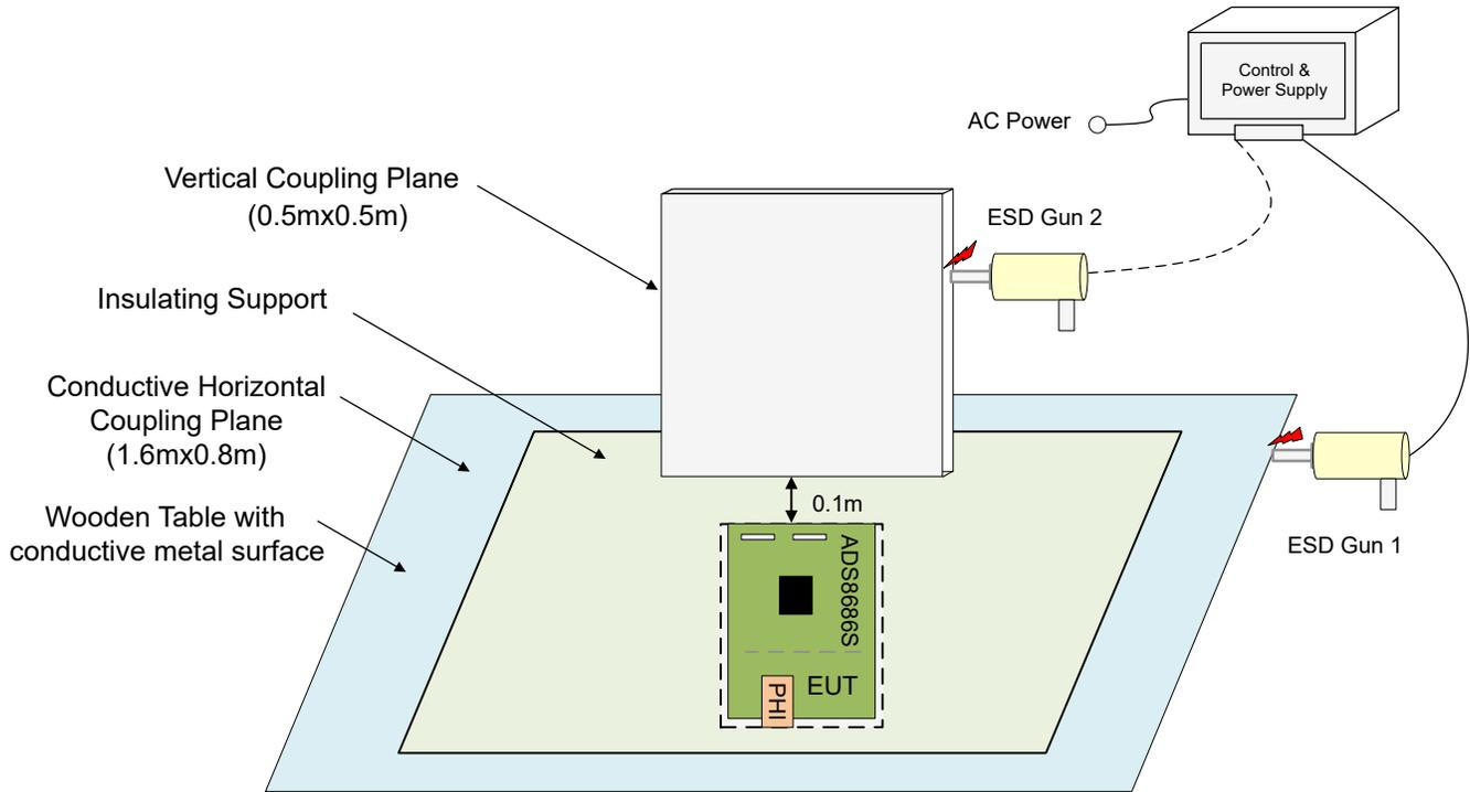
**Figure 3-4. Discharges to the HCP and VCP With ESD Gun 1 and 2**
