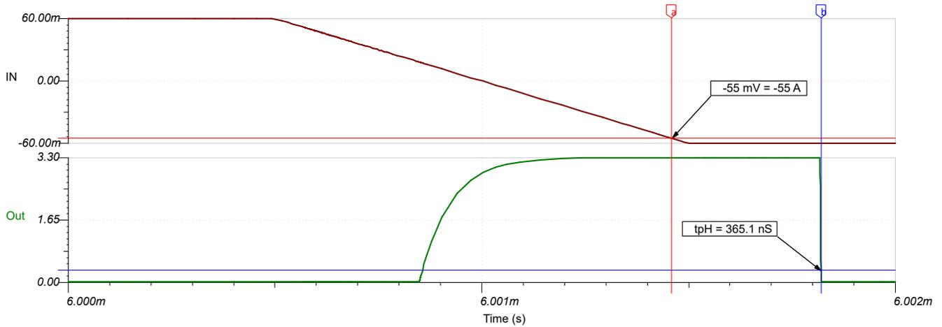
Transient Response of Overcurrent Protection Simulation - Falling
