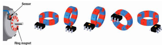
**Figure 4. Rotary Encoding Using Ring Magnets, and Various Sensor Placements**
