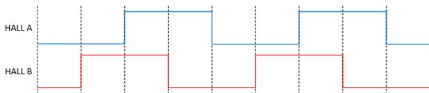
**Figure 2. 2-Bit Quadrature Output**
