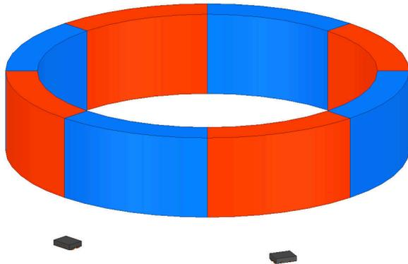
**Figure 3. Magnetic Incremental Encoder**
