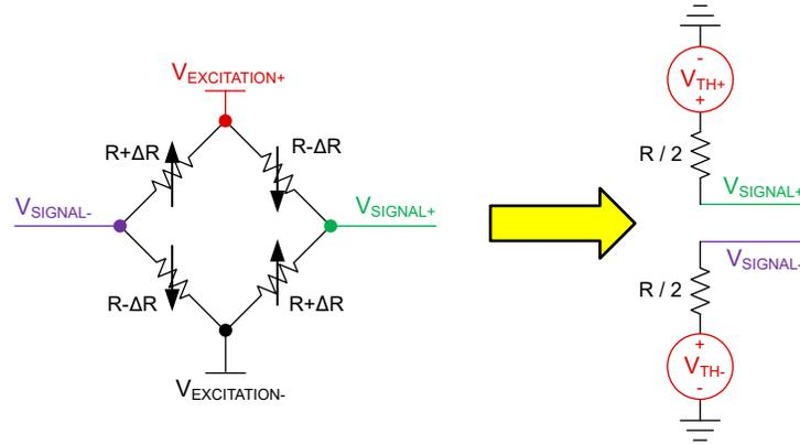
Figure 6-15. Thevenin Equivalent of a Single Bridge Circuit
