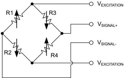
Figure 3-2. Connections for a Four-Wire Bridge
