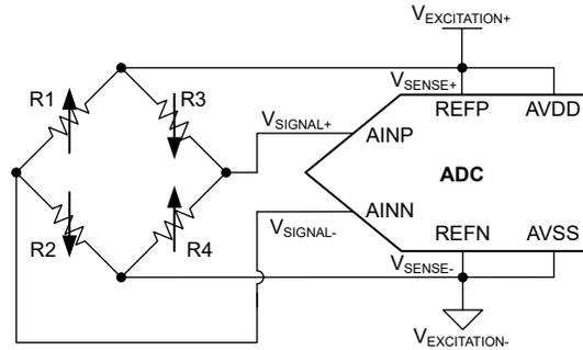
**Figure 3-1. Example of a Ratiometric Bridge Measurement**
