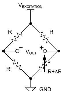
**Figure 1-1. Basic Configuration of a Simple Bridge Circuit**
