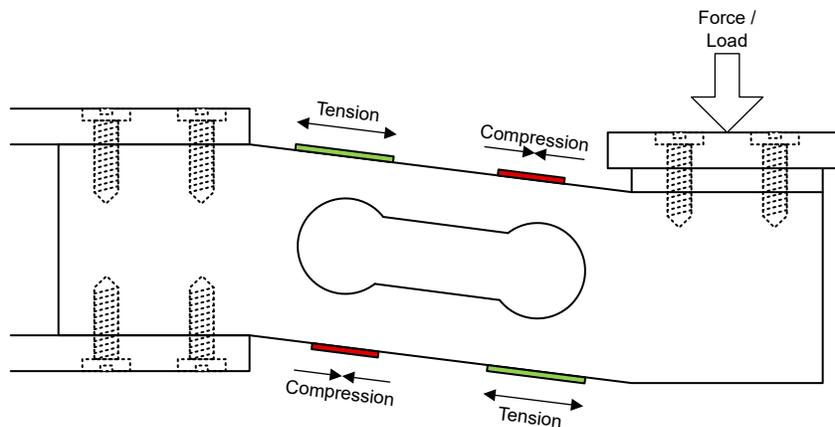
**Figure 2-11. Single-Point Load Cell With Approximate Positions and Responses of the Four Strain Gauges**
