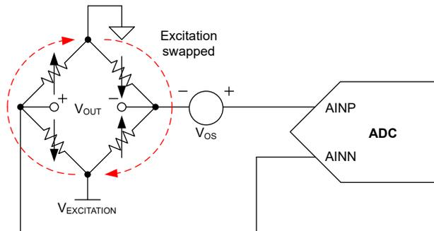
**Figure 5-10. Bridge Measurement During AC Excitation (Phase 2)**
