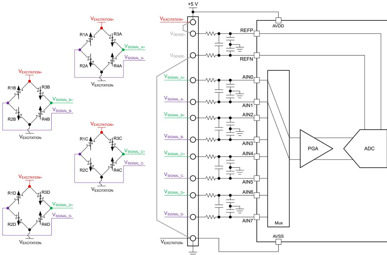
Figure 6-19. Measuring Multiple Four-Wire Resistive Bridges in Parallel Using a Multichannel ADC With a Ratiometric Reference and a Unipolar, Low-Voltage ( $\leq 5$  V) Excitation Source
