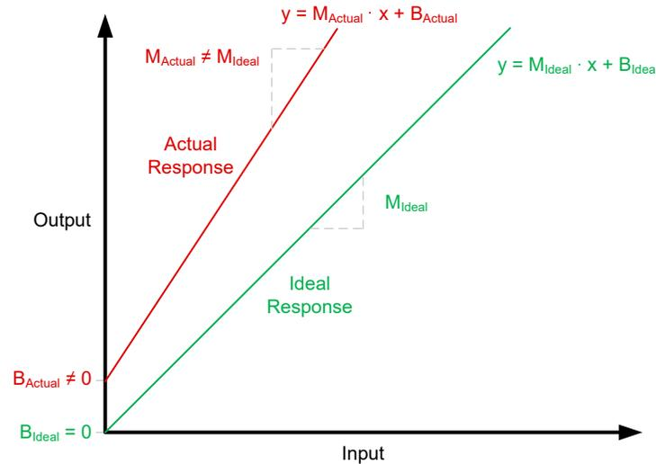
**Figure 5-11. Bridge Measurement Response: Ideal vs Actual**
