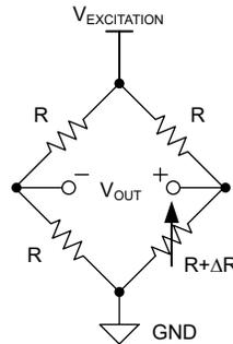
**Figure 2-1. Bridge With One Active Element (Quarter Bridge)**
