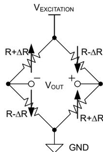
**Figure 2-8. Bridge With Four Active Elements (Full Bridge)**
