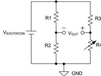
**Figure 1-3. A Simple Bridge Using a Differential Measurement Across Two Resistive Paths**
