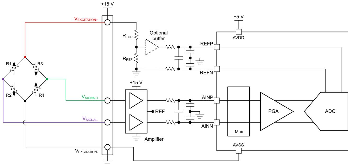
Figure 6-3. Four-Wire Resistive Bridge Measurement With a Pseudo-Ratiometric Reference and a Unipolar, High-Voltage (> 5 V) Excitation Source
