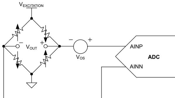
**Figure 5-9. Bridge Measurement During AC Excitation (Phase 1)**
