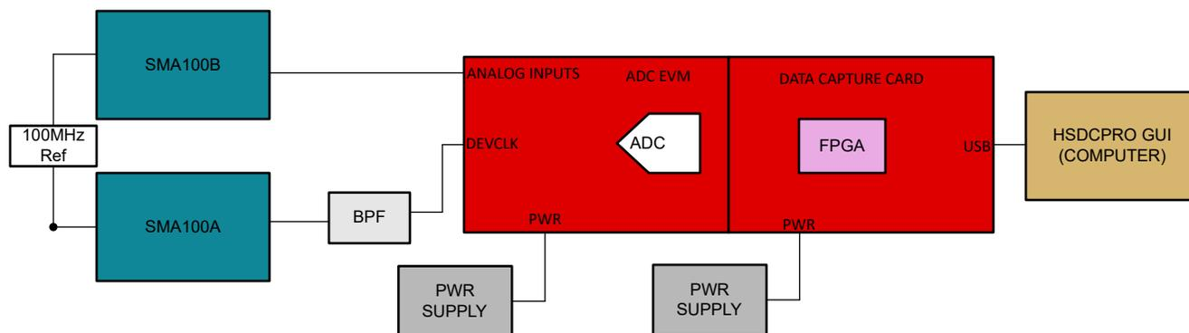
Figure 2-4. Test Configuration for SNR, SFDR, HD, and NSD Measurement
