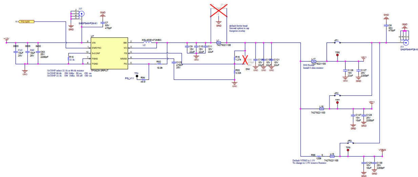
**Figure A-2. TPS6913 1.1V ADC Power Schematic**
