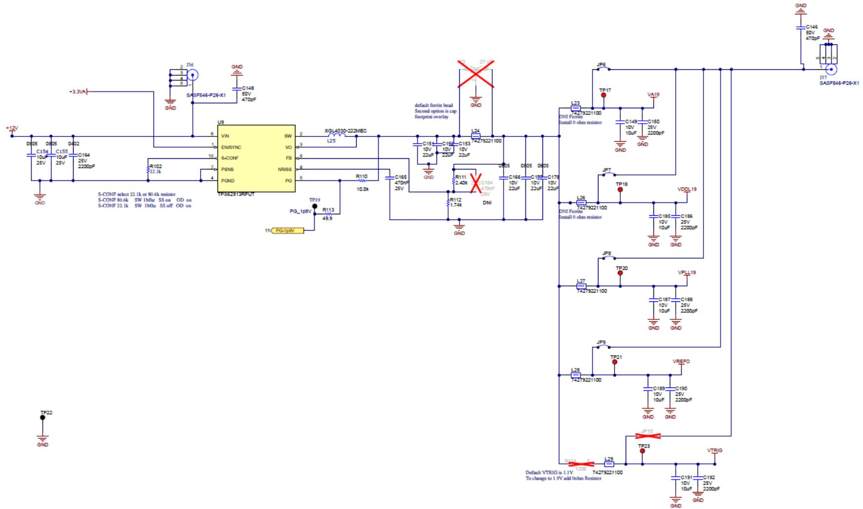
Figure A-3. TPS62913 1.9V ADC Power Schematic
