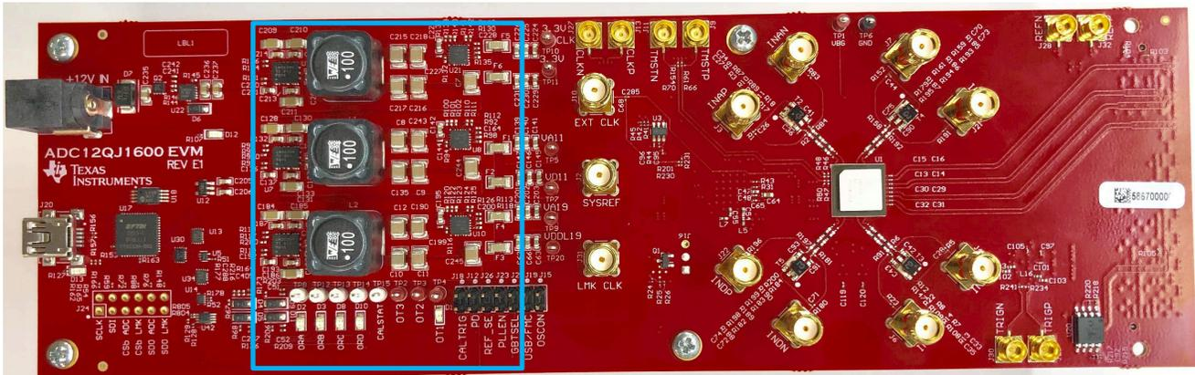
Figure 1-5. Image of Board With Switchers and LDO's Outlined in Blue
