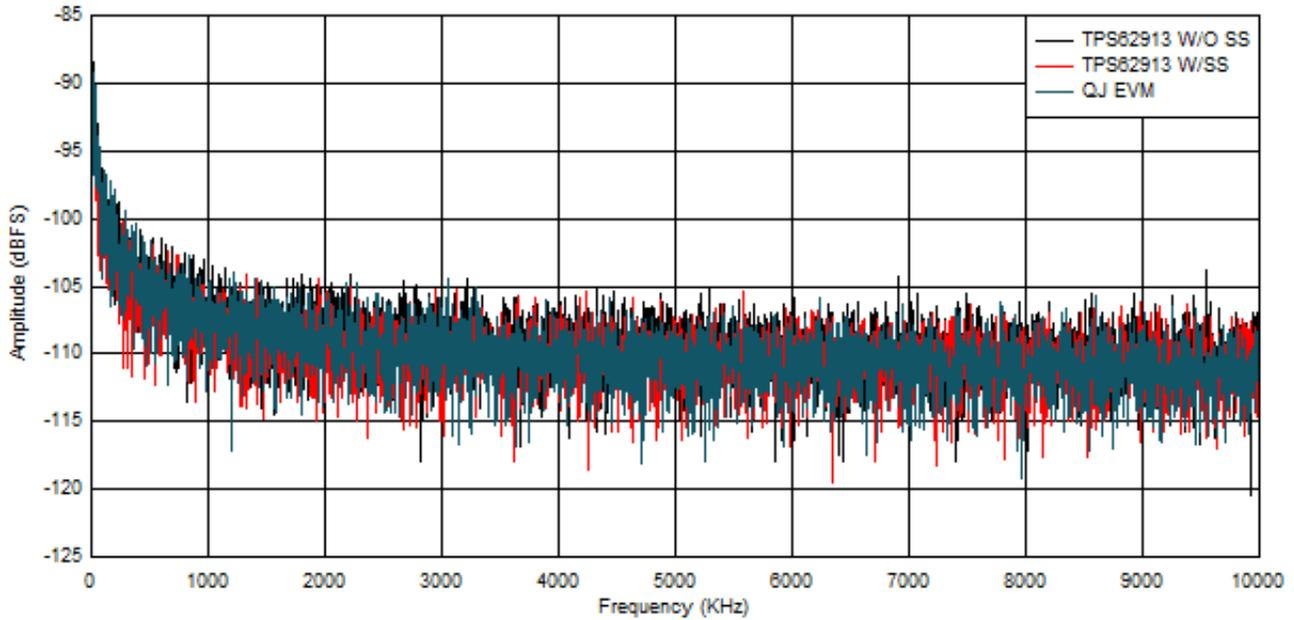
**Figure 2-9. PSMR Comparison of Original and TPS62913 at DC**
