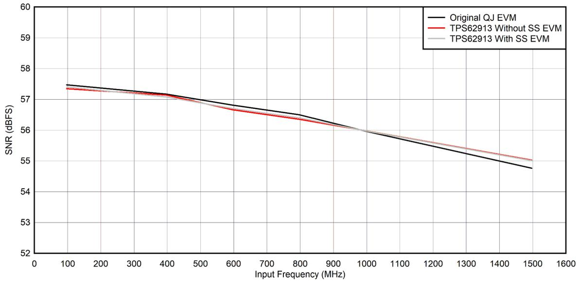
**Figure 2-5. Signal to Noise (SNR) Comparison Graph**
