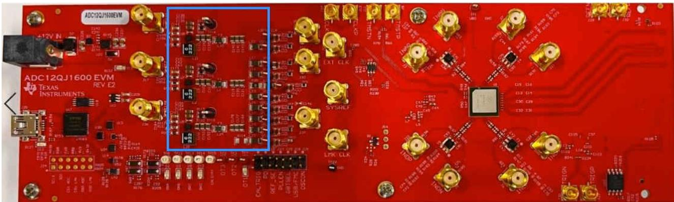
**Figure 1-7. Image of Board With TPS62913 Switchers Outlined in Blue**
