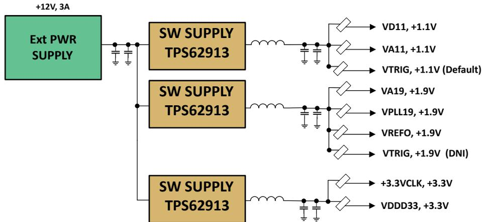
**Figure 1-6. Power Block Diagram for ADC12QJ1600-Q1 Rev E2 Evaluation Module With TPS62913**
