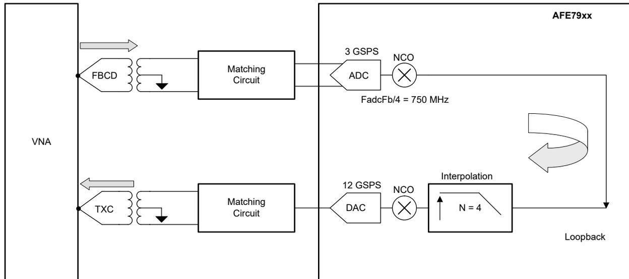
Figure 1-2. ADC to DAC Low Latency Loopback
