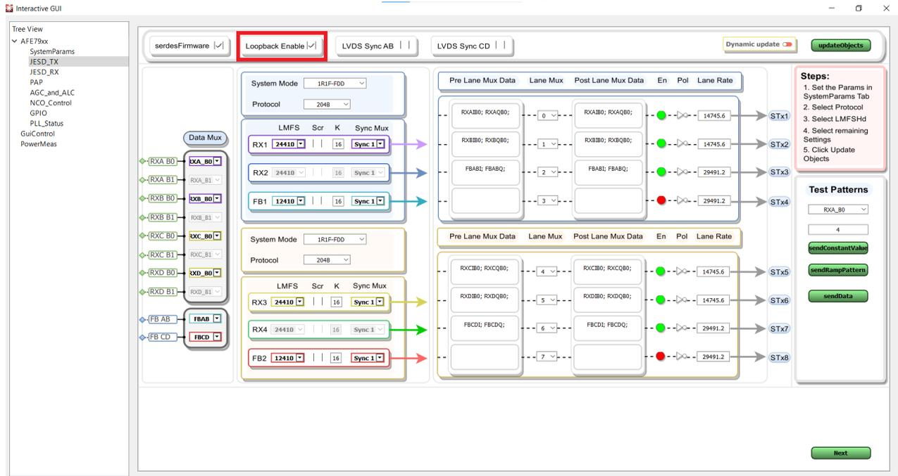
Figure 2-3. ADC to DAC JESD Loop Back Enable Mode
