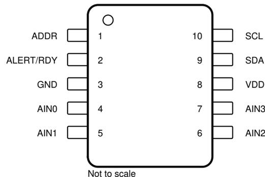
**Figure 4-1. Pin Diagram (VSSOP) Package**
