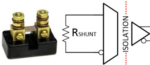
Figure 1. Isolated Shunt Based Current Sensing
