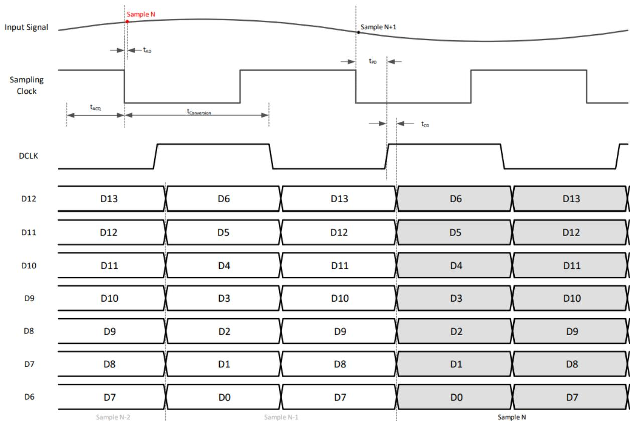
**Figure 2-4. Parallel CMOS DDR Timing Diagram**
