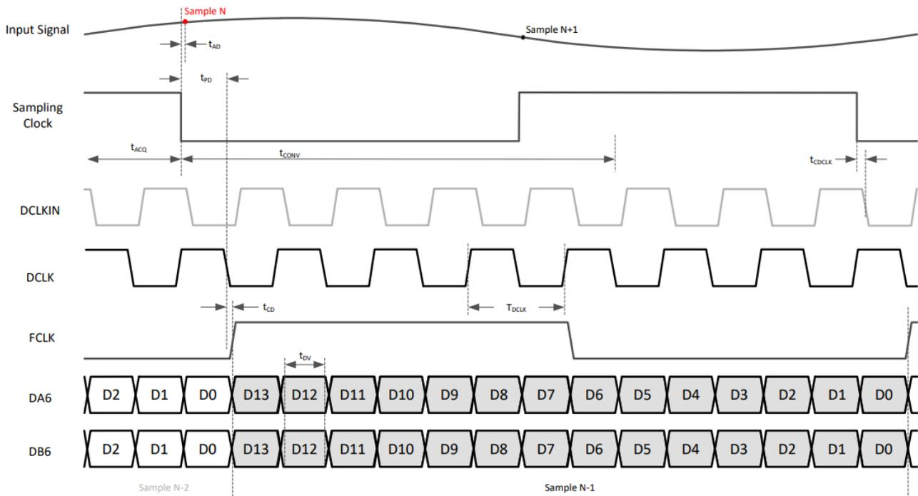
**Figure 2-8. Serial CMOS 1W Timing Diagram**
