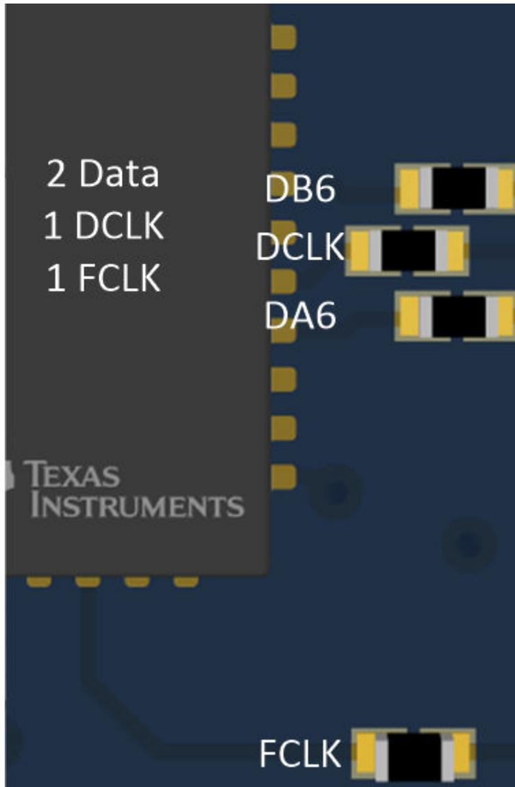
**Figure 2-7. ADC3643 Serial CMOS: 1 Wire Resistors**
