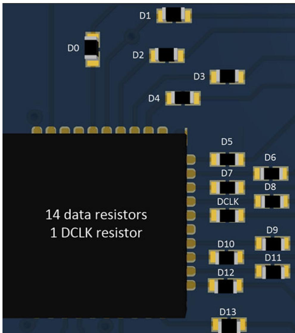
Figure 2-1. Parallel CMOS: 14 bit SDR Resistors
