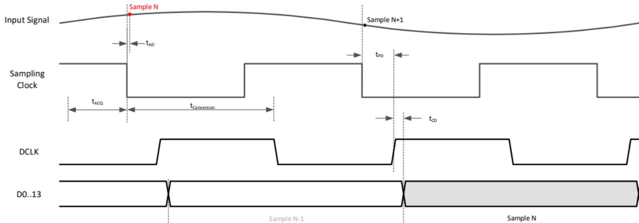
**Figure 2-2. Parallel CMOS SDR Timing Diagram**
