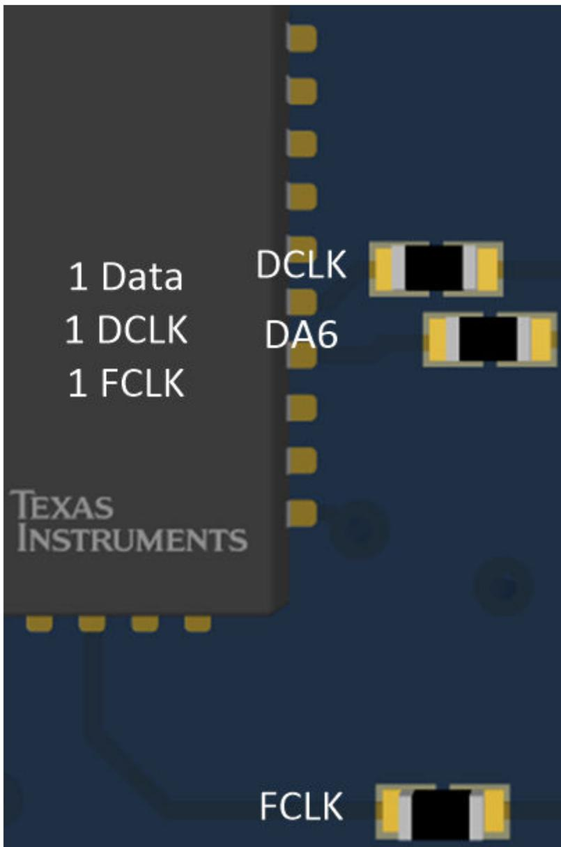
**Figure 2-9. ADC3643 Serial CMOS: 0.5 Wire Resistors**
