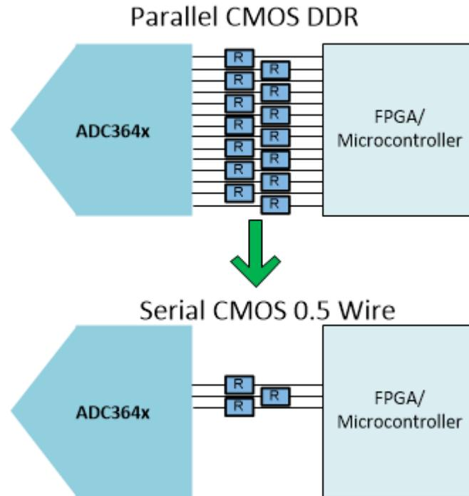
**Figure 1-1. ADC3643 2CH CMOS Interfaces**
