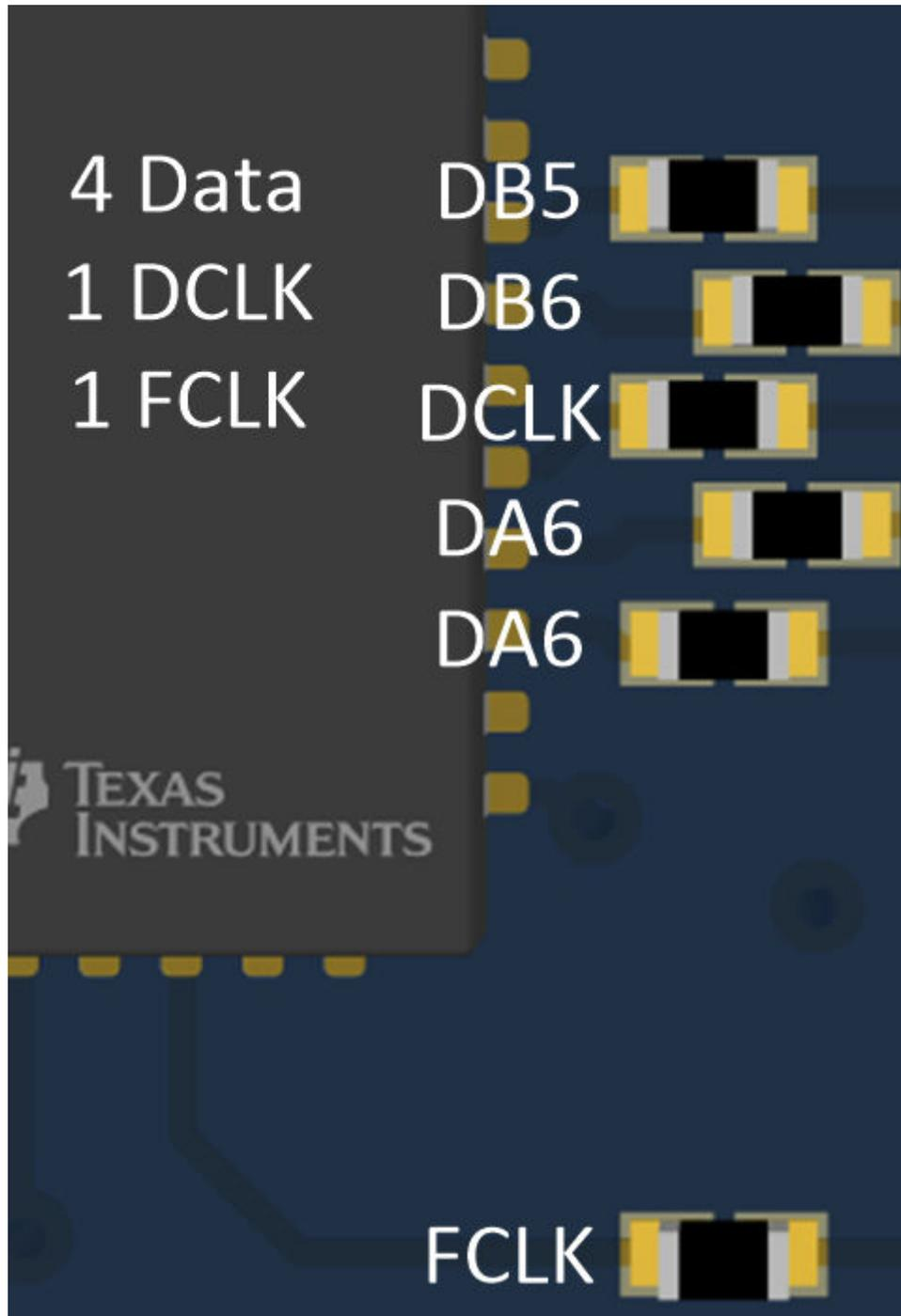
**Figure 2-5. ADC3643 Serial CMOS: 2 Wire Resistors**
