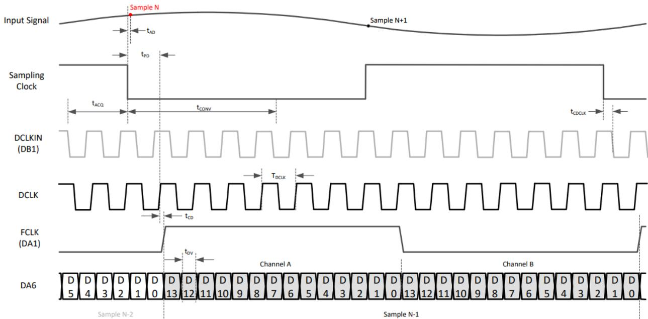
**Figure 2-10. Serial CMOS 0.5W Timing Diagram**
