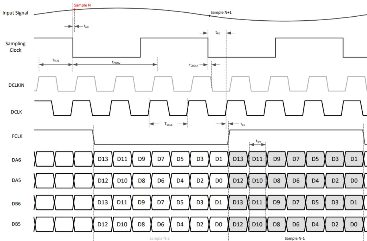
**Figure 2-6. Serial CMOS 2W Timing Diagram**
