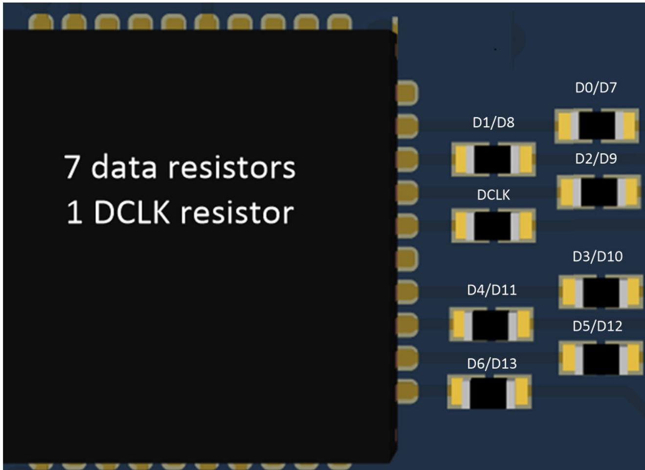
**Figure 2-3. Parallel CMOS: 14 bit DDR resistors**
