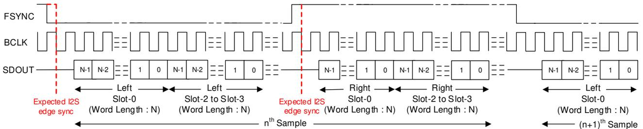
**Figure 3-1. Default I<sup>2</sup>S in Controller Mode (TX\_Offset = 0) Showing Incompatible FS<sub>SYNC</sub> Edge Sync**
