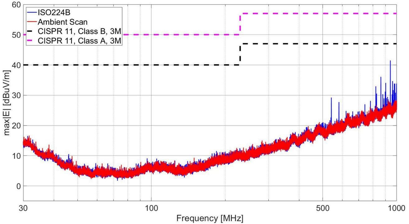
Figure 3-1. ISO224 CISPR 11 Radiated Emissions EMI Scan
