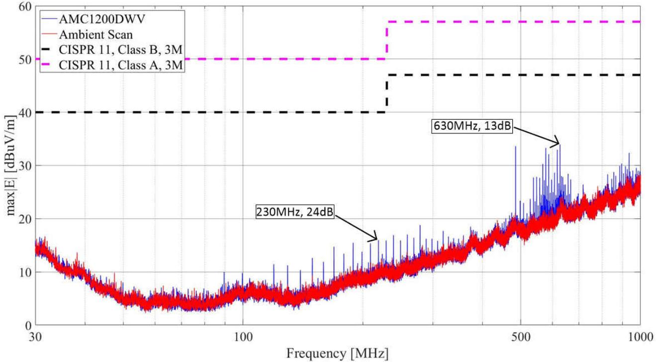
**Figure 3-2. AMC1200 CISPR 11 Radiated Emissions EMI Scan**
