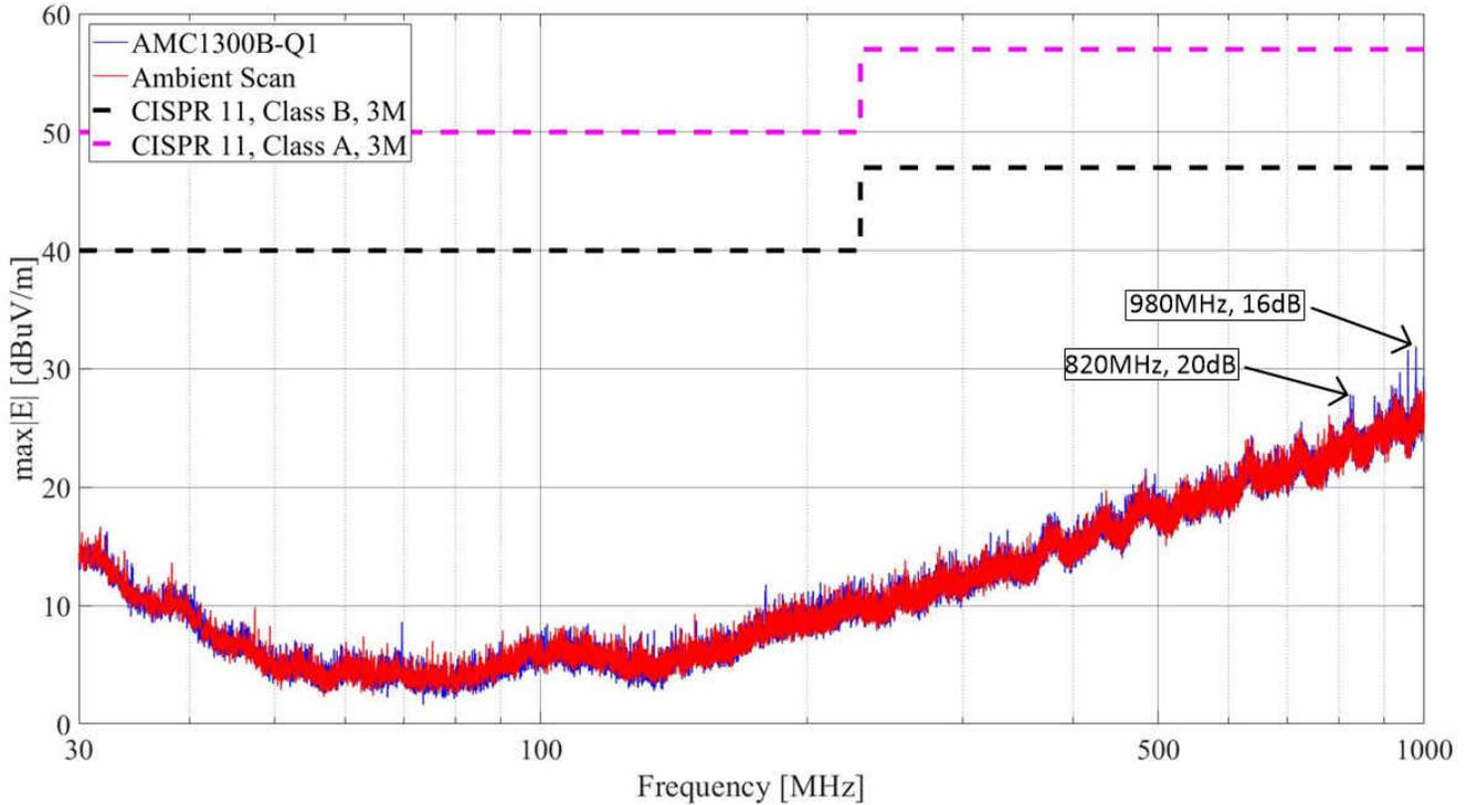
Figure 2-1. AMC1300B-Q1 CISPR 11 Radiated Emissions EMI Scan
