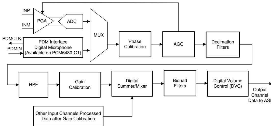
Figure 2. Block Diagram of Audio Signal Chain
