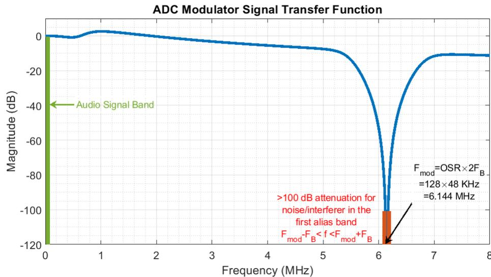
**Figure 3. Signal Transfer Function of ADC Modulator**
