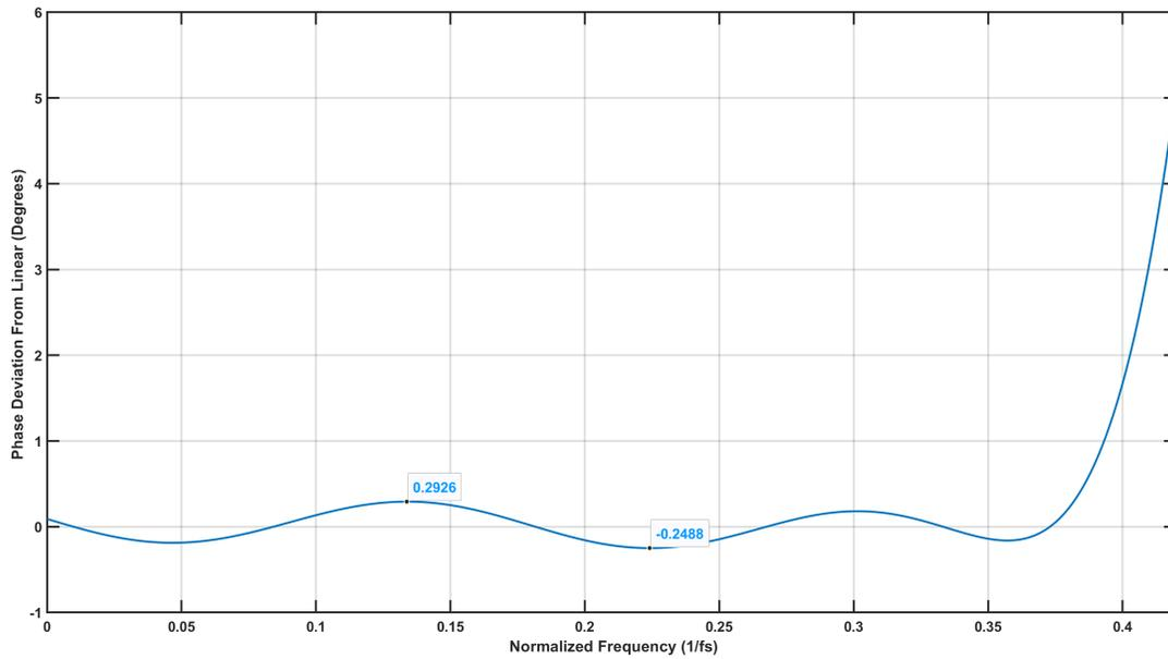
**Figure 7. Phase Deviation of Low-Latency Decimation Filter**
