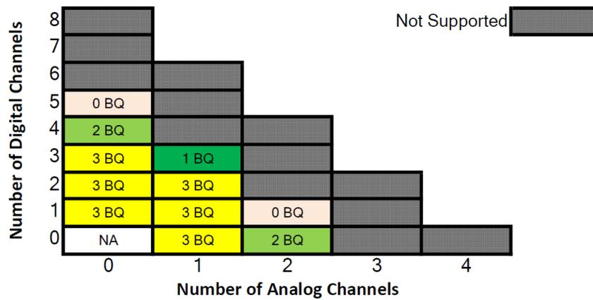
Figure 3-2. Channel Combinations for 96 kHz with DRE/AGC Enabled
