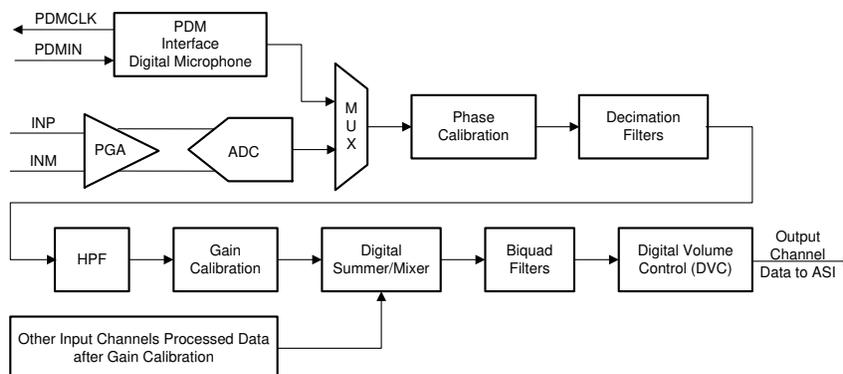
**Figure 1-1. TLV320ADCx140/PCMX140-Q1 Channel Signal Chain Processing Flow Chart**
