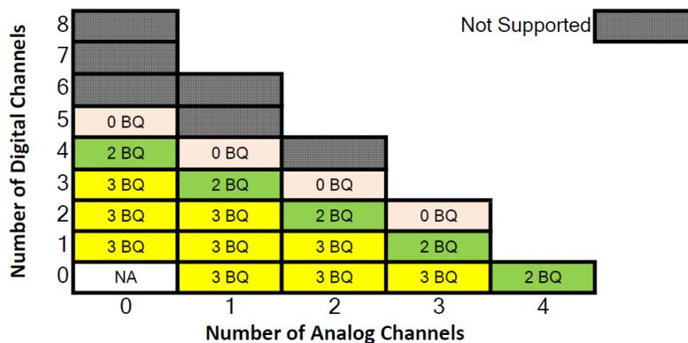
Figure 3-3. Channel Combinations for 96 kHz with DRE/AGC Disabled
