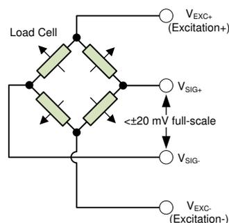
**Figure 2. Typical Load-cell Implementation**
