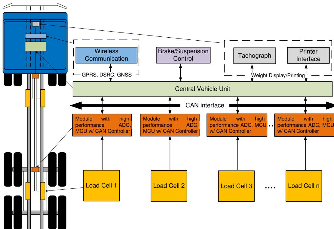
Figure 1. Typical Implementation of an On-Board Weighing (OBW) System
