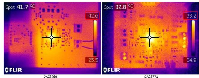
**Figure 3. Thermal Comparison of DAC8760 and DAC8771 with Adaptive Power Management**
