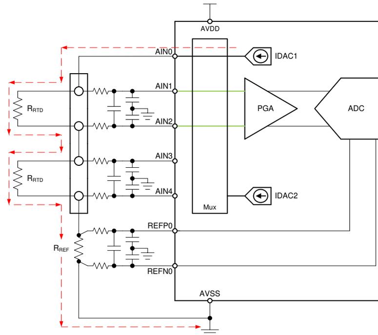
**Figure 2-7. Two Series Two-Wire RTD, Low-Side Reference Measurement Circuit**
