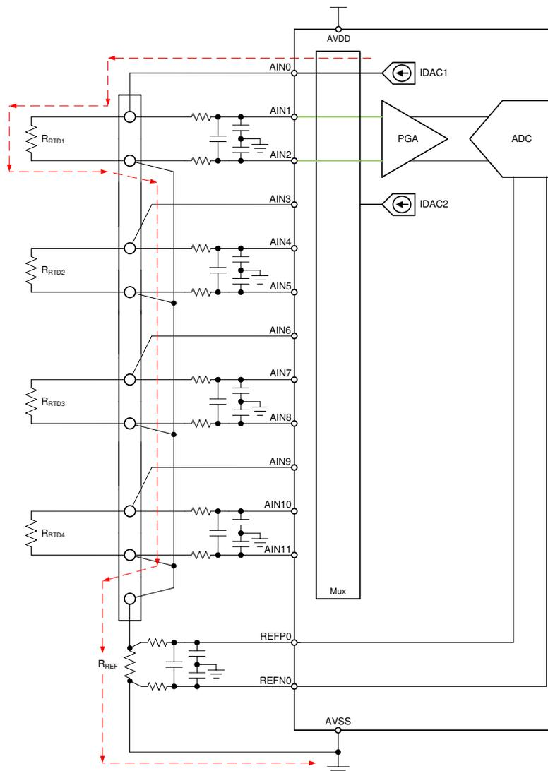
Figure 2-9. Multiple Two-Wire RTDs Measurement Circuit
