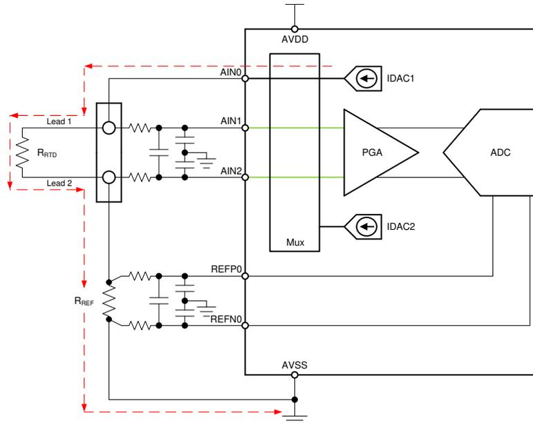
**Figure 2-1. Two-Wire RTD, Low-Side Reference Measurement Circuit**
