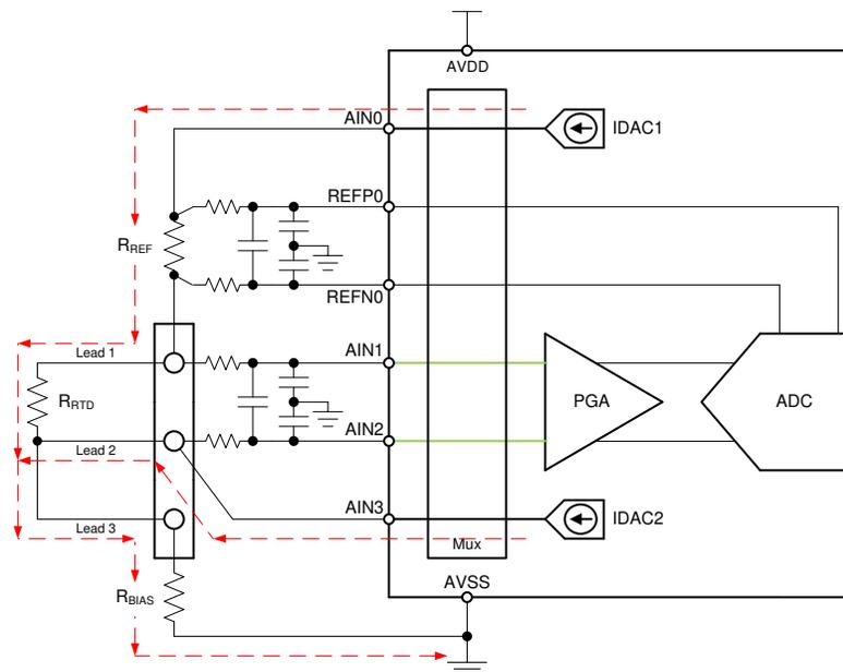
**Figure 2-5. Three-Wire RTD, High-Side Reference Measurement Circuit**
