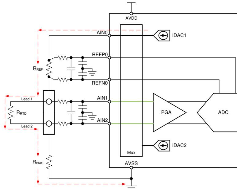
Figure 2-2. Two-Wire RTD, High-Side Reference Measurement Circuit
