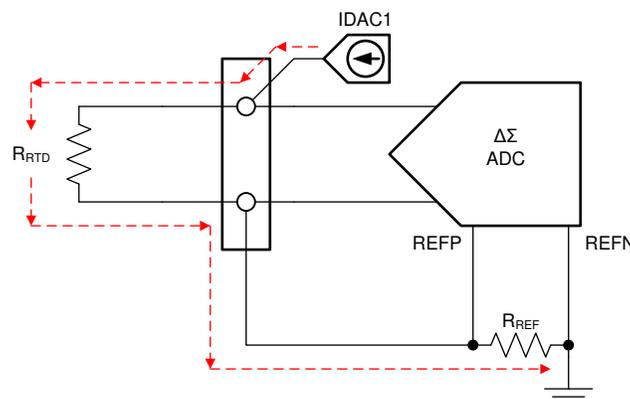
**Figure 1-4. Example of a Ratiometric RTD Measurement**
