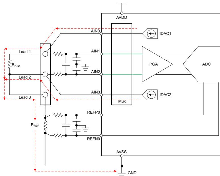
**Figure 2-3. Three-Wire RTD, Low-Side Reference Measurement Circuit**
