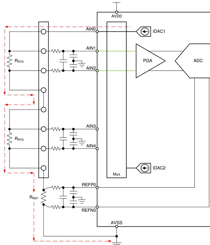
Figure 2-8. Two Series Four-Wire RTD, Low-Side Reference Measurement Circuit
