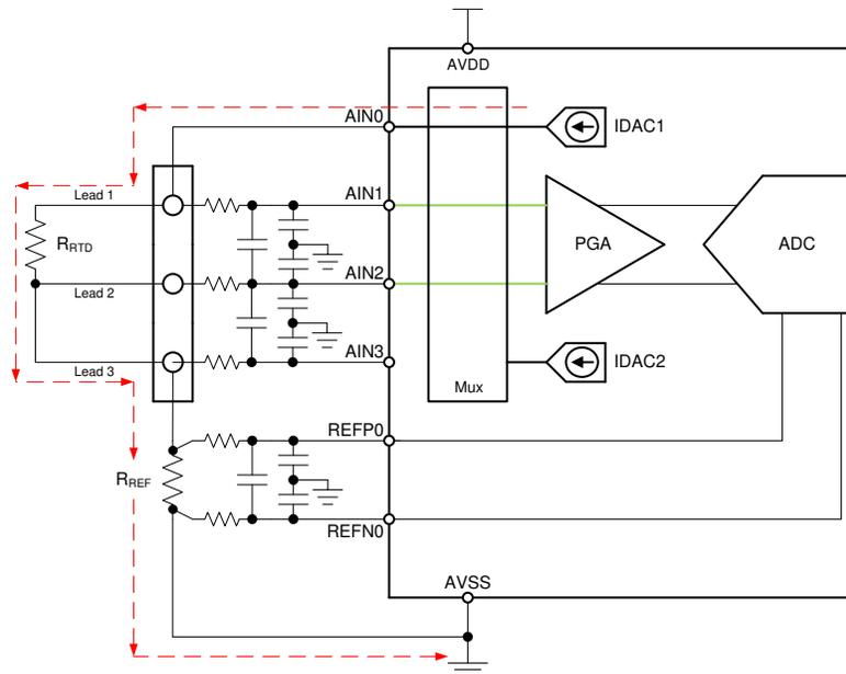
Figure 2-4. Three-Wire RTD, Low-Side Reference Measurement Circuit With One IDAC Current Source
