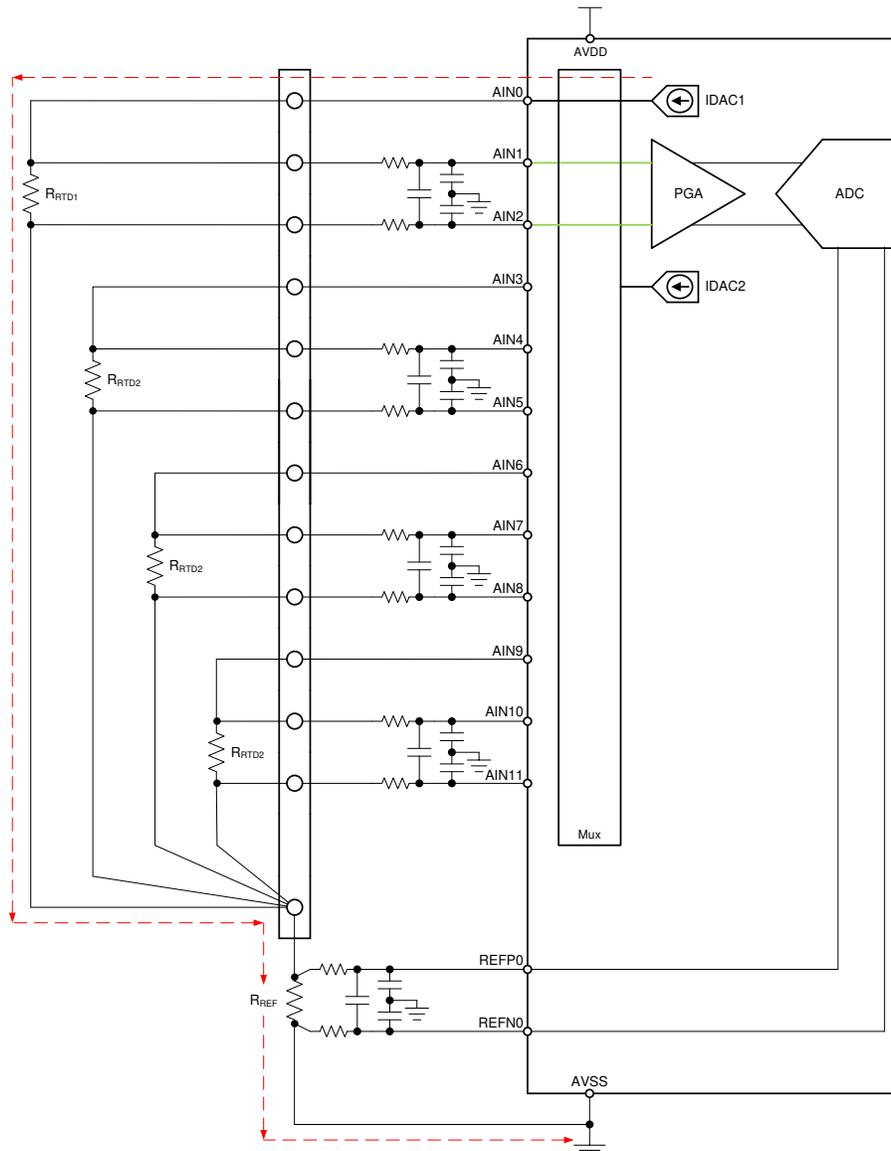
Figure 2-11. Multiple Paralleled Four-Wire RTDs Measurement Circuit
