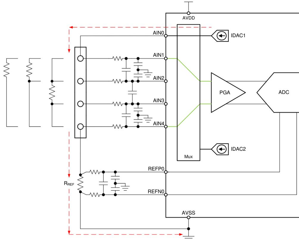
**Figure 2-12. Universal RTD Measurement Interface With Low-Side Reference Circuit**
