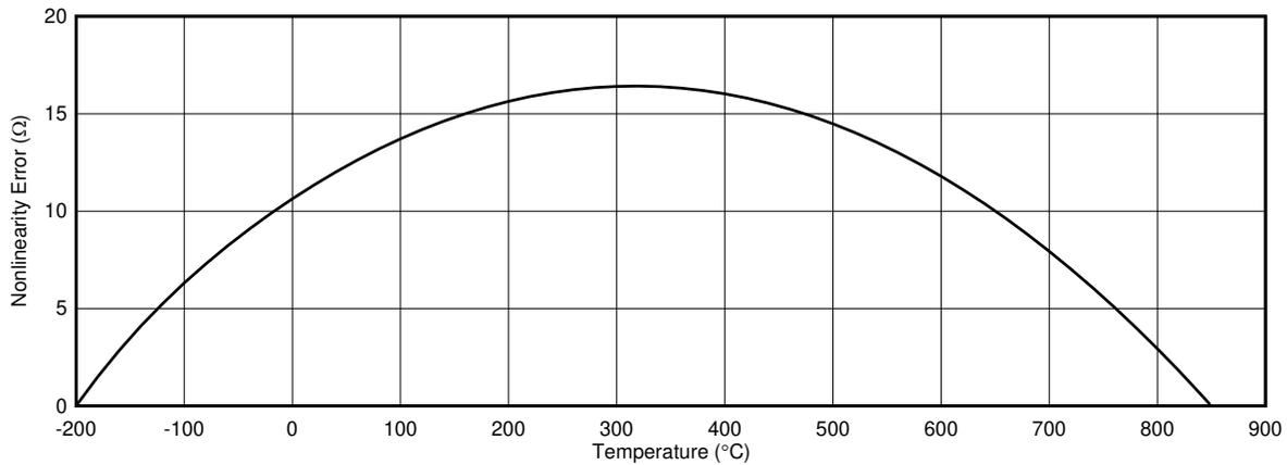
**Figure 1-2. PT100 RTD Non-Linearity From -200°C to 850°C**
