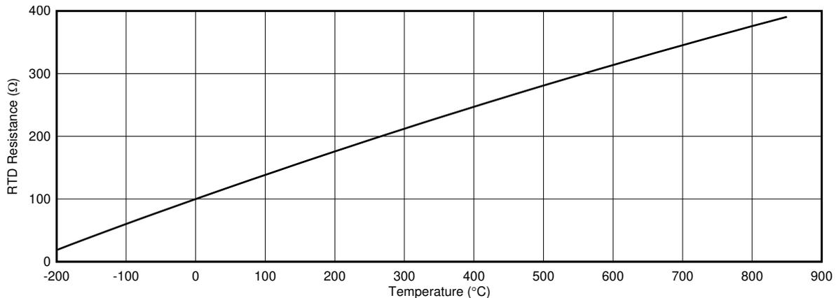
**Figure 1-1. PT100 RTD Resistance From  $-200^{\circ}\text{C}$  to  $850^{\circ}\text{C}$**
