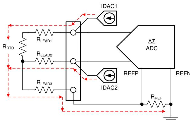
**Figure 1-5. Example of Lead Wire Resistance Cancellation**
