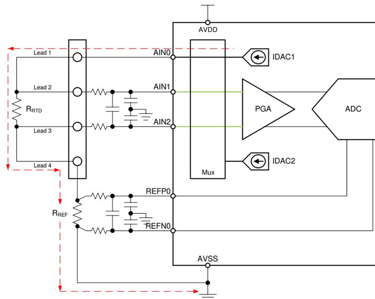
Figure 2-6. Four-Wire RTD, Low-Side Reference Measurement Circuit
