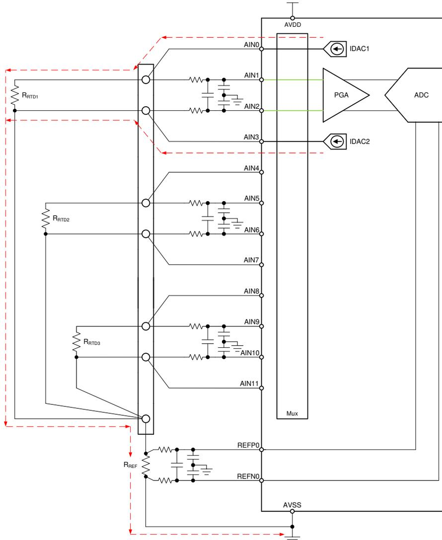
**Figure 2-10. Multiple Three-Wire RTDs Measurement Circuit**
