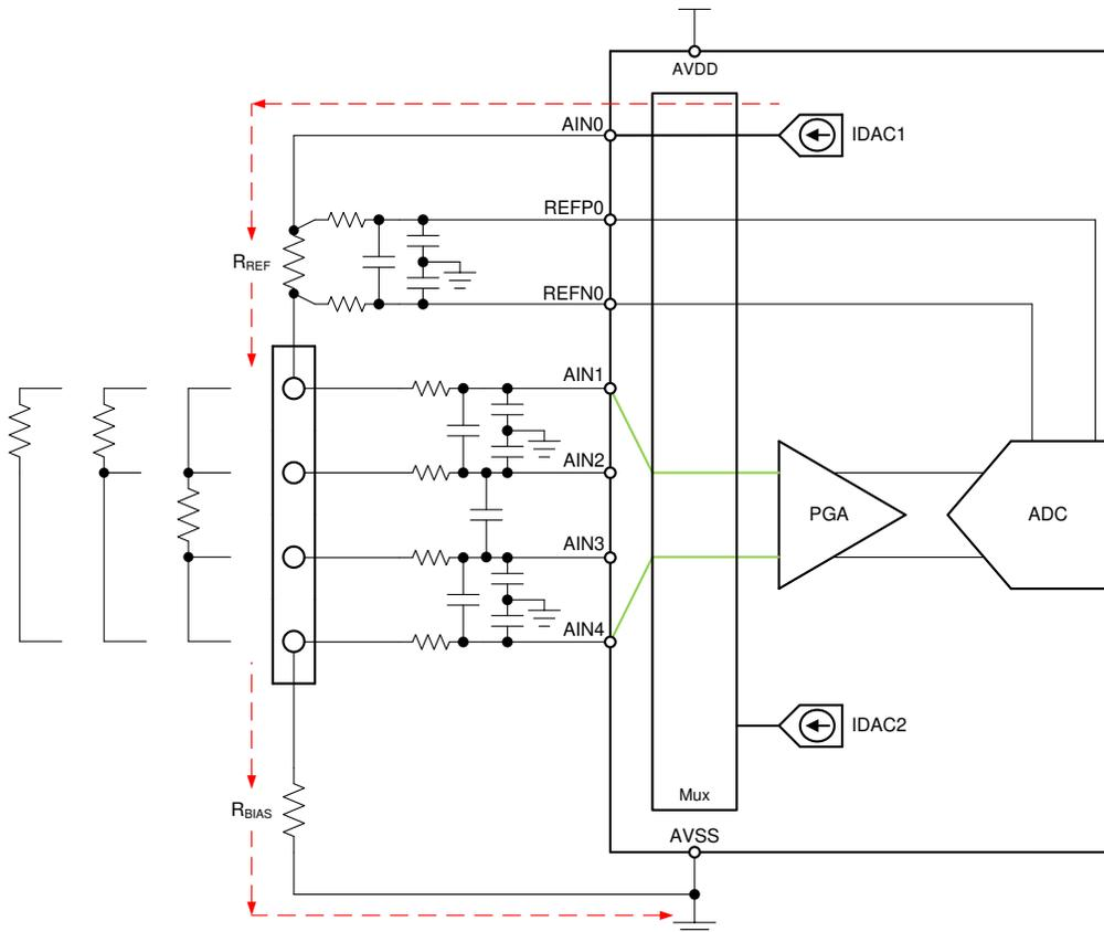
Figure 2-13. Universal RTD Measurement Interface With High-Side Reference Circuit
