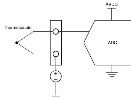
**Figure 1-6. Voltage Biasing of a Thermocouple**
