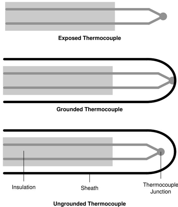
**Figure 1-3. Thermocouple Construction Types**
