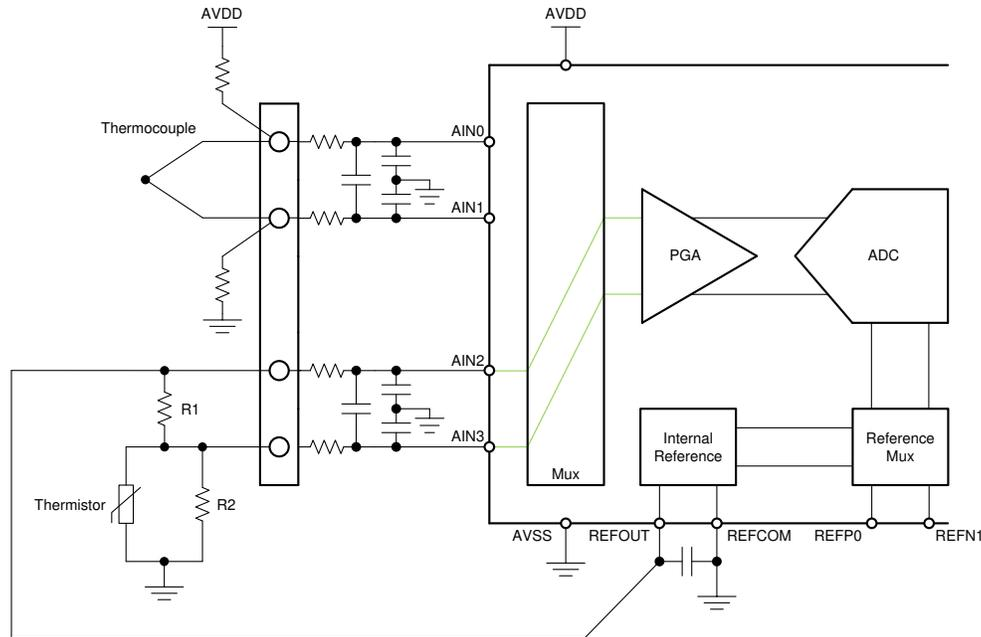
**Figure 2-9. Thermocouple Measurement Circuit With Thermistor Cold-Junction Compensation**
