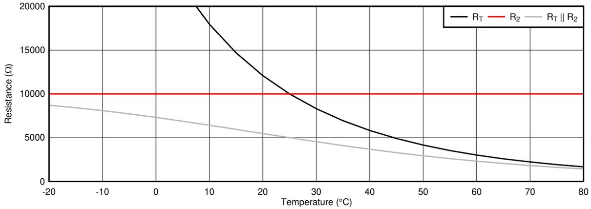
Figure 2-10. Thermistor and Linearization Responses Over Temperature
