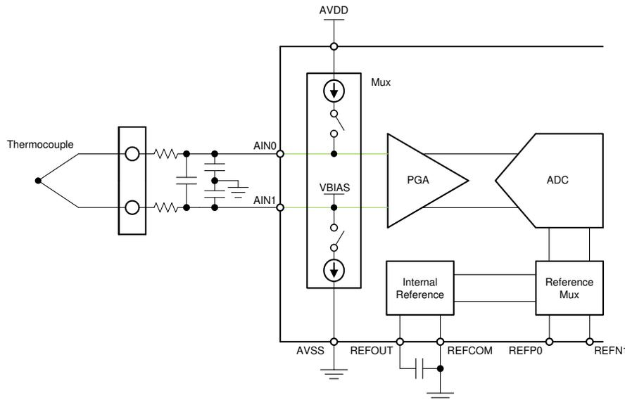
**Figure 2-4. Thermocouple Measurement Circuit With VBIAS for Sensor Biasing and BOCS**
