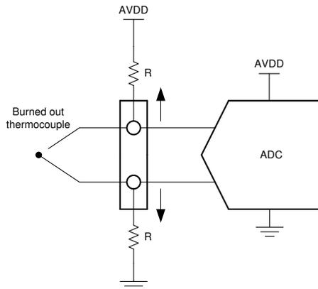
**Figure 1-9. Burn-out Detection Using Resistor Biasing**
