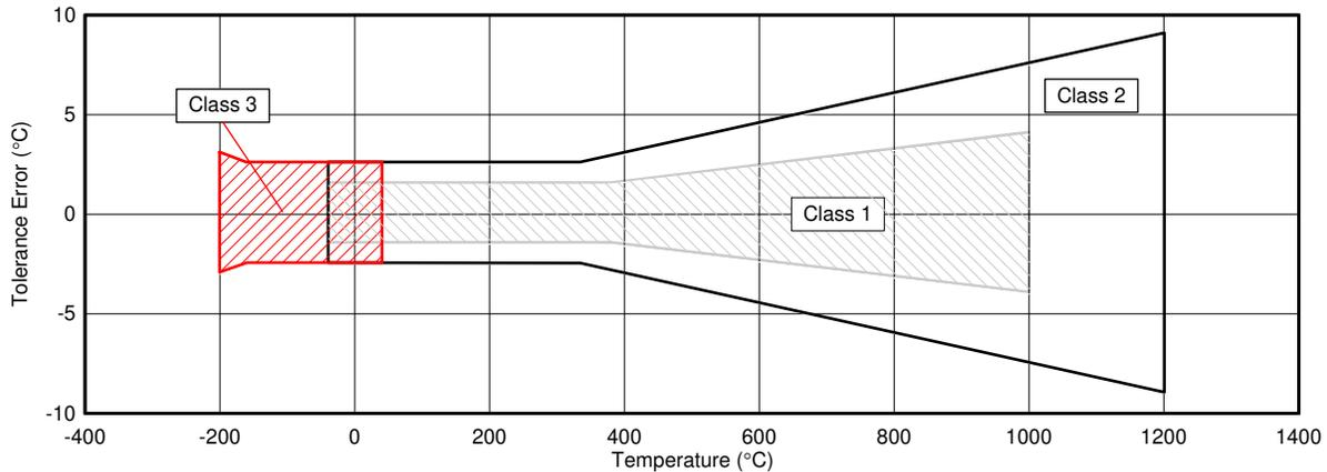
**Figure 1-4. Type-K IEC-EN 60584-2 Tolerance Class Errors**
