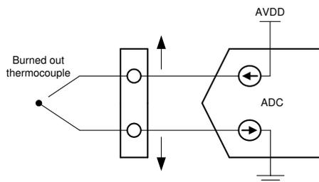
**Figure 1-10. Burn-out Detection Using BOCS**
