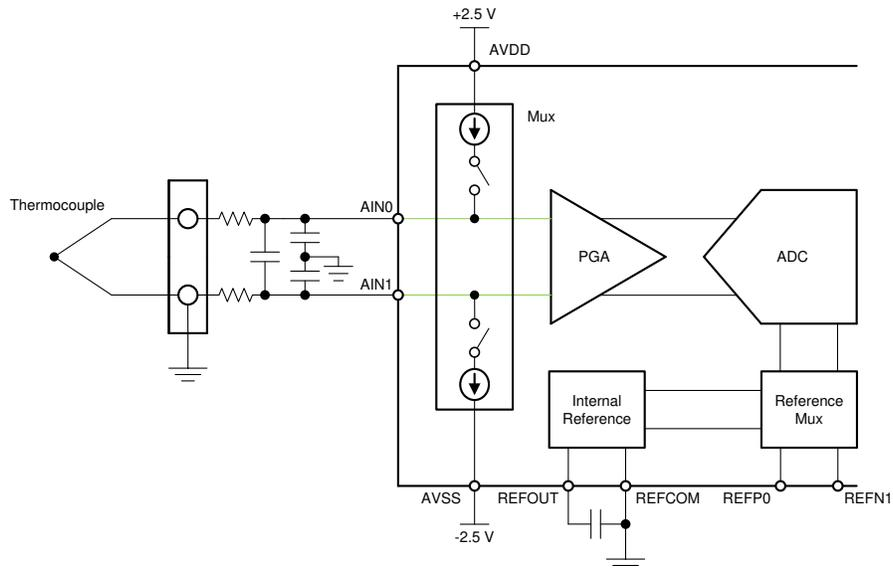
**Figure 2-7. Thermocouple Measurement Circuit With Bipolar Supplies and Ground Biasing**
