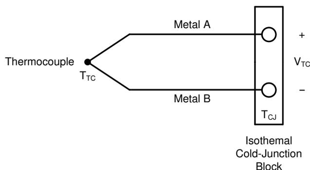
**Figure 1-1. Thermocouple Voltage**
