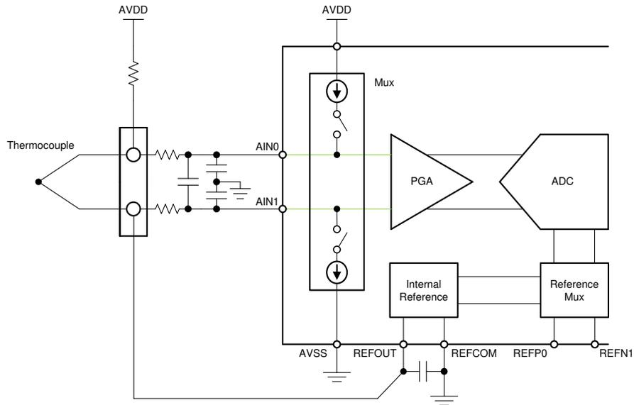
**Figure 2-5. Thermocouple Measurement Circuit With REFOUT Biasing and Pullup Resistor**
