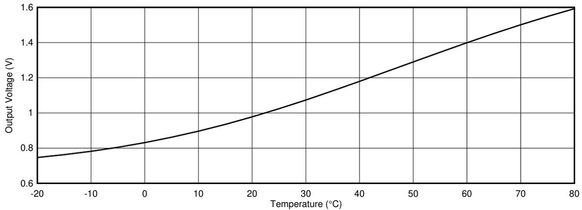
**Figure 2-12. Linearized Output of Thermistor Circuit**
