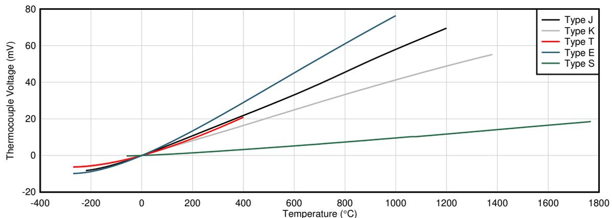
**Figure 1-2. Thermocouple Responses**
