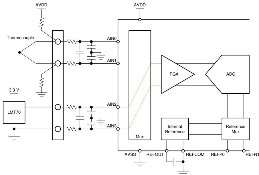
Figure 2-13. Thermocouple Measurement Circuit With Temperature Sensor Cold-Junction Compensation
