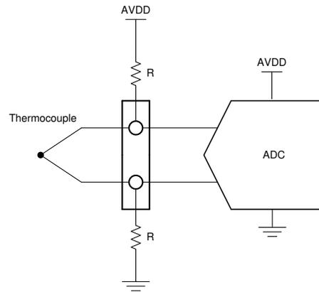
**Figure 1-5. Resistor Biasing of a Thermocouple**
