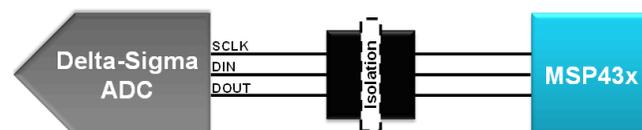
Figure 3. Isolation Scheme Using 3-wire SPI
