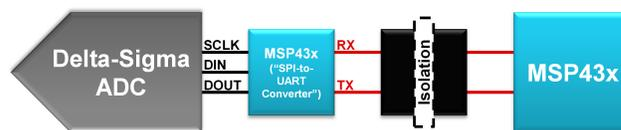
Figure 4. Isolation Scheme Using “SPI-to-UART Converter”
