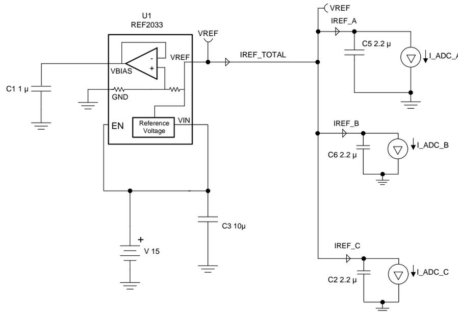
Figure 14. TINA-TI™ Schematic for Voltage Reference Settling
