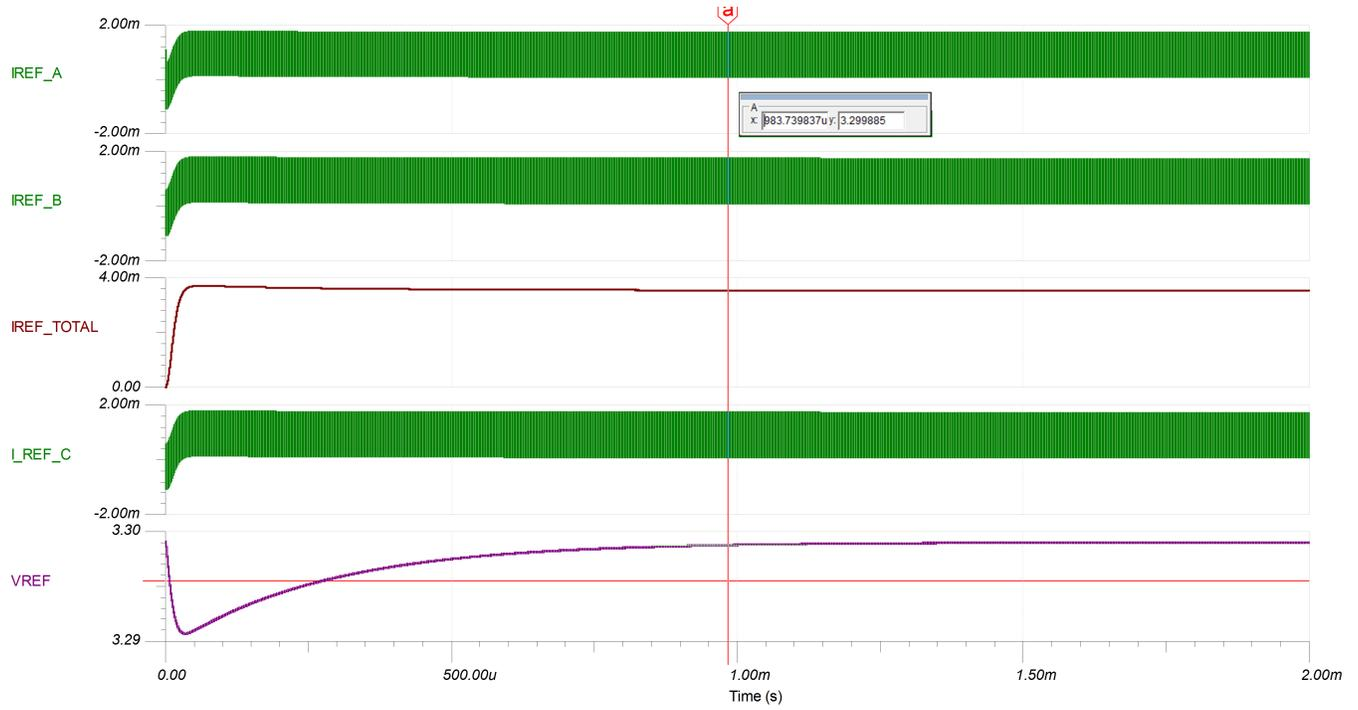
Figure 15. TINA-TI™ Simulation Results for Voltage Reference Settling
