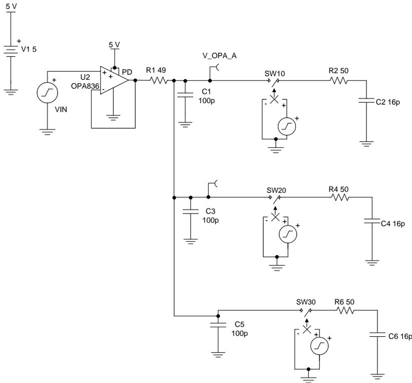
Figure 12. TINA-TI™ Schematic for Noise Analysis of Front End Driver
