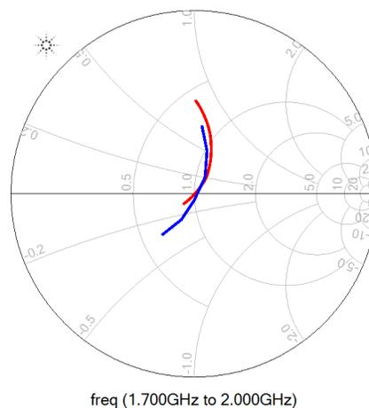
**Figure 19. Comparison Between Lab and Simulation for S11**
