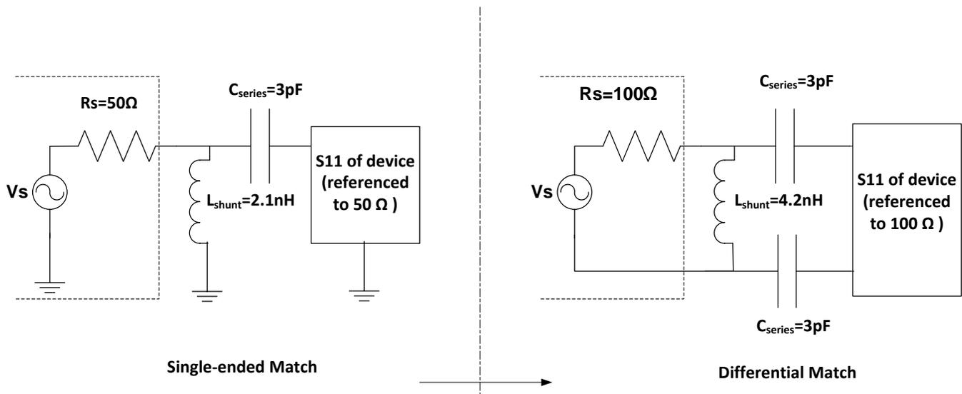
Figure 14. Single-Ended and Equivalent Differential Matching Network
