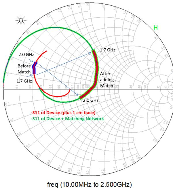
**Figure 17. S-Parameters Before and After Adding Matching Network**
