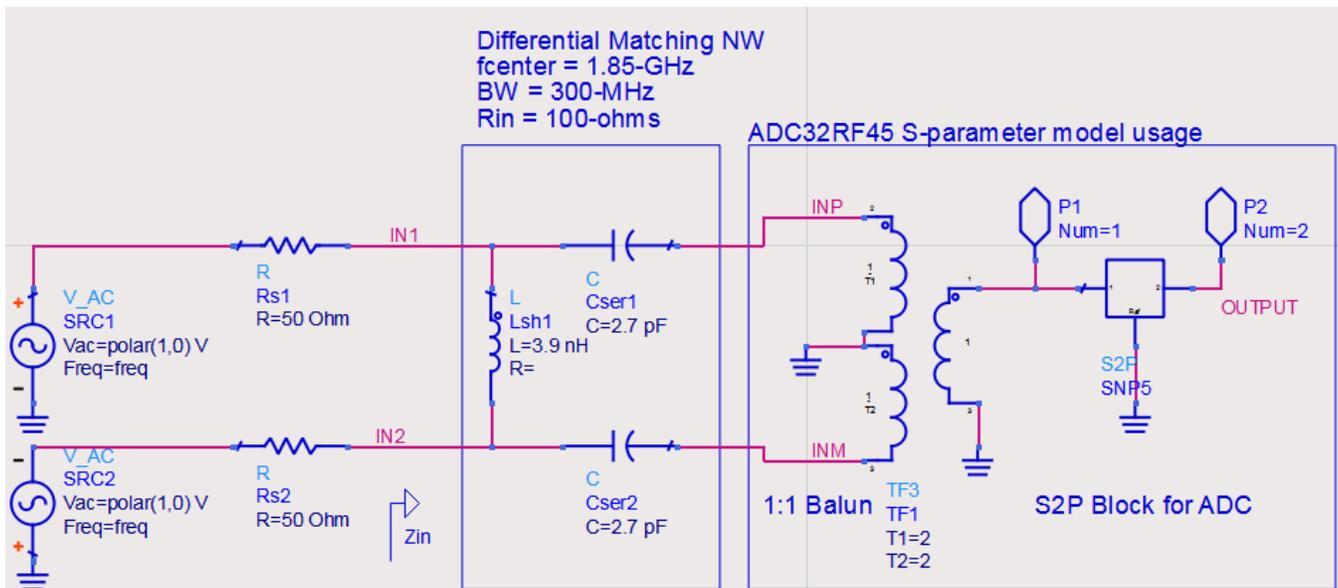
**Figure 16. Simulation Deck for Matching Network Analysis**
