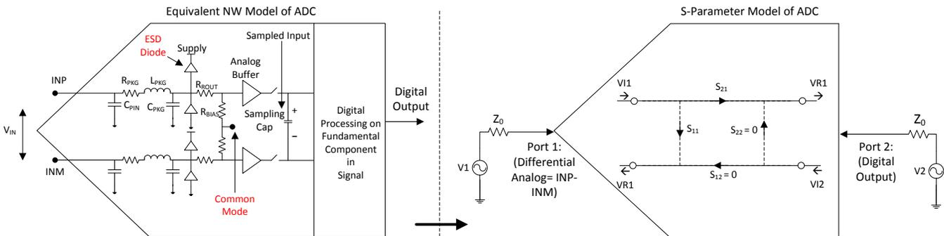
Figure 7. Equivalent NW Model and S-Parameter Model for ADC With S12 and S22 Chosen as 0
