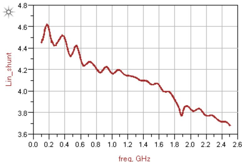
The frequency profile was obtained through an S-parameter characterization of the component in the lab.
