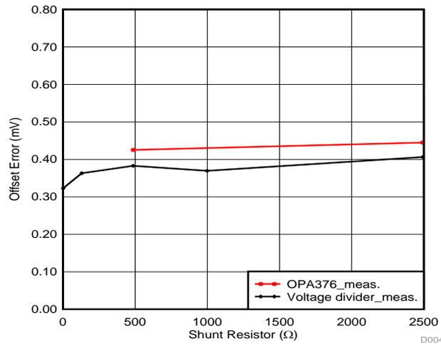
Figure 7. Offset Error vs Different Shunt Resistor With OPA376 (AMC1204)
