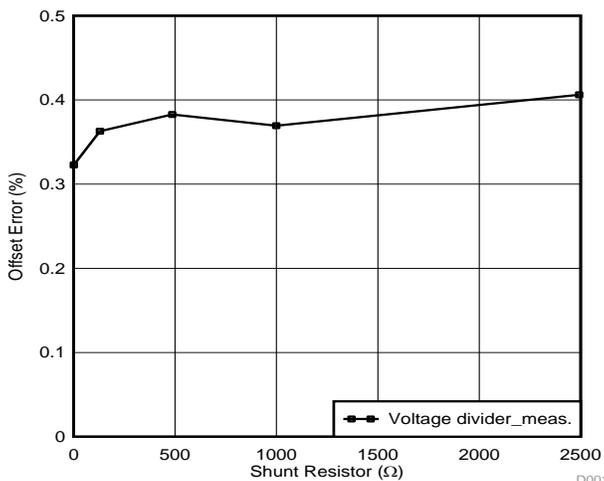
Figure 3. Offset Error vs Different Shunt Resistor (AMC1204)
