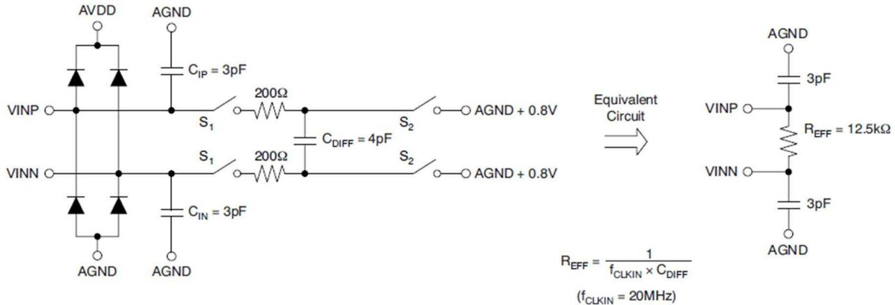
Figure 1. Equivalent Analog Input Circuit
