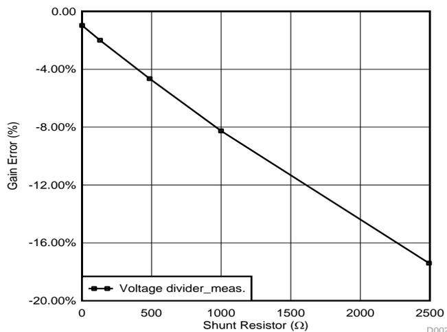
Figure 4. Gain Error vs Different Shunt Resistor (AMC1204)
