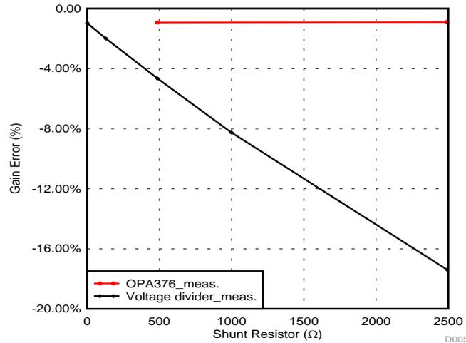
Figure 8. Gain Error vs Different Shunt Resistor With OPA376 (AMC1204)
