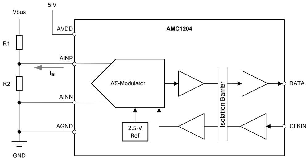
Figure 2. First Rough Solution to Perform Isolated Voltage Monitoring
