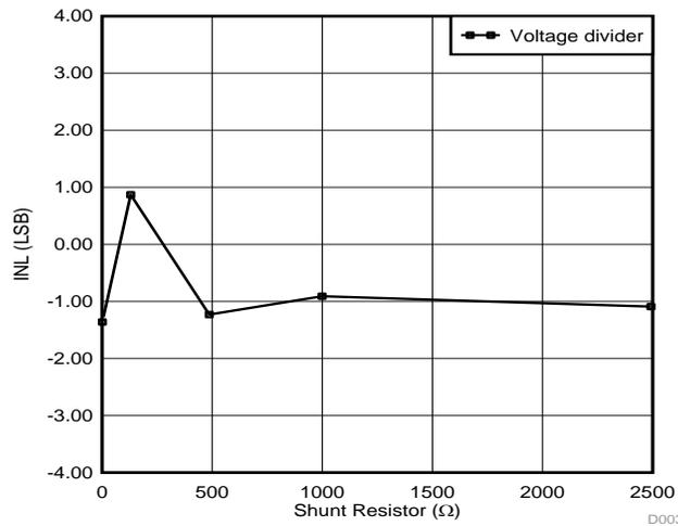
**Figure 5. INL vs Different Shunt Resistor (AMC1305M25)**
