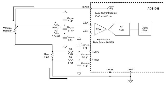
Figure 3-3. Example of a Four-Wire Ratiometric Configuration with RC Filters (R <sub>Lead</sub> Removed for Simplicity)
