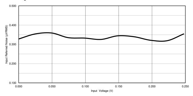
Figure 3-4. Input-Referred Noise vs Input Voltage Using Matched RC Filters
