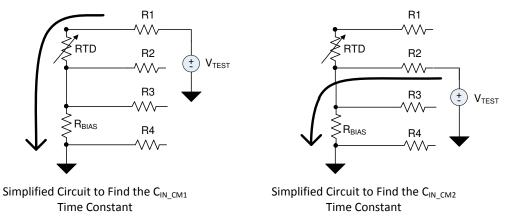
Figure 2-4. Simplified RC Circuit to Find the Corner Frequency of the Common-Mode Input Filter
