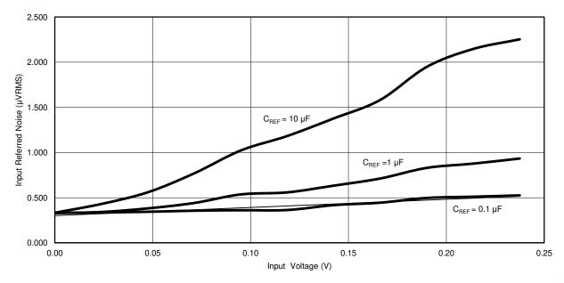
Figure 3-2. Input Referred Noise vs Input Voltage Using Mismatched RC Filters
