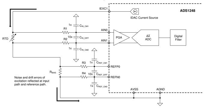
Figure 2-2. Four-Wire Ratiometric RTD Measurement with Filters (R<sub>LEAD</sub> Removed for Simplicity)
