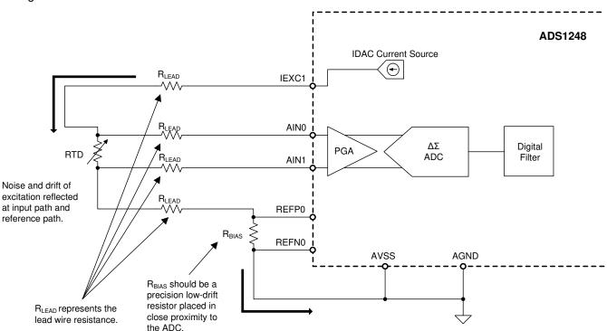
Figure 1-1. Four-Wire Ratiometric RTD Measurement Using the ADS1248
