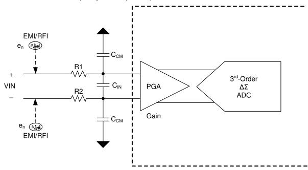
Figure 2-1. Typical Differential and Common-Mode Filter
