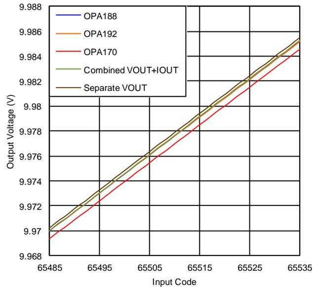
Figure 15.  $\pm 10$ -V Output Results with Bipolar Supplies
