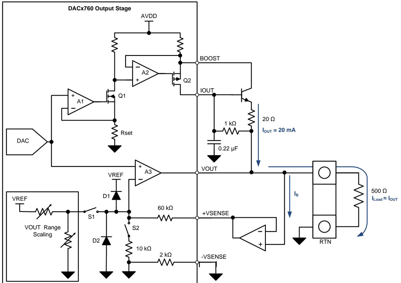
Figure 16. Buffering the +V<sub>SENSE</sub> Pin Using an External Amplifier with a Boost Transistor
