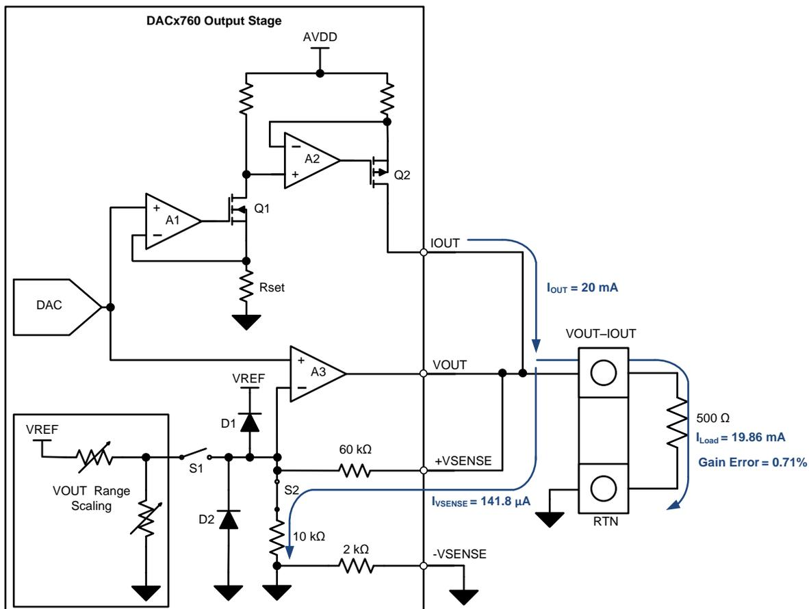
Figure 5. Closing S2 in Current Mode with a Combined V<sub>OUT</sub>-I<sub>OUT</sub> Connection
