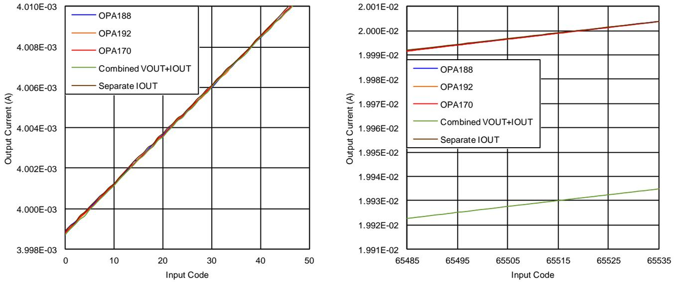
Figure 11. 4-mA to 20-mA Output Results with Unipolar Supplies
