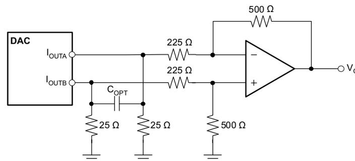
**Figure 2. DC-Coupled, Differential to Single-Ended DAC Interface**
