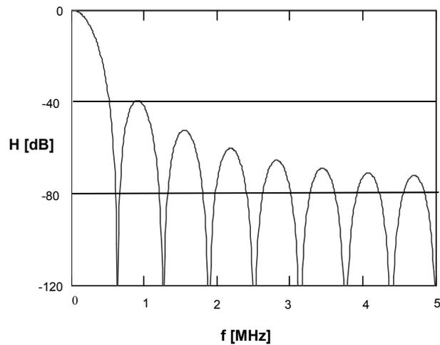
**Figure 10. Frequency Response of the Sinc<sup>3</sup> Filter with M = 16**
