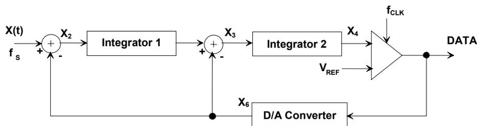
**Figure 4. Block Diagram of the 2nd-Order Modulator**
