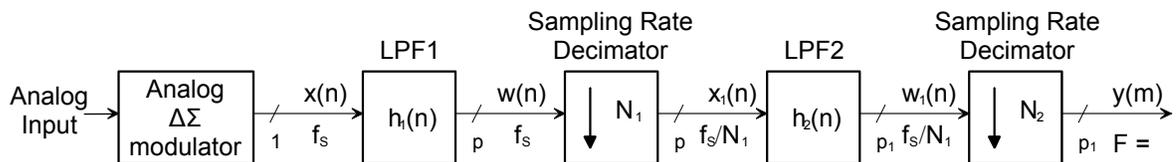
**Figure 7. Simple Example of a Two-Stage Network for Decimation by a Factor of  $N_1N_2$**
