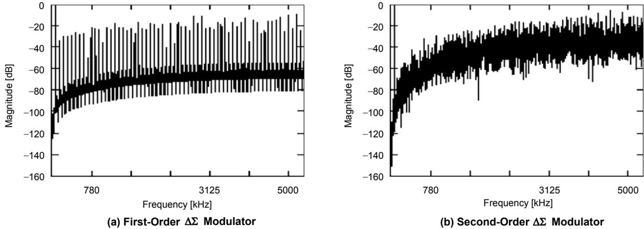
**Figure 5. 1st and 2nd Order ΔΣ Modulator Modulation Noise**
