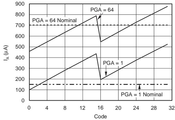
Figure 7. Analog Current Consumption vs Code at 18MHz
