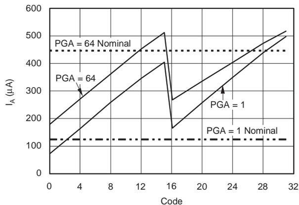
**Figure 5. Analog Current Consumption vs Code at 4.9152MHz**
