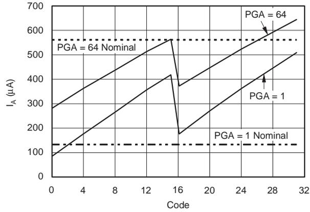
Figure 6. Analog Current Consumption vs Code at 10MHz
