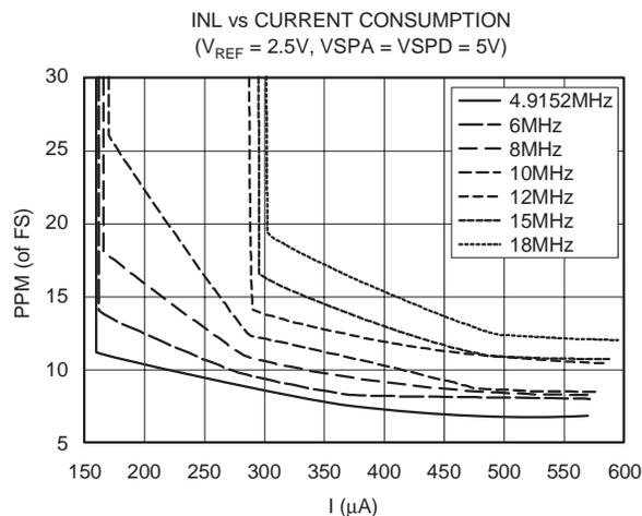
**Figure 2. Typical Integral Nonlinearity versus Current Consumption at Various Standard Clock Frequencies**
