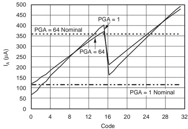
**Figure 4. Analog Current Consumption vs Code at 2.4576MHz**
