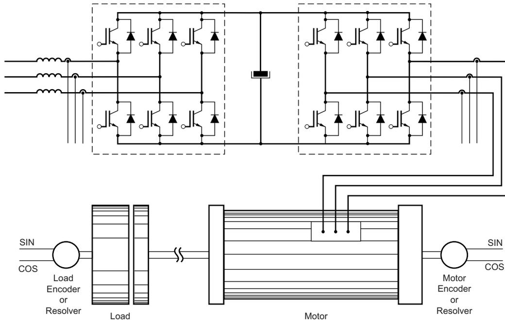
Figure 1. Motor Control System with Measuring Signals
