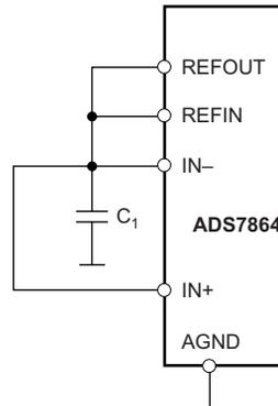
**Figure 8. A/D Converter DC Parameter Testing Circuit**
