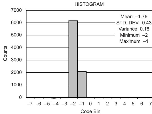
Figure 9. Histogram of 8192 Points with Inputs Connected Together
