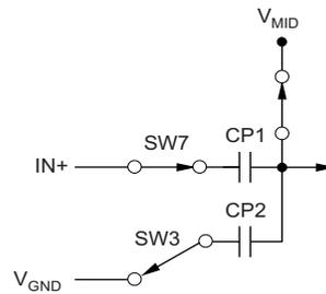
**Figure 5. Equivalent Input Circuit During Sampling, Acquisition, Time**
