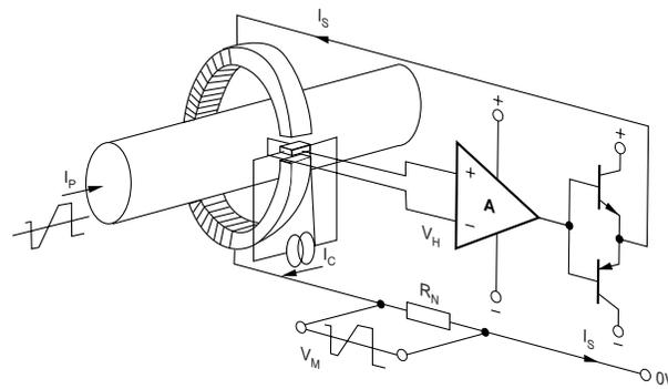
**Figure 2. Operating Principle of the Closed-Loop Transducer**
