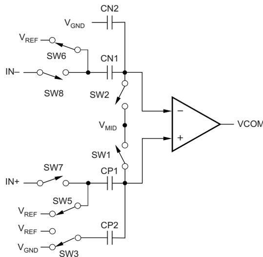
Figure 4. Equivalent Input Circuit of SAR A/D Converter
