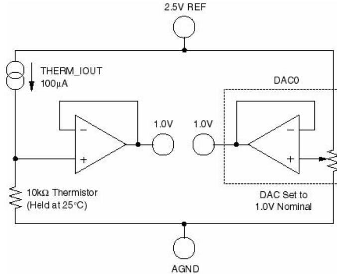
By using the reference in this ratiometric mode, the absolute value of the reference doesn't matter; moreover, reference drifts over time and temperature won't affect the temperature control loop at all.
