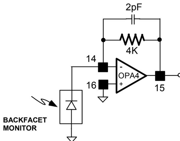
The ADC monitors the output signal from this circuit, in hopes that the back facet monitor diode's measurement of optical power is approximately correct. This is probably true as long as the output power is close to the rated power (remember the tracking ratio is better at higher powers!) and the monitor diode is kept at a constant temperature—and that has been taken care of already by the TEC.
