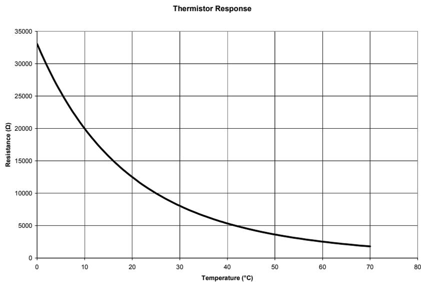
Since the thermistor is the transducer for measuring temperature, and the system must measure and control temperature within  $0.01^\circ\text{C}$ , this transducer must be linearized. Fortunately, the characteristic of this thermistor is known, so the nonlinearity can be taken into account.
