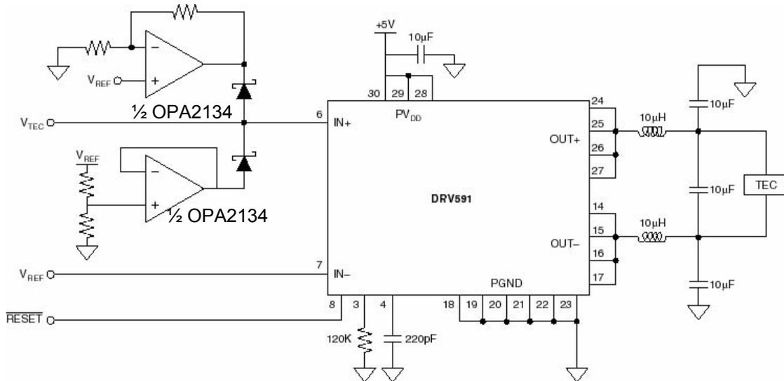
The PWM driver circuit shown in Figure 8, built around a Texas Instruments DRV591, can supply up to  $\pm 3A$  to a TEC. The DRV591 has a fixed gain of 2.34, resulting in a transfer function of:
