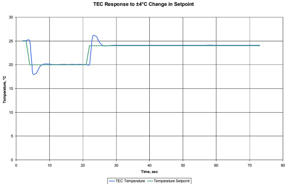
The resulting operation of the TEC control loop is shown in Figure 11. Temperature stability, even under a 20°C change in ambient temperature, was approximately  $\pm 0.005^{\circ}\text{C}$  at steady state. Note that for the most part, the temperature stability is within  $\pm 0.002^{\circ}\text{C}$  over a long period, and is within  $\pm 0.001^{\circ}\text{C}$  for short periods.
