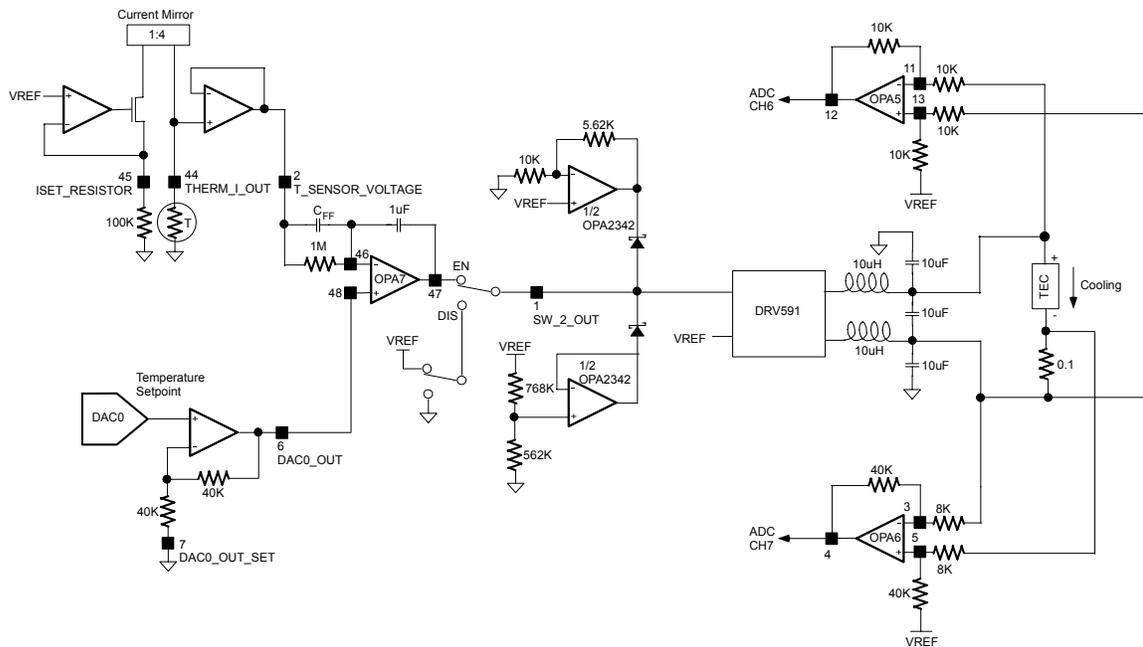
DAC0 determines the temperature setpoint, and affords temperature resolution of approximately 0.03°C per LSB. The DAC requires a reference voltage; the internal AMC7820 reference will have an initial tolerance of 2%, and a drift of 10ppm/°C. How can this error be eliminated?
