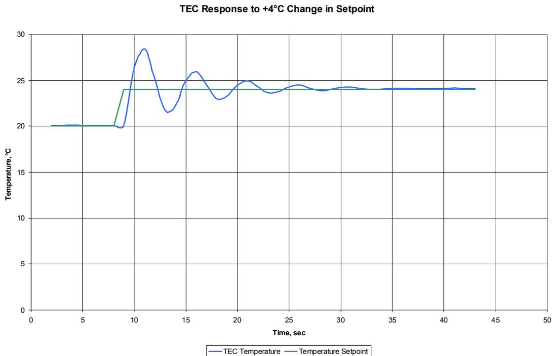
Adding a feedforward capacitor ( $C_{FF}$ ) to the integrator greatly reduces the overshoot and the time needed for the loop to stabilize. See Figure 10 for a 1 $\mu$ F capacitor used as the feedforward capacitor; the system is still a bit underdamped. Note that the response time has reduced to about 5 seconds.
