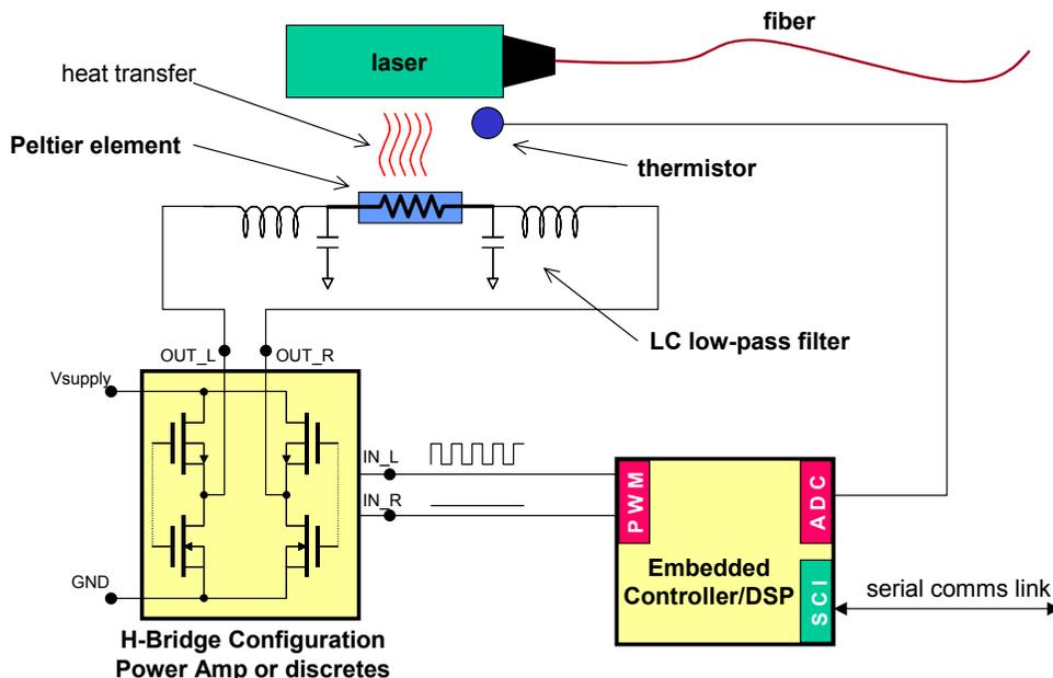
For system stability, note that maintaining  $\pm 0.1^\circ\text{C}$  temperature stability with the newer laser still may result in a change of 0.002nm out of the 975nm center wavelength. This is a change of  $\pm 2\text{ppm}$ . Even with the great advances made in the lasers over the past year, temperature control is still a very important part of the optical system, as overall stability of approximately  $\pm 4\text{ppm}$  is needed in these systems.
