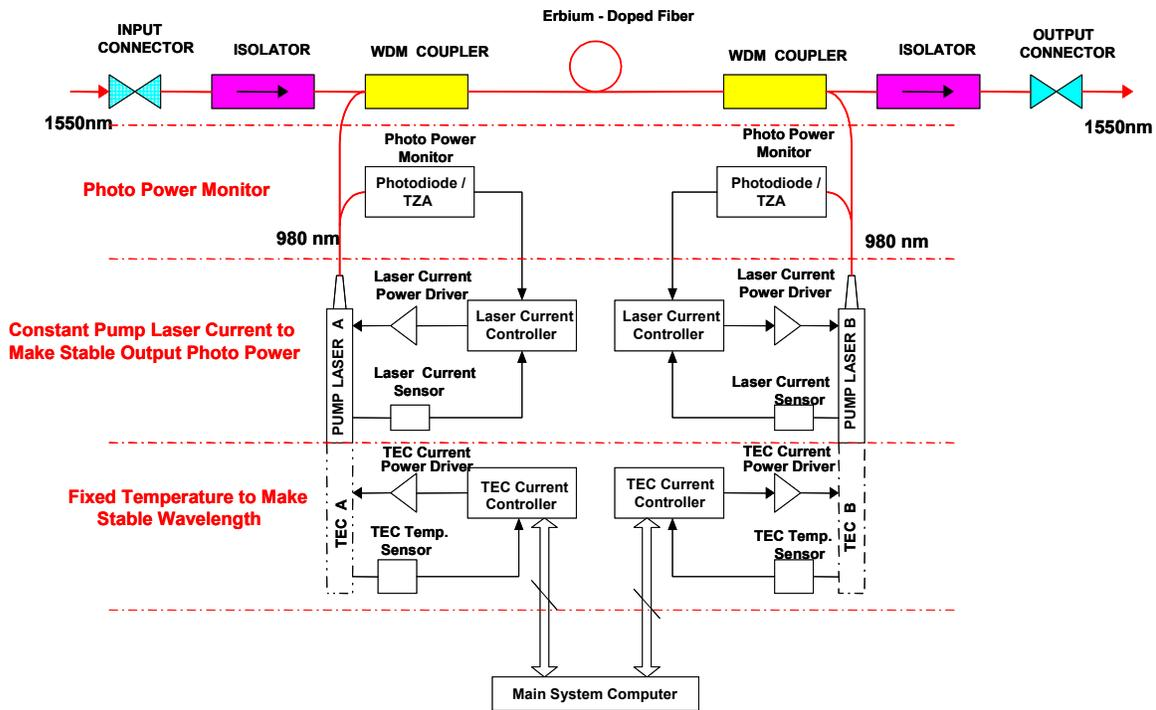
There are actually several control loops here. Inside the laser module, there are control loops for the pump laser current and the TEC, to laser current optical power and temperature. These loops are relatively slow, almost DC control problems.
