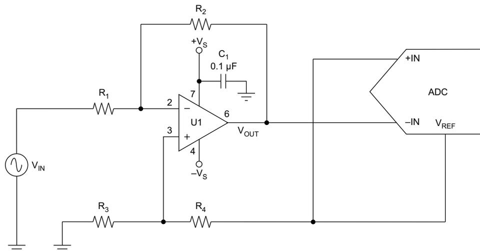
**Figure 5. Circuit Schematic Utilizing the Programmable Gain Amplifier and Output Voltage Reference.**
