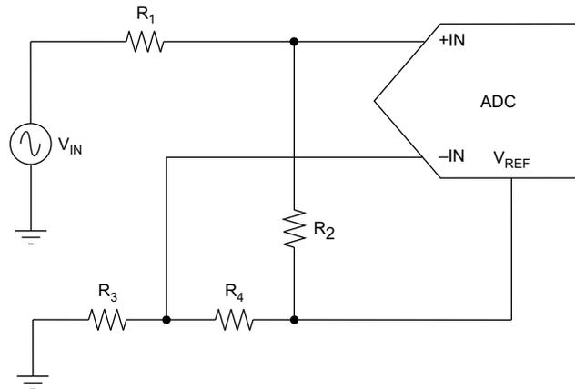
**Figure 3. Utilizing a Resistive Network to Achieve Attenuation and DC Bias of the Input Signal.**
