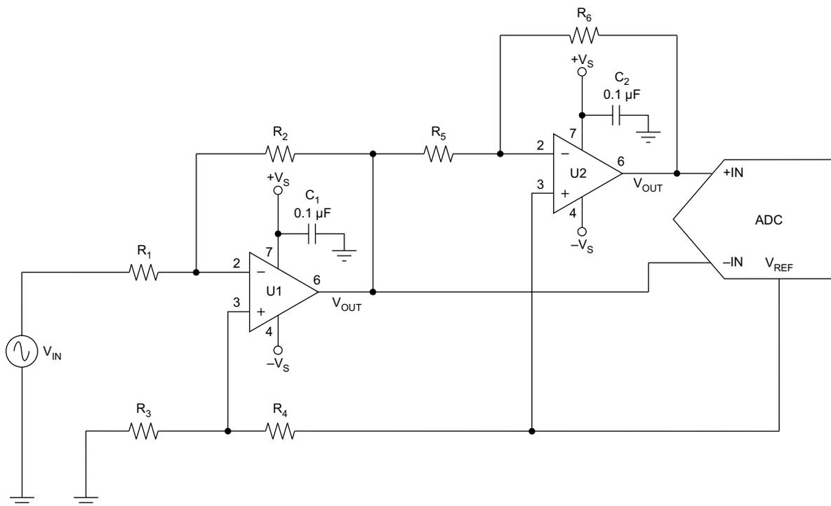
**Figure 1. Circuit Schematic to Convert a Single-Ended Bipolar Input to a Unipolar Differential Output.**
