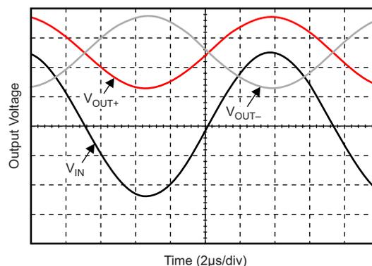
**Figure 2. Scope Trace (Circuit of [Figure 1](#)),  $V_{IN} = 5Vp-p$  (Bipolar), with a Corresponding Differential Output, ( $V_{OUT+}$ ,  $V_{OUT-}$ ) = 2.5Vp-p Biased at 2.5V DC.**
