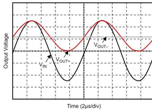
**Figure 4. Scope Trace, V<sub>IN</sub> = 5Vp-p V<sub>IN</sub> = 5Vp-p (Bipolar), with a Corresponding Output, V<sub>OUT+</sub> = 2.5Vp-p Biased at 2.5V DC, V<sub>OUT-</sub> = 2.5V DC.**
