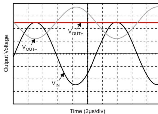
**Figure 6. Scope Trace,  $V_{IN} = 5\text{Vp-p}$   $V_{IN}$  (bipolar), with a Corresponding Output,  $V_{OUT+} = 2.5\text{V DC}$   $V_{OUT-} = 2.5\text{Vp-p}$  Biased at  $2.5\text{V DC}$**
