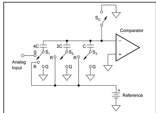
FIGURE 2. Simplified 3-bit Switched Capacitor Array A/D.
