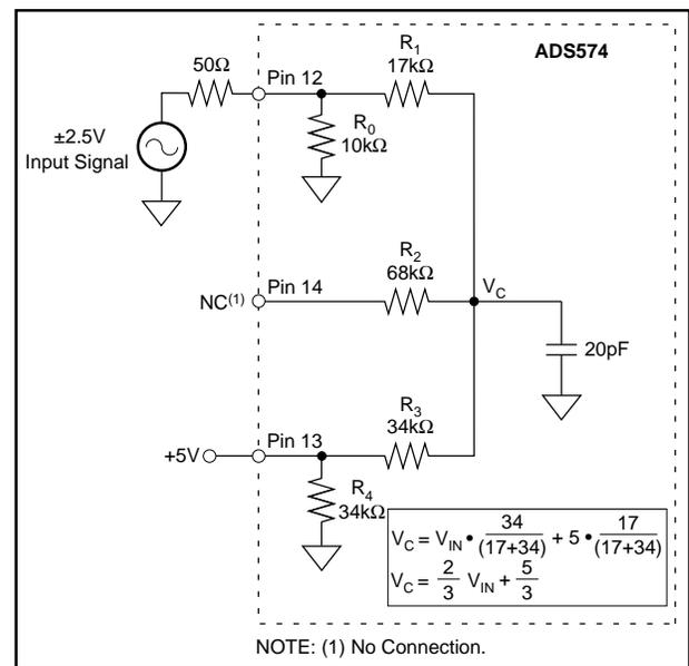
FIGURE 6. Connections for  $\pm 2.5$ V Input Range.
