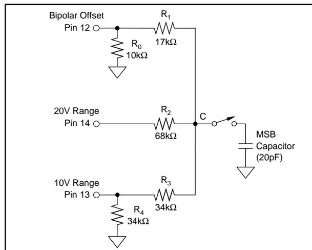
FIGURE 3. ADS574 Input Structure.
