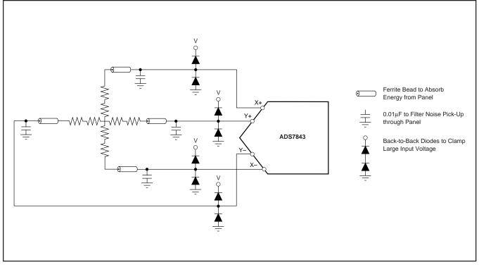
FIGURE 9. Input Protection for ADS7843.
