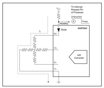
FIGURE 6. Simplified Schematic of ADS7843 for PD0, PD1 = 00.
